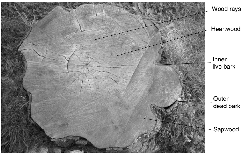
FIGURE 2.4 Cross-section of a tree trunk showing outer dead bark, inner live bark, sapwood, heartwood, and wood rays. (Source: Photograph by author.)
