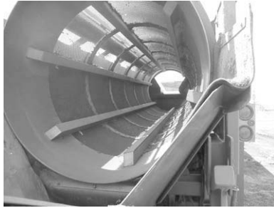
FIGURE 8.13 Portable trammel used in the fuel yard for size classification. (Source: Photograph by the author).
