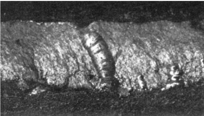
Figure 3.25 Wormhole porosity in weld metal. From Jackson (55).
