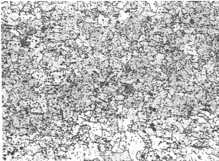
Figure 5 Typical microstructure of the weld metal ( \times 320 )
