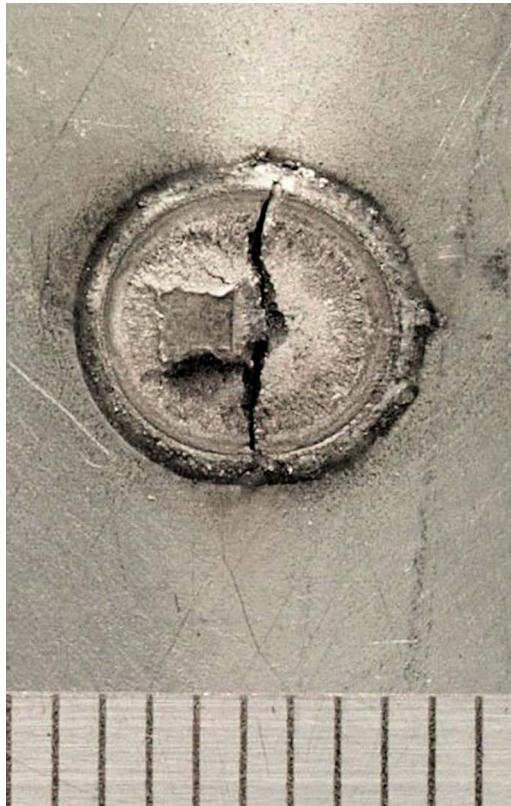
FIGURE 1.2 Interfacial weld defect showing a prominent crack from the RSW process [5].
