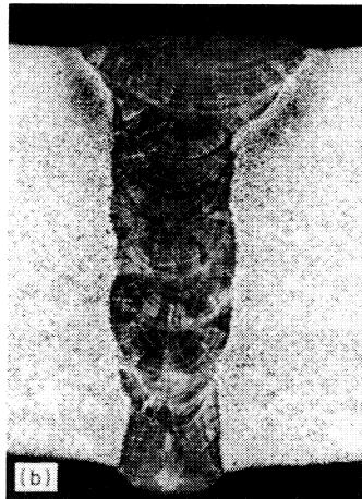
42 Narrow gap weld in 15mm (0.6in) wall thickness cast HK40 pipe using TIG-cold wire: a) Joint preparation; b) Section through weld (courtesy of APV Paramount Ltd).
