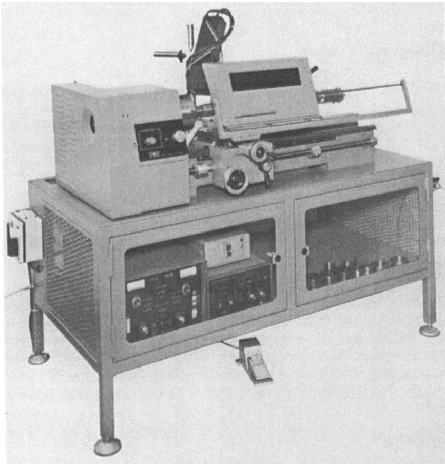
7.1 Manually loaded automatic TIG welding lathe with single button sequence control.
