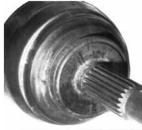
Figure 9.1. View of driveshaft and CV housing (front wheel) with its arc weld
