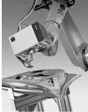
Figure 2.15. Six axis robot equipped with a remote laser welding system (Trumpf document)
