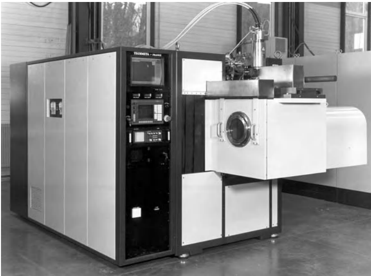
Figure 2.19. 6 kW EBW machine; dimensions 0.6 m × 0.6 m × 0.9 m (Techméta document)
