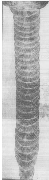
Figure 11.10. Macrographic section of a narrow chamfer TIG weld carried out in the 5GT position
