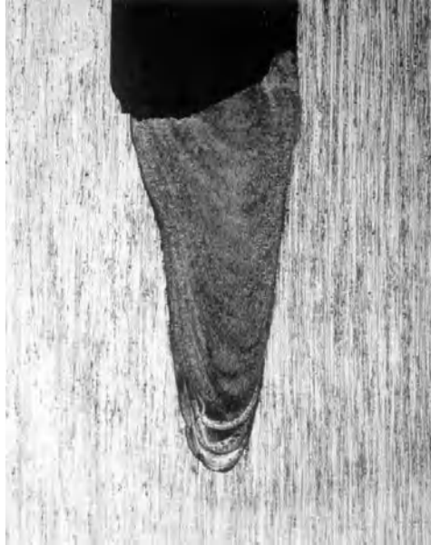
Figure 2.31. 2 mm penetration depth in a aluminum alloy 7020 welded by electron beam (Institut de Soudure document)
