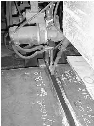
Figure 10.10. Butt weld joint – photograph from Baudin-Châteauneuf
