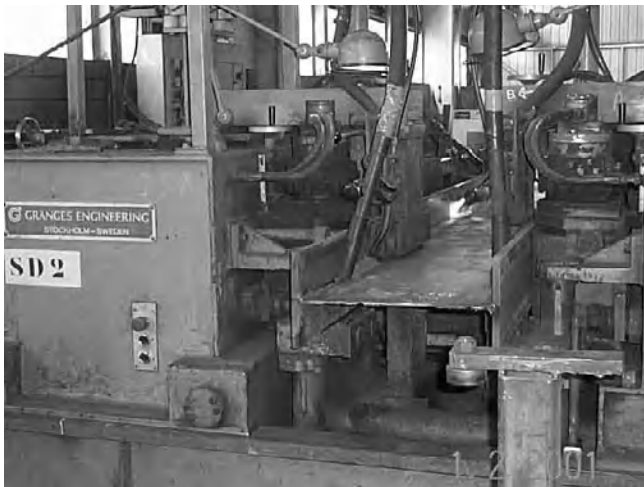
Figure 10.3. Construction of an I section on a horizontal bench – photograph from Baudin-Châteauneuf
