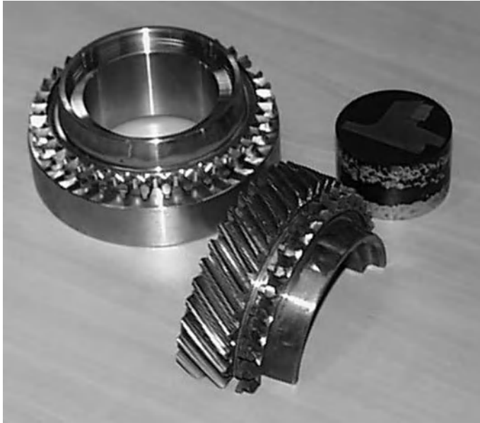
Figure 9.3. Picture of a dog clutch welded onto a pinion with teeth cut or not
