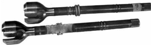
Figure 9.10. Shaft friction welded to tulip
