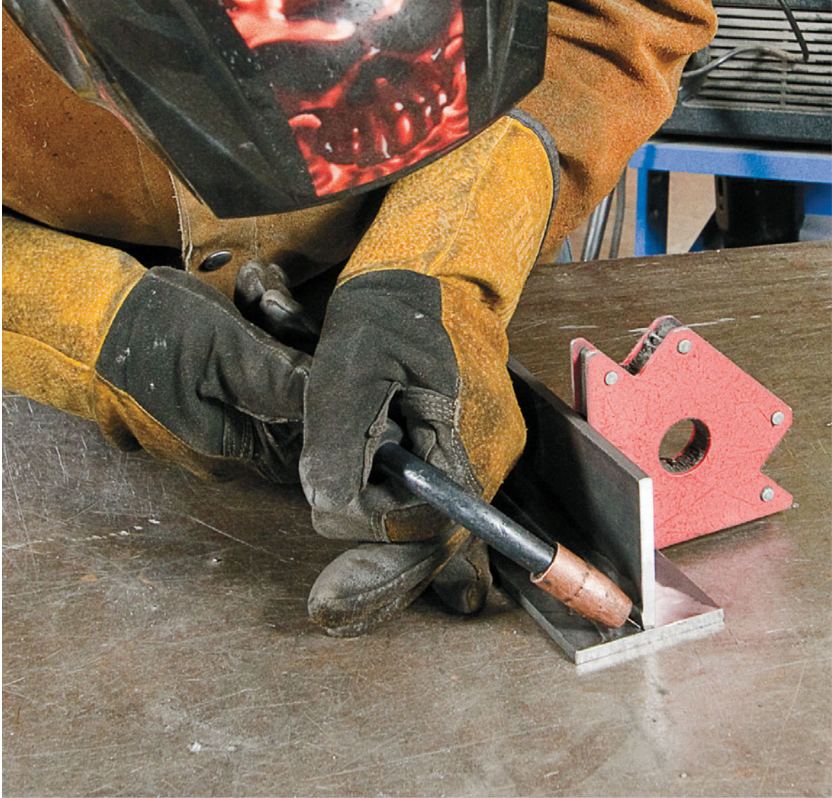
Set up first and get comfortable with the angle you will be welding at.
