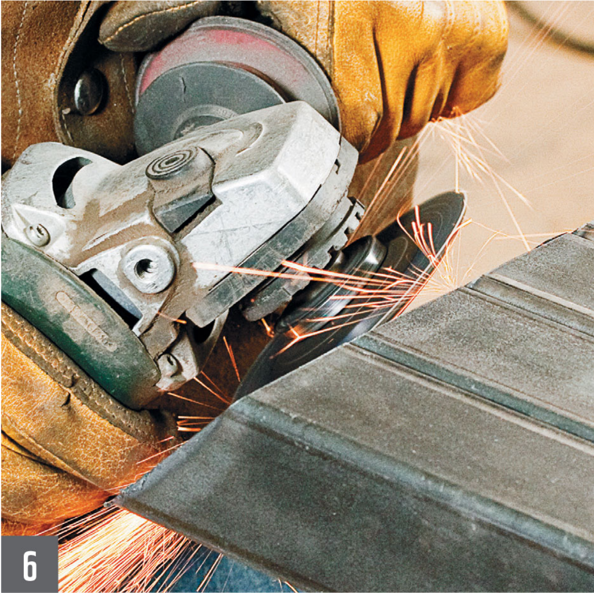
Using the most accurate piece of each series, true up the rest to match that piece.
