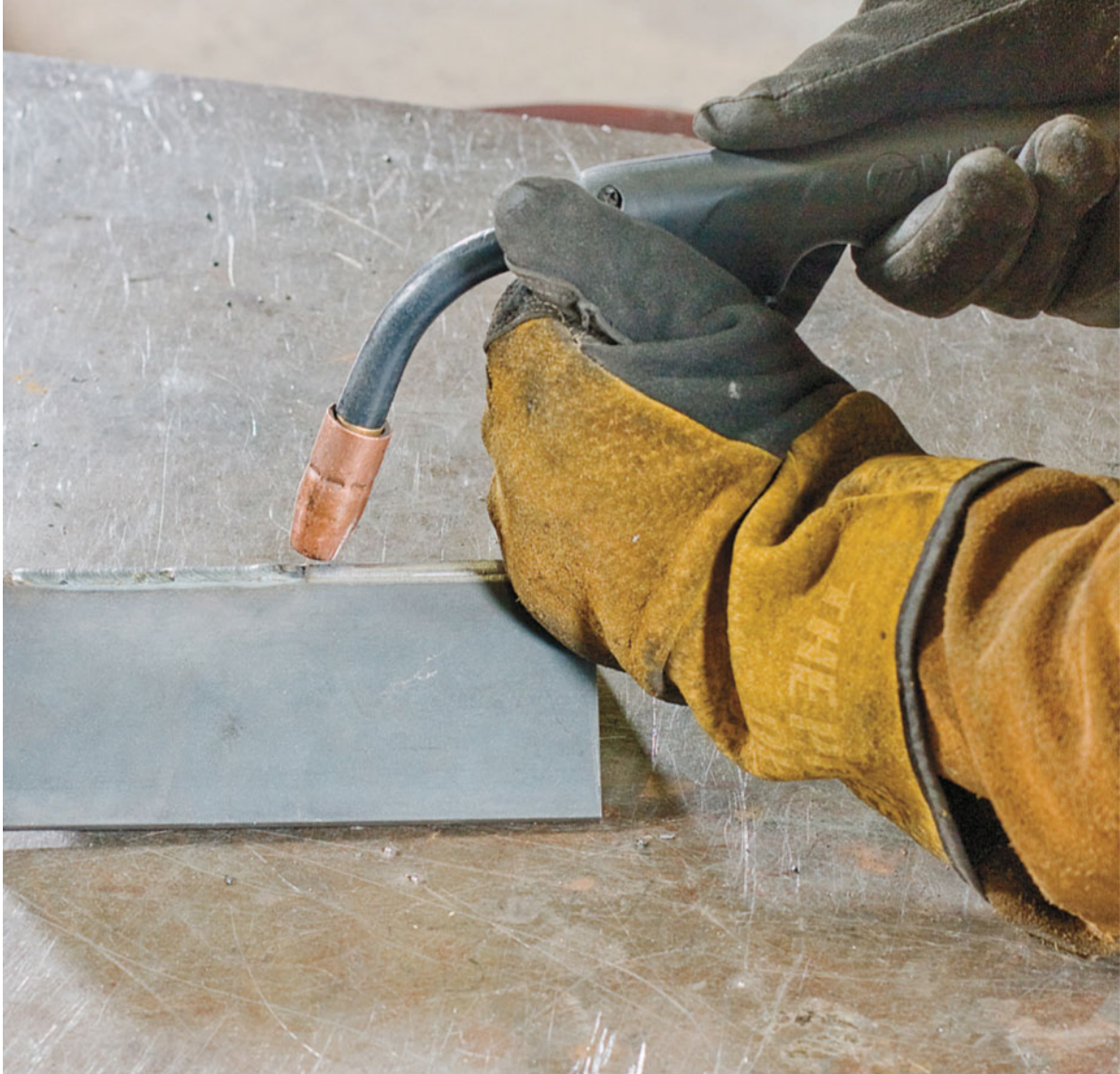
You should have a drag angle of no less than 45 degrees.
