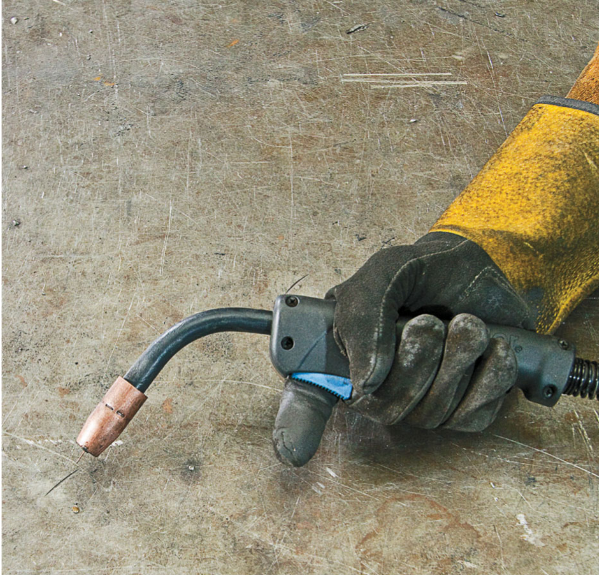
The wire on a MIG welder feeds through the tip of the nozzle.
