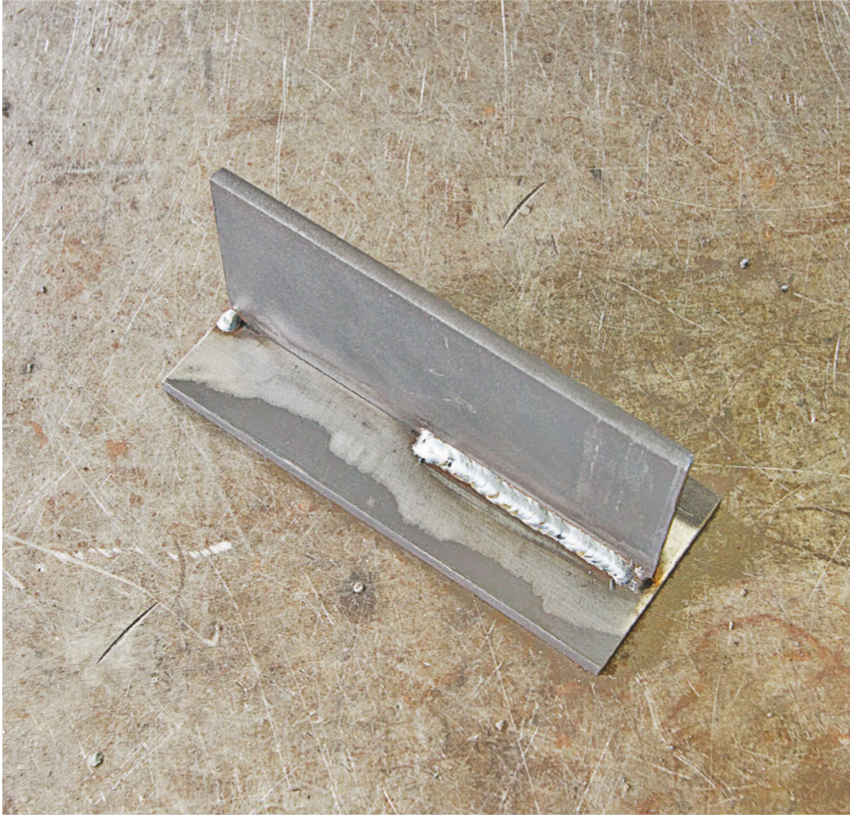
Clean the weld zone with the stainless steel wire brush and then continue the weld.
