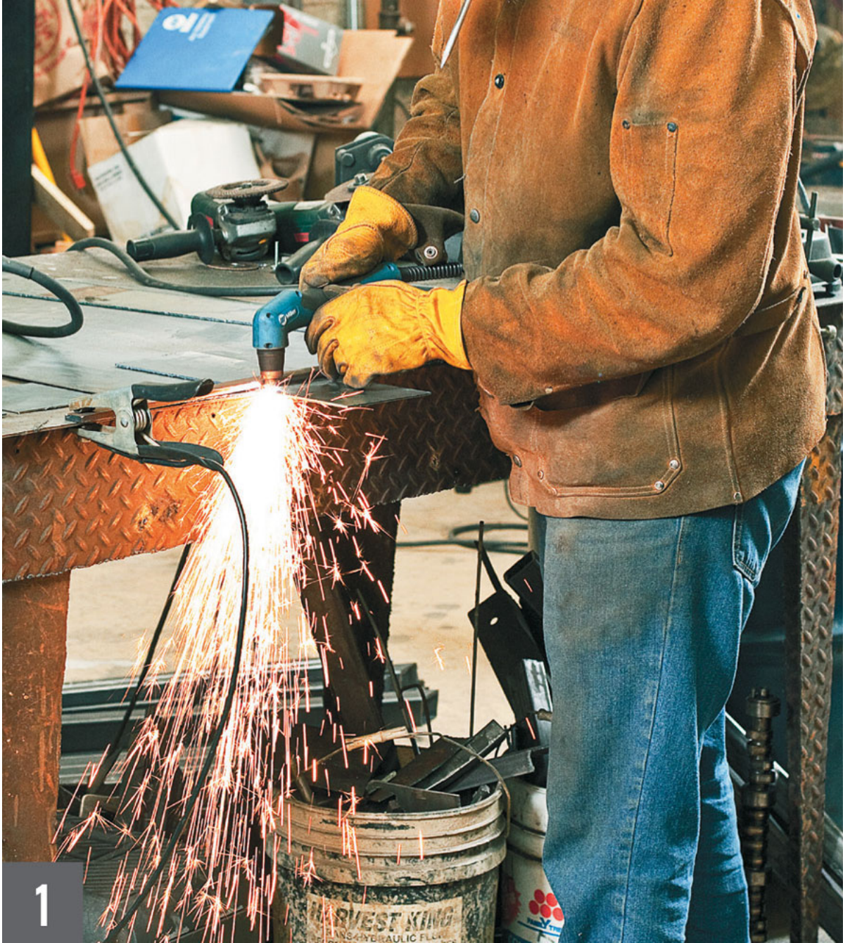
Start the arc off of the piece and move into the cut.
