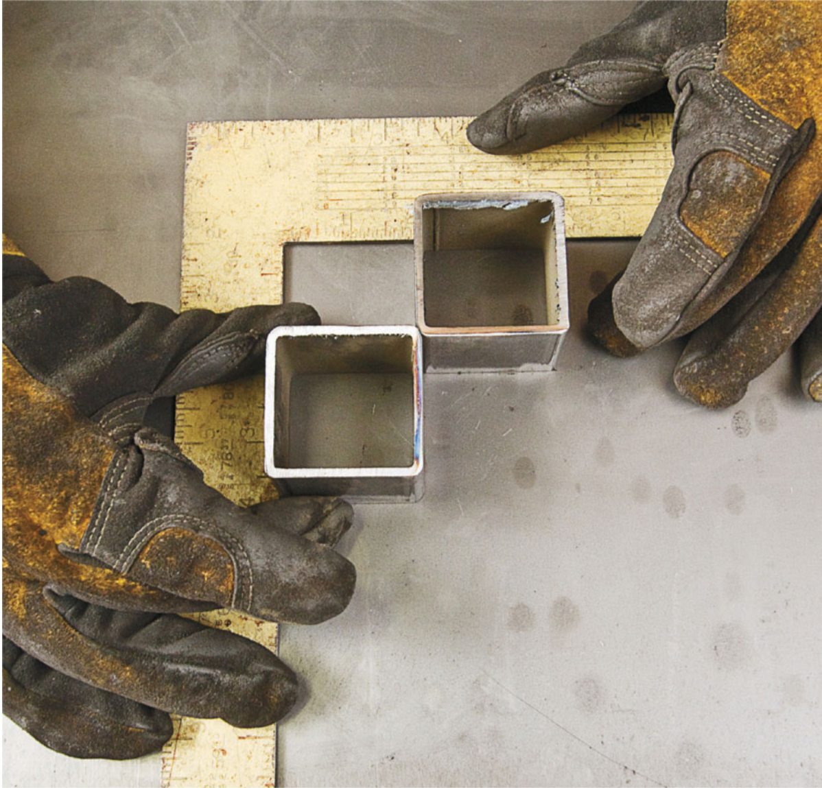
To make a right angle jig, use two pieces of square tube and a carpenter square.
