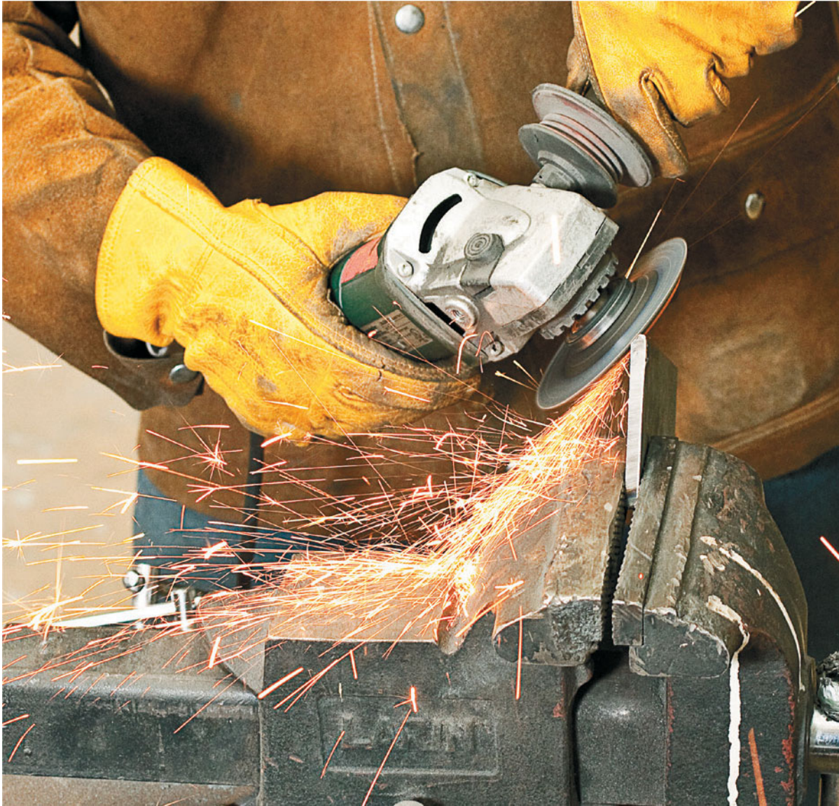
When chamfering, lock in the angles to get a nice flat surface.
