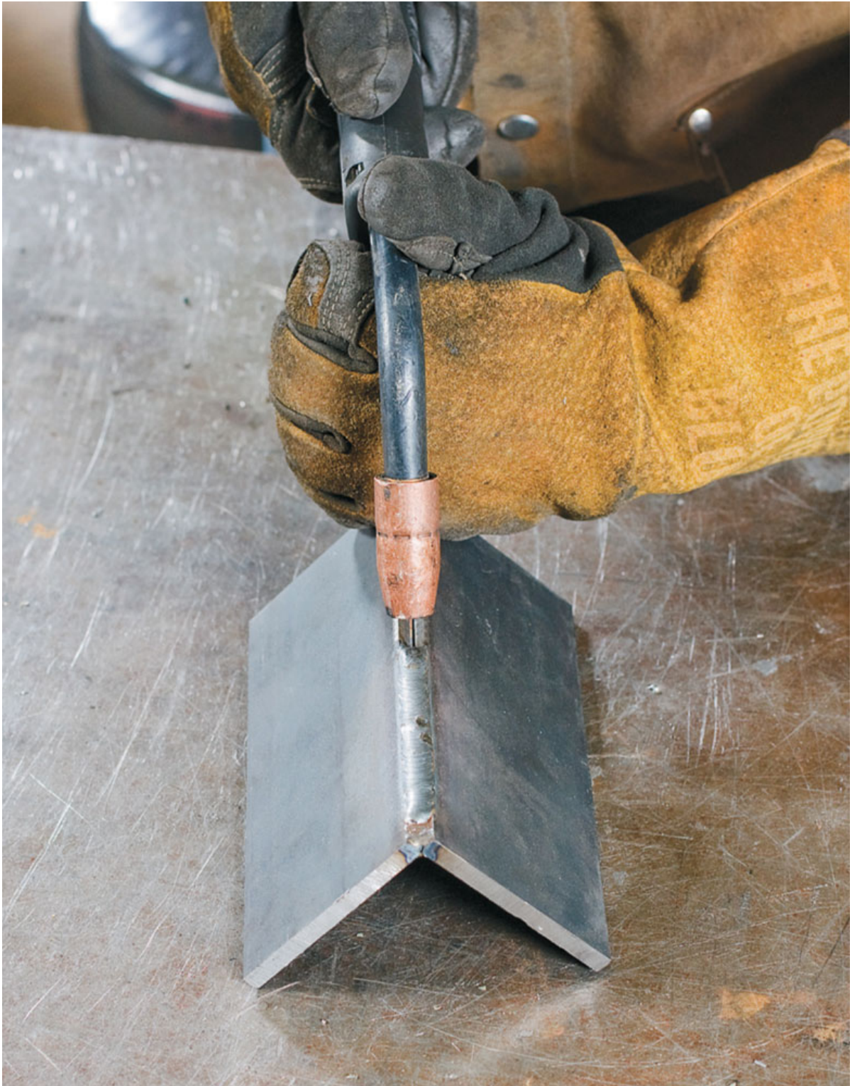
The same rules apply to all of these techniques—straight on and perpendicular so the shield gas hits the puddle evenly.
