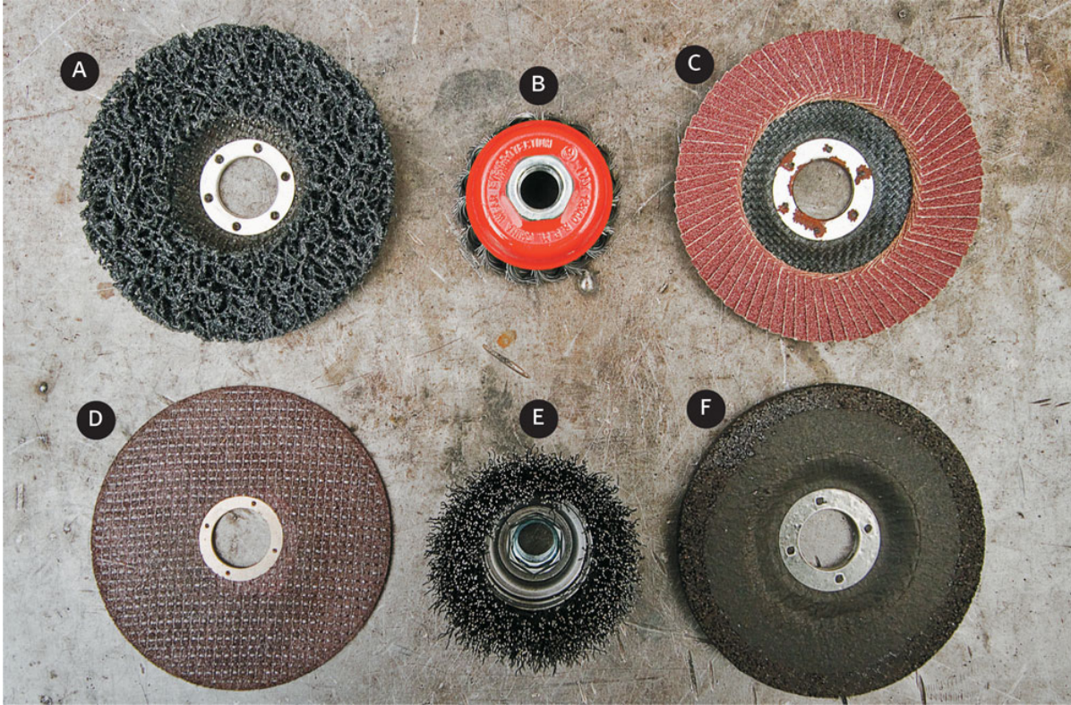
Here are some of the commonly used attachments for an angle grinder: A. Synthetic rust and paint removal disk ; B. Braided cup brush; C. Flap-disk (available in a wide range of grits); D. Aluminum oxide cutting disc; E. Fine wire brush; F. Grinding or stone disk
