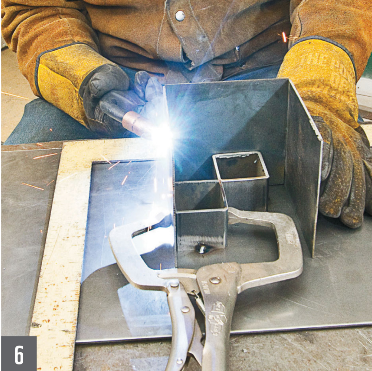
Once one edge is completed, add another side the same way. Clamp and tack in place.
