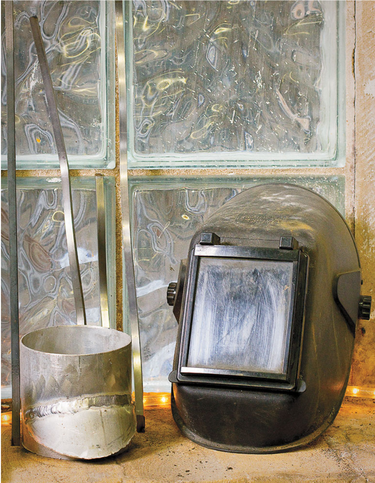
This is a classic single shade (DIN) welding lid. The new auto-darkening helmets allow you to set up with the lid down; the lens darkens as soon as the arc light hits the photo cells.
