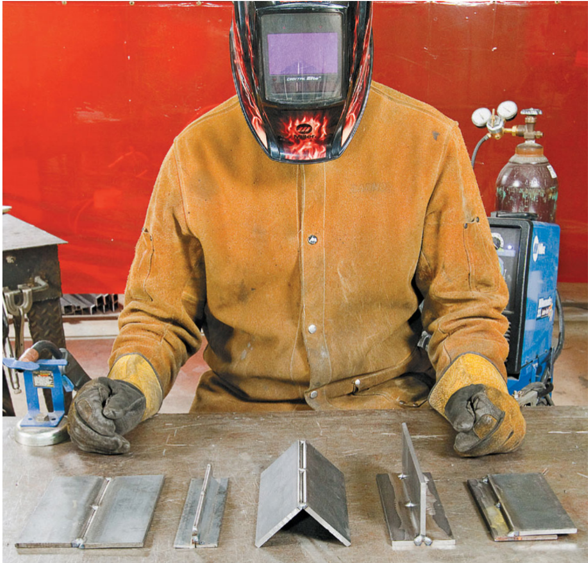
Here all the basic joints are tacked together, prepped, and ready to weld.
