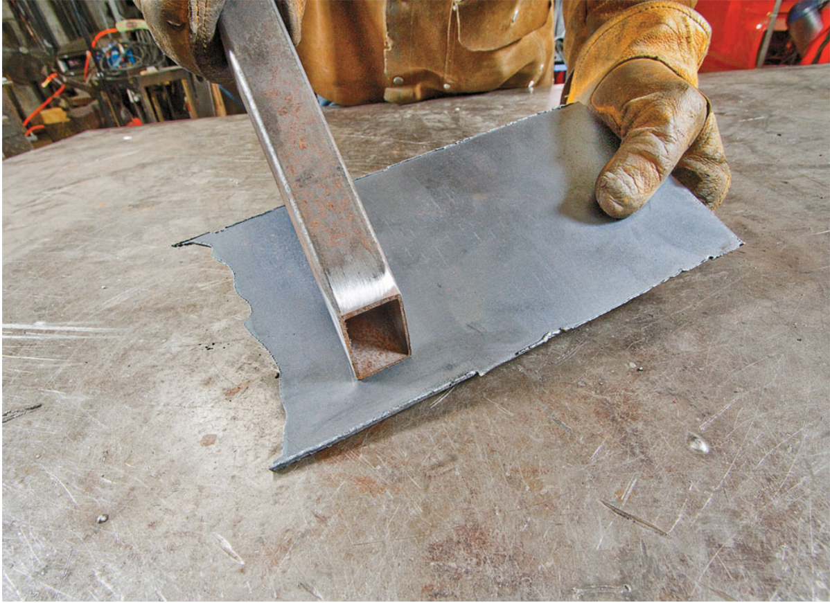
This is dross on the other side of a plasma cut. Use a piece of scrap or a chipping hammer to remove the dross.
