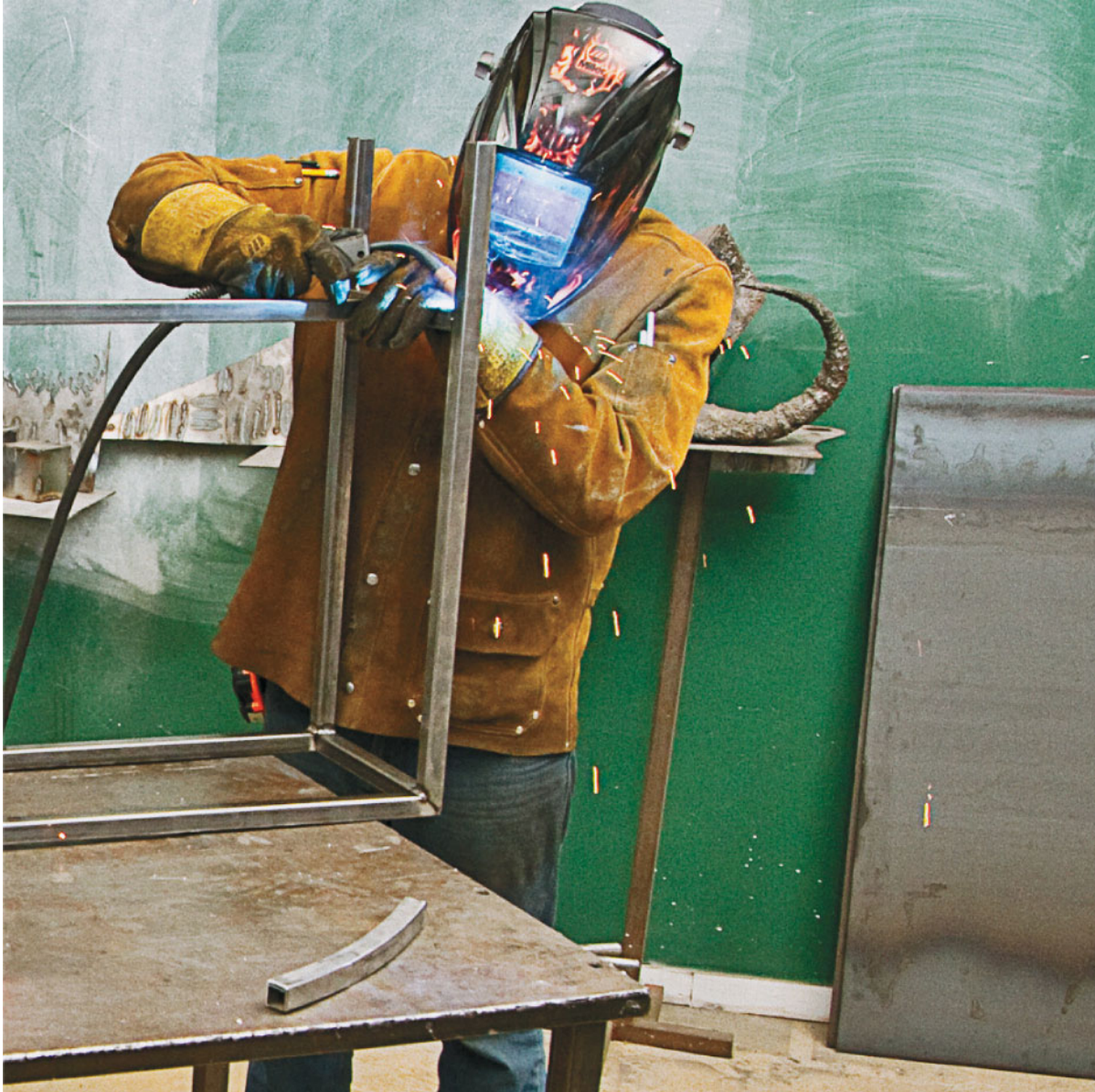
Put yourself in the most comfortable position you can while welding large pieces.
