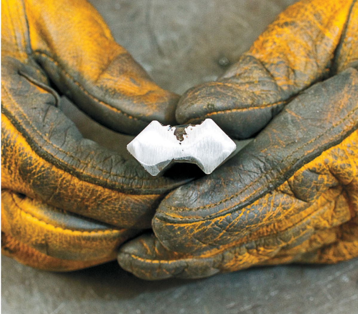
Here is a crosscut of a weld that has deep porosity. This weld is not structurally sound.
