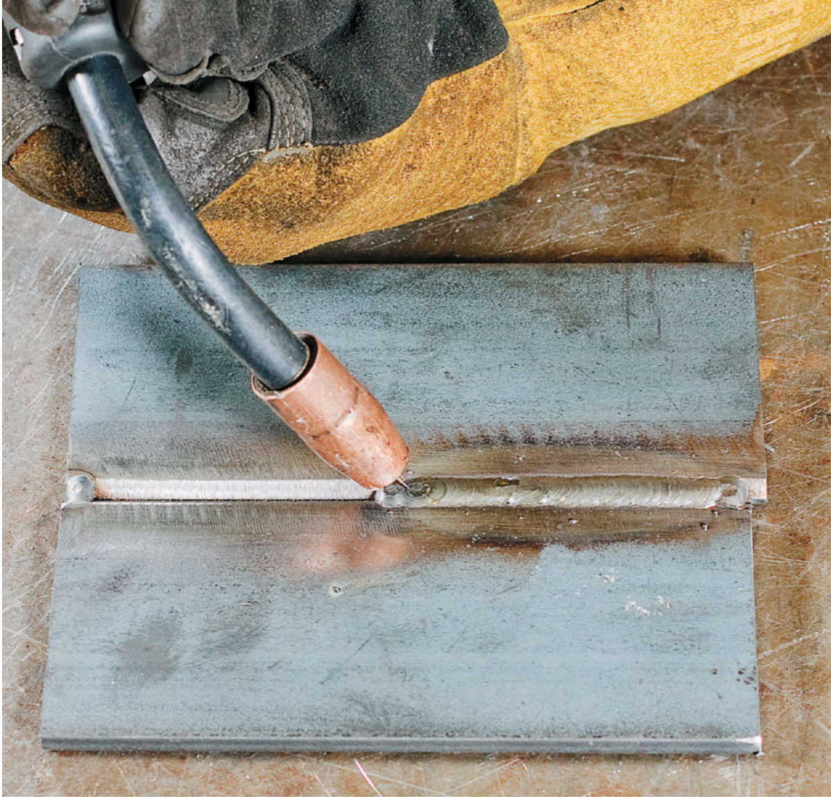
As you can see in this cross body weld, the direction of the nozzle is still straight into the weld and I am perpendicular on both sides. In order to do a cross body weld, I don't break the rules, but I do have to position my trigger hand towards me a little in order to keep those angles and adjust my drag angle.
