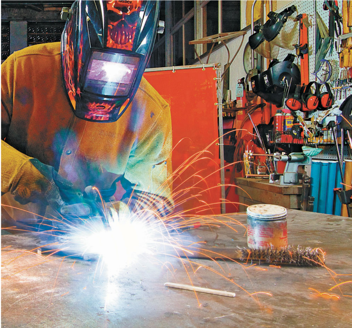
Small molten balls of steel known as "spatter" are ejected from the weld in progress.
