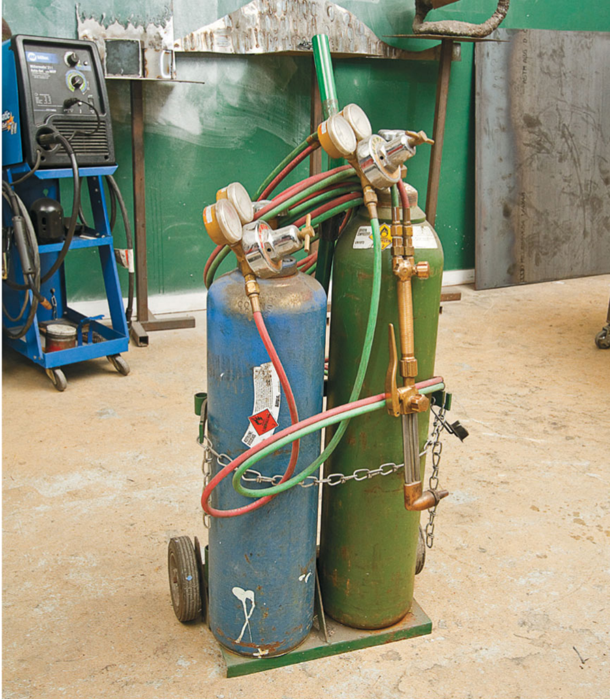
Here is an oxy-acetylene torch setup chained to hand truck. All cylinders need to be chained to something for safety. If a hand truck is not available, chain the cylinders to the wall or stationary table.
