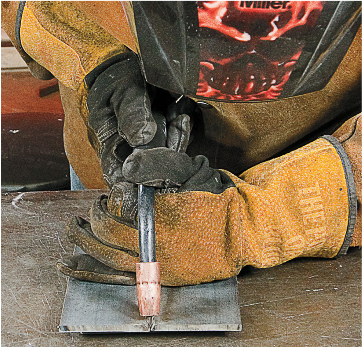
Tack at the top first, then the bottom, and finally the middle.
