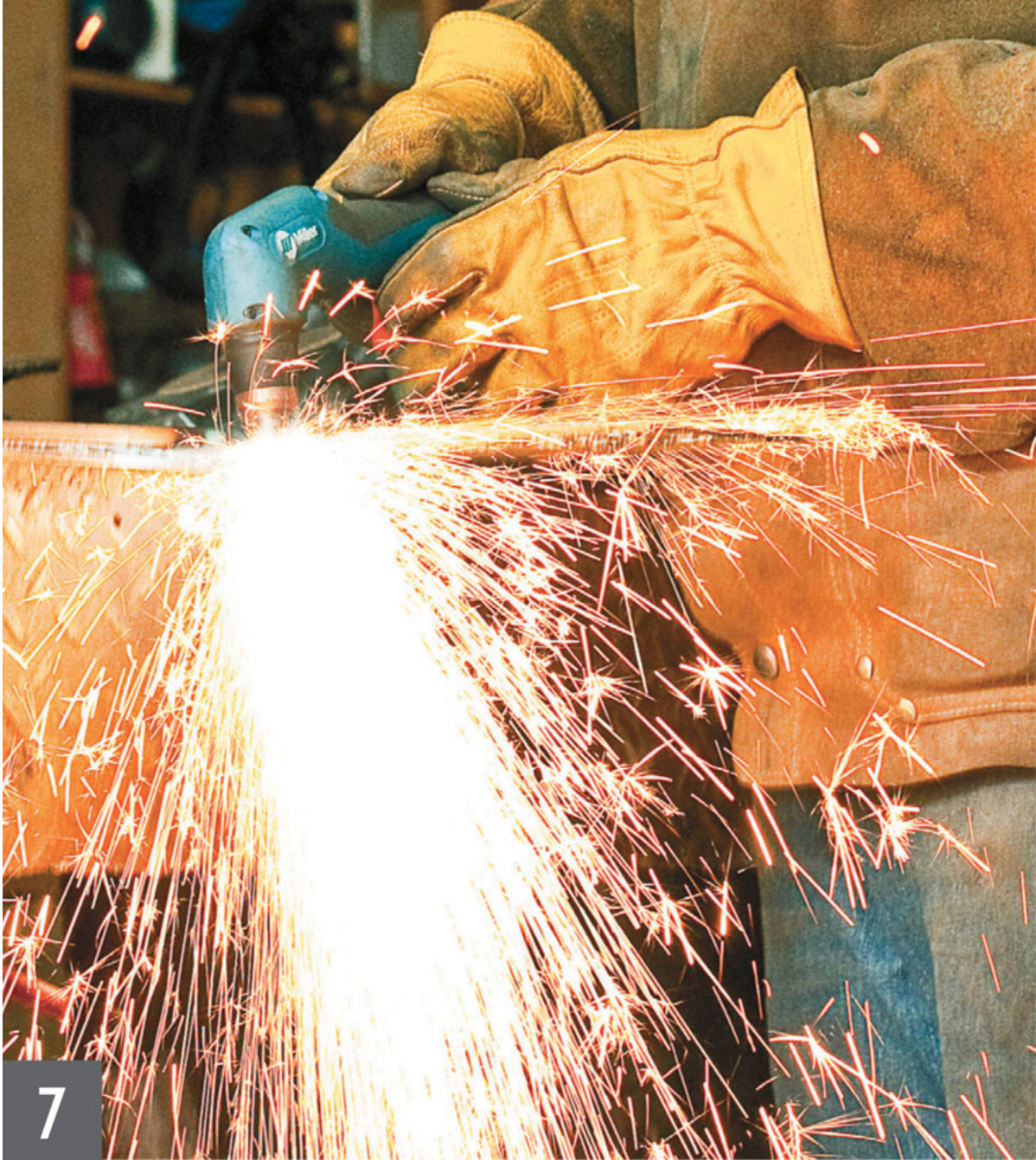
Keeping the center seam of the torch in line with the guide line will help you keep a straighter cut.
