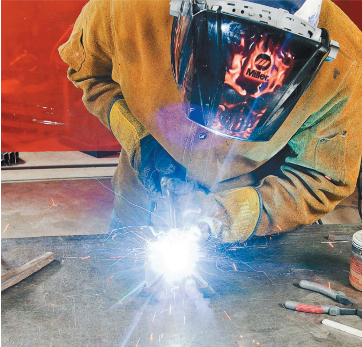
Try to remain braced and supported. If the weld is higher up, find something that height to rest your support hand on that will slide on the table.
