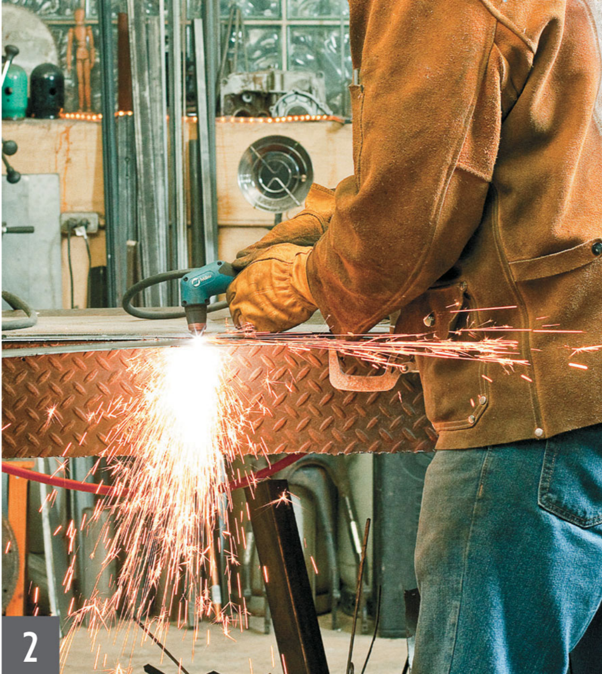
2 Keep the torch perpendicular to the cut.
