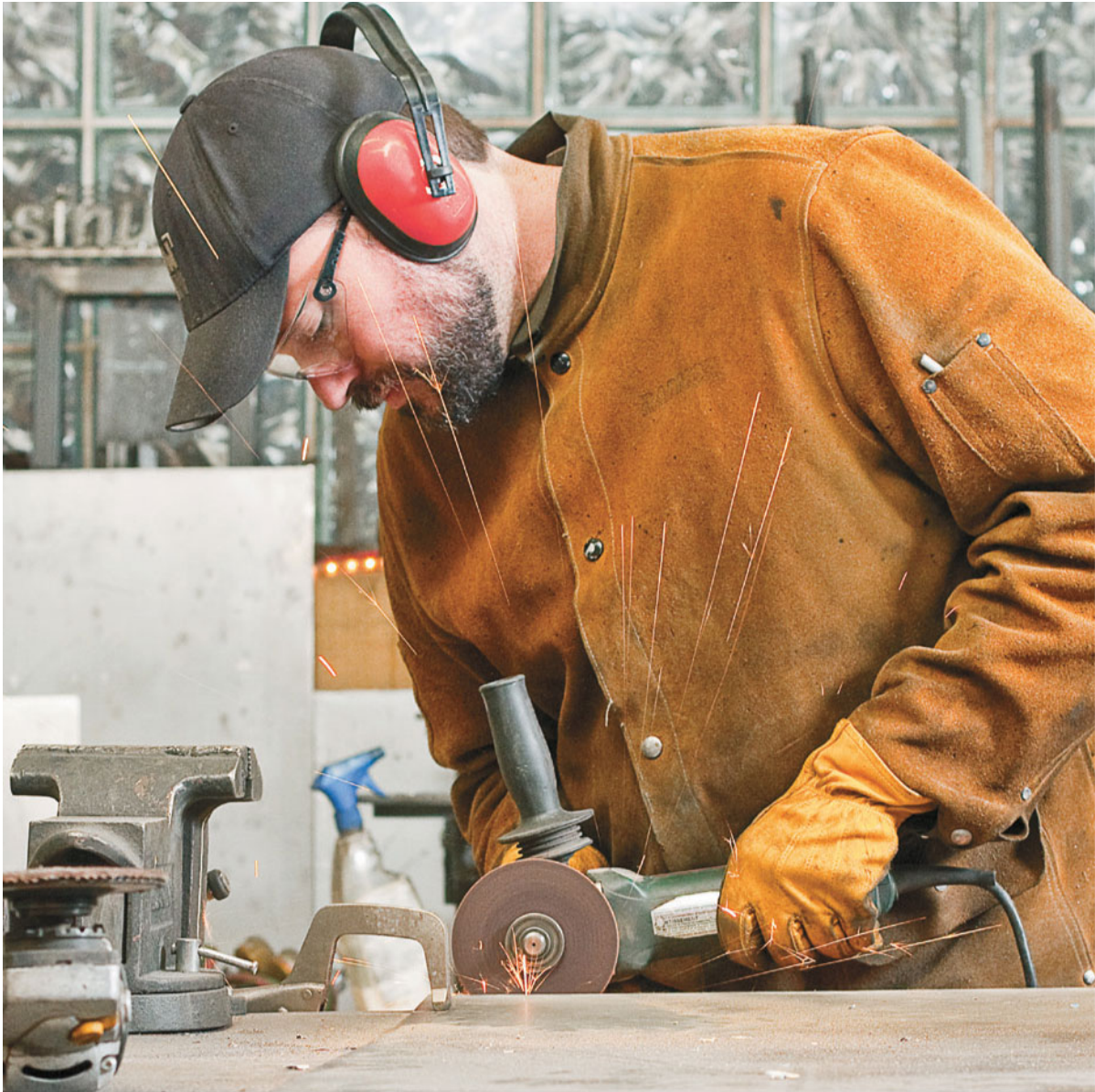
Using a grinder with a cutting disk will allow for straighter cuts. Keep the disk straight into the cut or it could bind or kick.
