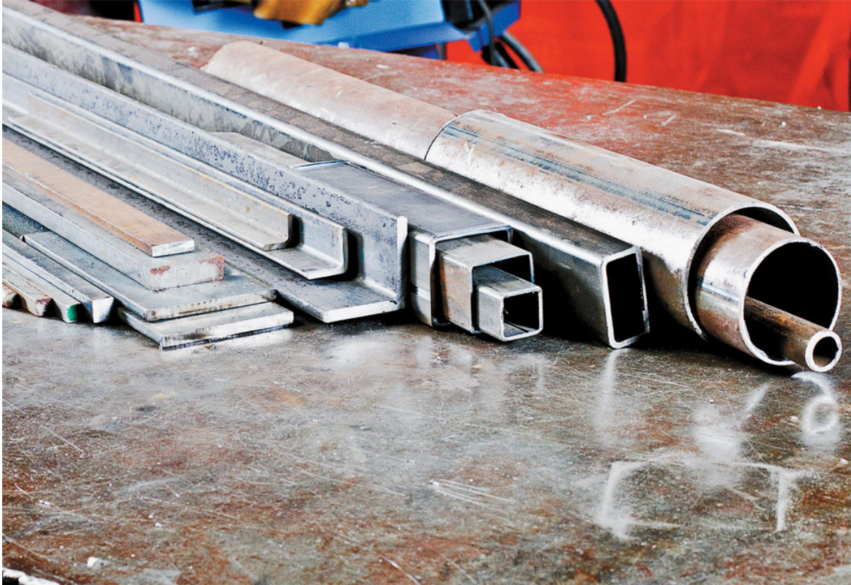
Metal is made in all different shapes and sizes to suit almost any job you can think of. You can find it in plate, bar, angles, and tubes that come in square, round, or rectangle.
