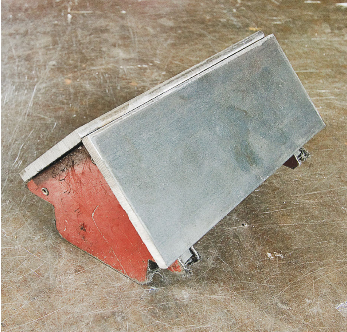
Corner joints like this will use the same shark tooth technique as a butt joint.
