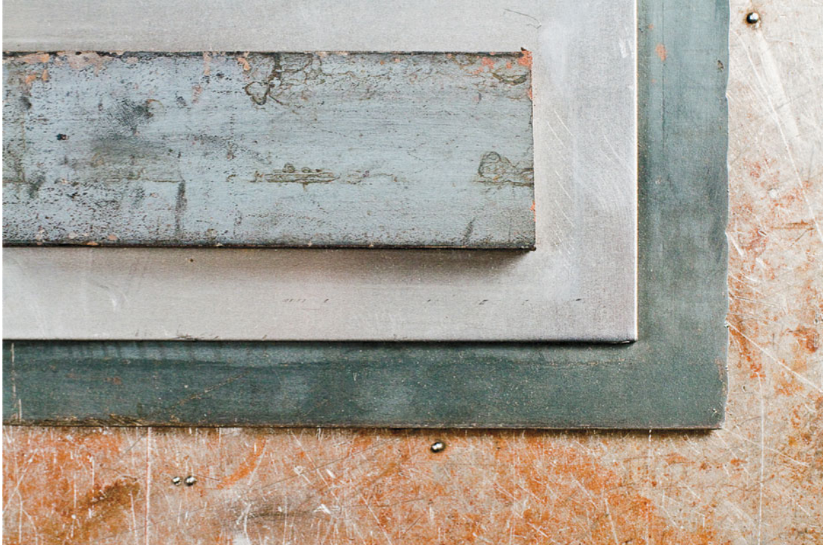
Here you see a piece of cold roll steel between two pieces of hot roll steel. Notice the difference in color. Hot roll has a murky blue/gray patina called "mill scale."
