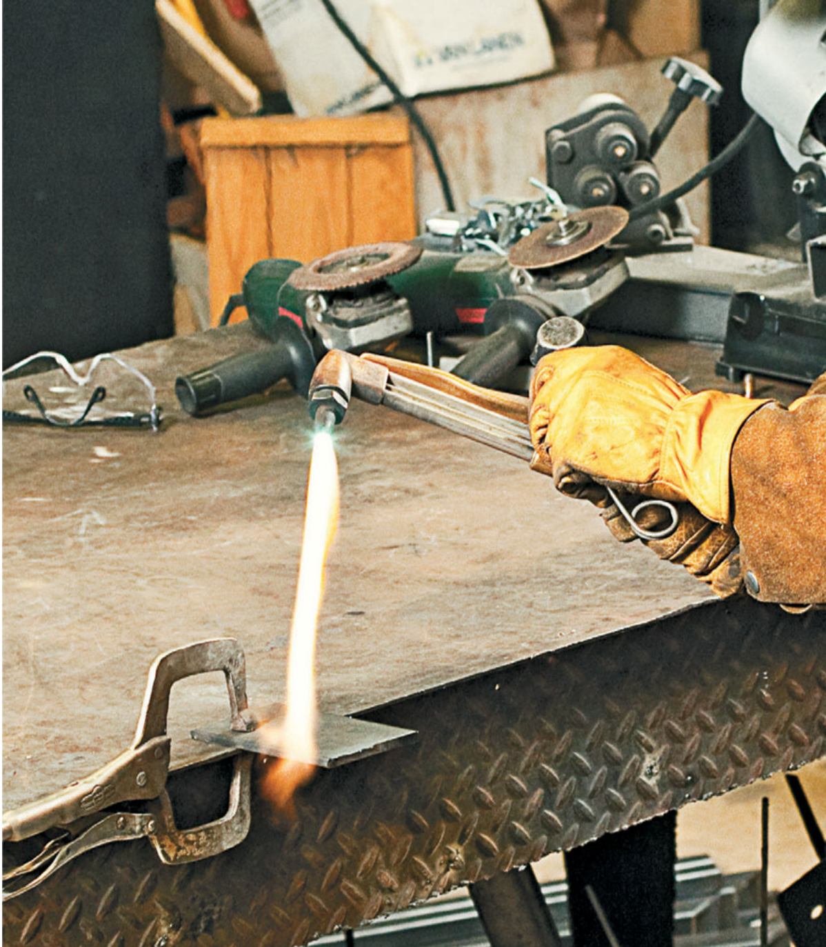
When cutting with an oxyfuel torch, it is necessary to wear proper safety gear. Eye protection should have a 3 to 6 shade DIN.
