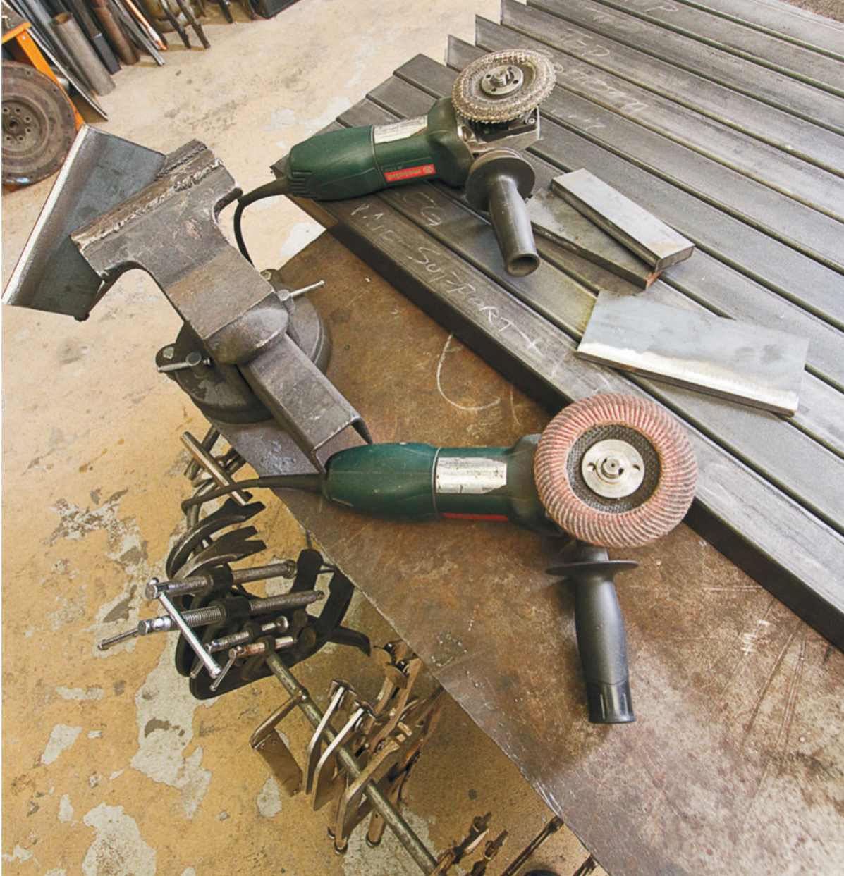
When grinders are not in use, always put them down on the back. Never place a grinder on its front.
