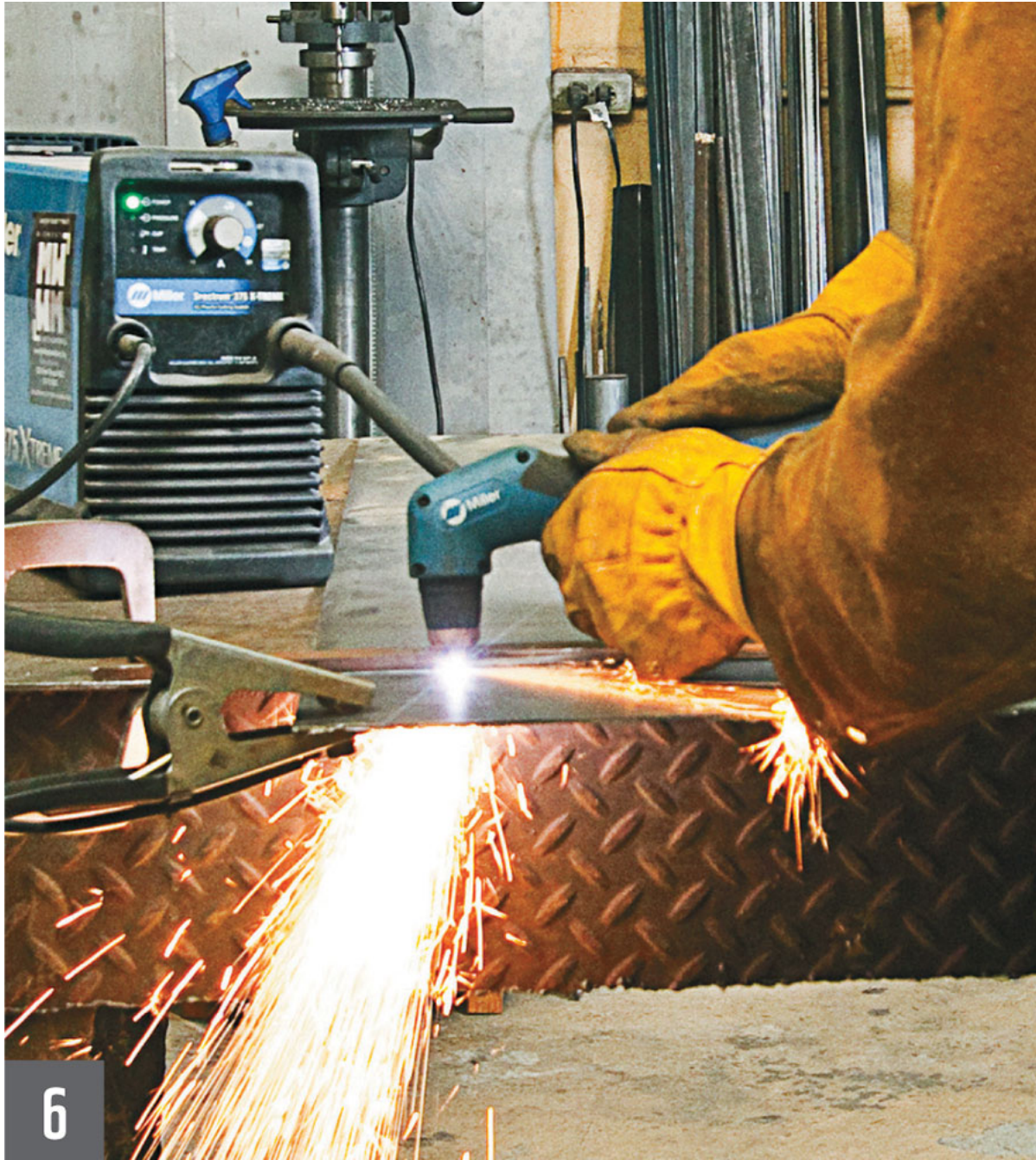
When cutting straight edges with a guide, make sure to measure out from where the drag shield makes contact to the guide to the center of the torch tip for a more accurate cut.
