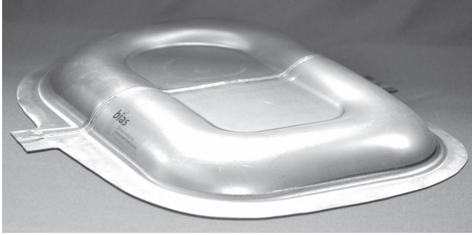
9.11 Aluminium-steel tailored hybrid blank after hydromechanical deep drawing (Courtesy: LFT, Chair of Manufacturing Technology, University Erlangen-Nuremberg and BIAS; Thomy and Vollertsen, 2009).
