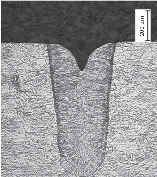
7.31 Undercutting or weld blowout caused by too much power/energy at the workpiece. This leads to vaporisation of material.
