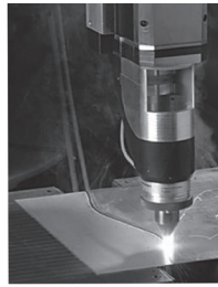
Laser welding 2.2 kW, Ar 15 l/min
