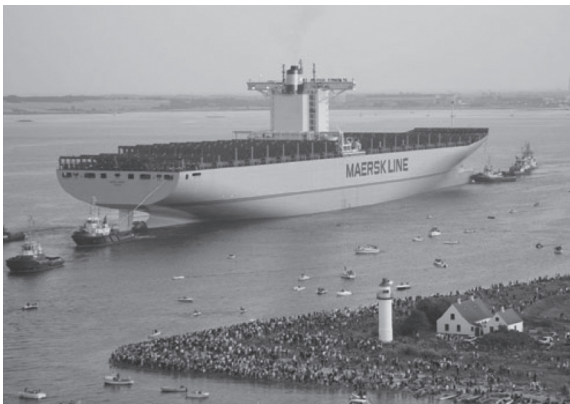
23.11 11,000 TEU container vessel at Odense Steel Shipyard. With 11,000 TEU containers including 1,000 FEU reefers, the ship was in 2008 the world's largest container carrier and reefer vessel. (Courtesy: Odense Steel Shipyard.)
