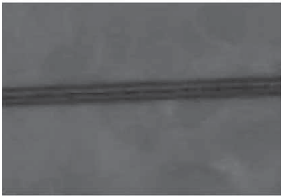
22.6 The influence of welding speed on area of surface quality: (a) P = 2.0 kW, v = 25 mm/s, D_d = 0 mm; (b) P = 2.0 kW, v = 22 mm/s, D_d = 0 mm; (c) P = 2.0 kW, v = 19 mm/s, D_d = 0 mm.
