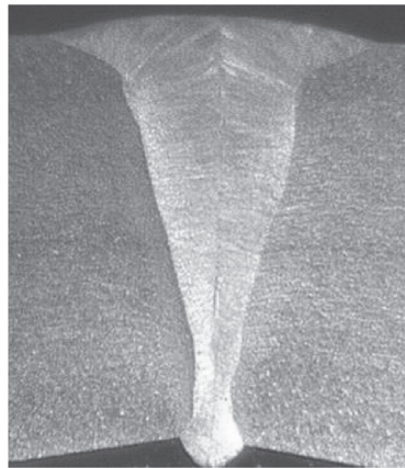
High quality (acc. to ASME section VII, IX) 12 mm stainless steel tube
