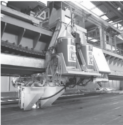
23.8 Photos of the installation as well as of a stiffener welding head and clamping tools. (Courtesy: Guido Pethan, Meyer Werft.)
