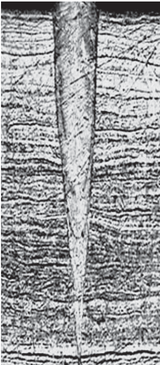
7.17 Cross section of Gaussian beam profile weld; 100 W average power.
