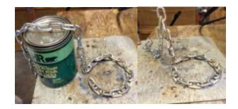
Step 3: After the weld, take away the paint container and make a circle 1 3/8" to 1 1/2" diameter at the top of the "stem" or the draping. Weld the circle. Check the size of the circle with an empty wine bottle. Then wrap the chain around the neck of the wine bottle and weld it all to the dangling end.
