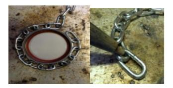
Step 2: Drape the chain over a container that can allow for a good length of draping. An empty paint can is a good option to consider. The chain should be positioned at around an 85-degree angle.
