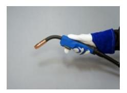
Several MIG welding is achieved using a gas shield; mixes of carbon dioxide and argon/CO2 are very common. There is often a regulator or flowmeter in the gas bottle that helps to set the flow of gas. For light-duty welding, a good rule of thumb requires that you use around 20 cubic feet/ hour of gas flow. You can optimize the amount of gas used when you become skilled with the gun.
