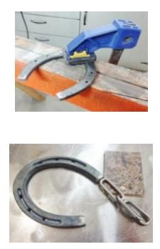
Step 3: Tack the chains to the horseshoe in a particular place. Create full weld beads on the edge to make the chain links stay firmly. Create a permanent open gap of 5/8" inch in between the two tips of the chain. You will get a very tight puzzle. It doesn't require any particular positioning to get it precisely joined together
