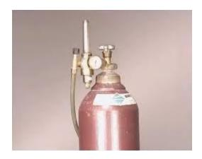
This is a gas that is commonly used in welding. They refer to inert gases that are used in gas metal arc welding. The shielding gases is used to prevent oxygen and water vapor. The shielding gas reduces the quality of the weld, and sometimes, it could also make it stronger. The shielding gas also shields from the environment that can contaminate the metal. Improper choice of welding gas can lead to a splatter.
