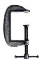
It is preached that you have an assortment of C clamps to save yourself from frustrations. You need the C clamp to secure your work firmly to the table while you cut or make other processes on the metal. Don't mix up the importance of the welding clamp and the C clamp. The C-clamp is majorly used to keep the metal fixed to the work surface, while the Welding clamp is used in holding two base metals together after they have been clamped.
