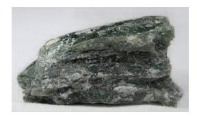
This is a marking tool used to indent a mark on metal when preparing metals before welding. It also helps you to withstand high welding heat. There are also available markers that will help you achieve the exact same result. It is just like the tailor's chalk. If you intend to cut out a particular shape from metal, you just need to draw the shape on the metal using the soapstone and make the cut.
