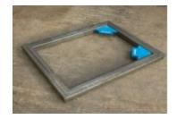
Step 3: Cut down 4 bits of steel at 25cm each for the vertices. Make three legs for the steel. It is more stable than it looks; you don't necessarily need
