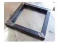
Step 8: Weld all the lower parts of this stool together.
