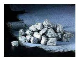
This is a lighter version of aluminum. It actually weighs 2/3 of aluminum. It also absorbs vibration, which makes it very easy to cast. It uses the same method used in welding aluminum. The only difference is its melting temperature. It is usually welded with a Tig welder. Note that magnesium's shavings from its grinding are highly flammable, use a gas shield if you must grind magnesium and don't try to use water to put out the flames.
