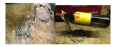
Step 4: Clean up the metal and apply two coats of spray paint. The semigloss black is very attractive. Coat with two coats of clear coat.
