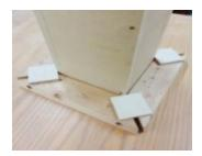
Step 4: With this form, you can't make mistakes on leg location and length. Just lower each leg and cut first. The insides of this form were marked using a paint pen.
