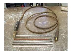
Electrode Coating – This the mixture of minerals that is placed on the core wire. Other chemicals and metallic alloys are also applied.
