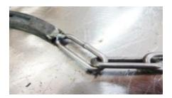
Step 4: Clean up the both sides of this weld with a steel brush.
