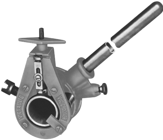
Fig. 9-4 A hand-operated grooving tool (Courtesy of Victaulic Company of America)
