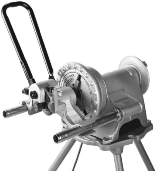
Fig. 9-3 A grooving tool mounted on a power drive
