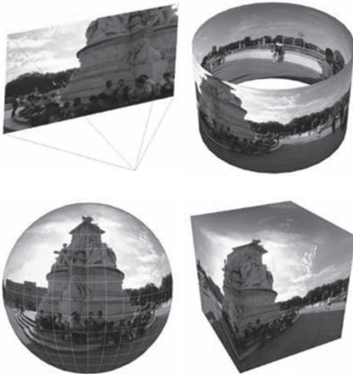
Figure 4. Various forms of panoramas may be created. Typically, they consist of images projected onto various types of surfaces (a) flat (b) cylindrical (c) spherical (d) cubic. (©James Rigg/panoguide.com—reproduced with permission).
