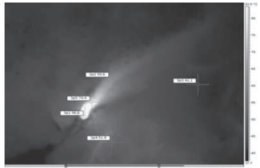
Figure 13. Hottest point (Sp1) temperature observed 96.6 C on rise sidewall of tunnel at 1350.
