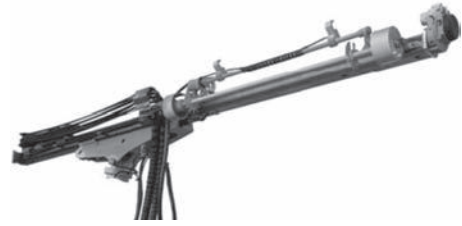
Figure 13. The Rod Handling System, RHS.
