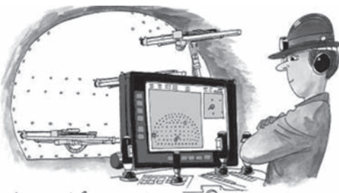
Figure 5. Automated collaring with ABC total.
