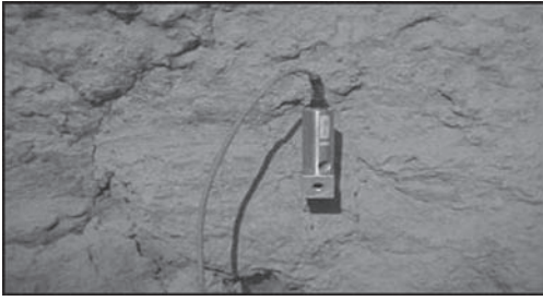
Figure 2. High frequency geophone used for near field monitoring.
