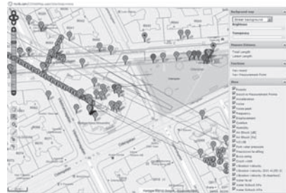
Figure 18. NCVIB: Green X symbols show active measuring points in, under and around Gustav Vasa Church. (Yellow dynamite symbols show blasts and progression.)
