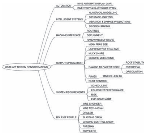
Figure 5. Underground blasting considerations 1.
