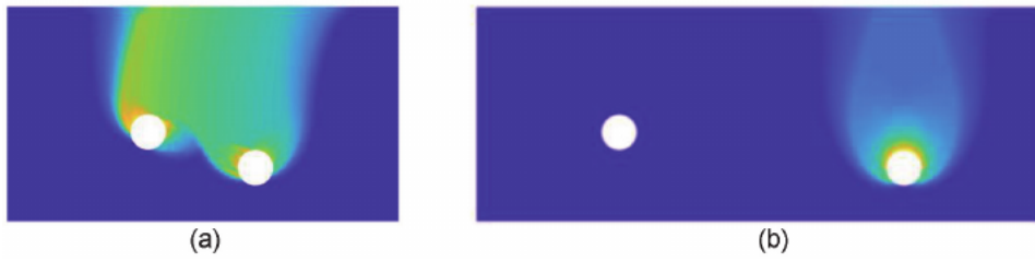
Figure 14. Power dissipation of dual circular tunnels in the case H/D = 3 . (a) H/D = 3 , L/D = 1 , S/D = 3 , \gamma D/c = 1.5 , \phi = 15^\circ . (b) H/D = 3 , L/D = 1 , S/D = 8 , \gamma D/c = 1.5 , \phi = 15^\circ .
