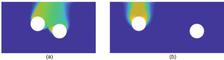
Figure 13. Power dissipation of dual circular tunnels in the case H/D = 1 . (a) H/D = 1 , L/D = 0.5 , S/D = 1.5 , \gamma D/c = 1.5 , \phi = 15^\circ . (b) H/D = 1 , L/D = 0.5 , S/D = 4 , \gamma D/c = 1.5 , \phi = 15^\circ .
