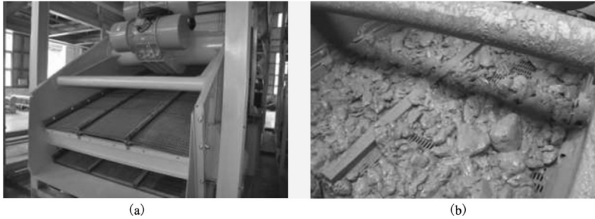
Figure 10.10 Schematic diagram of the screening unit. (a) Double-layer vibration screen. (b) Stainless steel tensile sieve plate.
