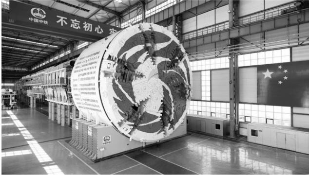
Figure 1.15 The large-diameter slurry shield independently developed for Shenzhen Chunfeng Road Tunnel Project, China.
