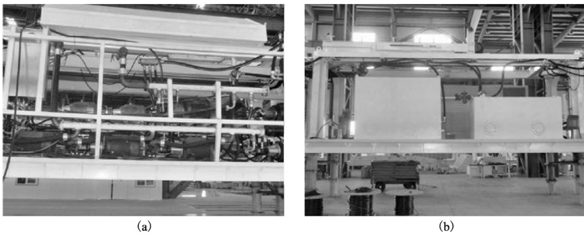
Figure 3.23 Layout of the backup system of the shield machine. (a) Hydraulic power unit. (b) The control room.
