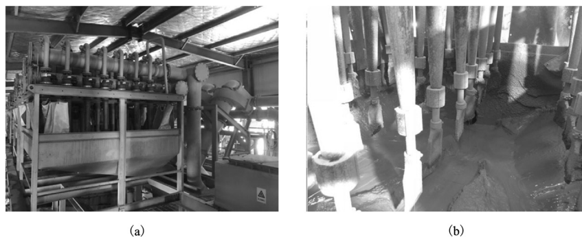
Figure 10.11 Schematic diagrams of primary and secondary cyclones and vacuum adjustment device. (a) Primary and secondary cyclones. (b) Vacuum adjustment device.
