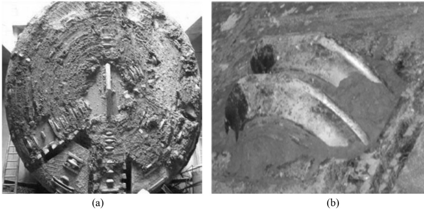
Figure 9.1 Clogging on cutterhead and cutters. (a) Clogging on the cutterhead. (b) Eccentric abrasion of cutters due to clogging on the cutter seat.
