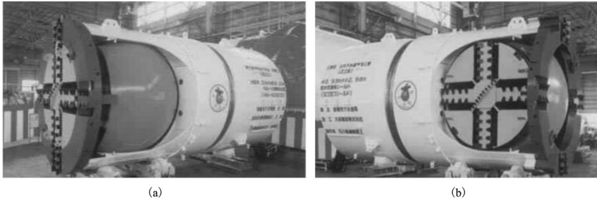
Figure 3.33 Horizontal-horizontal shield machine. (a) Cutterhead in the forward direction. (b) Cutterhead rotates 90°. From Chen K., Hong K., Wu X. Shield Constr Technol. Beijing: China Communications Press; 2016.
