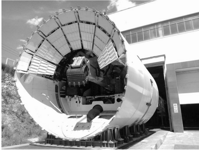
Figure 1.14 The open-shield machine used in construction of Beijing Metro Line 6.
