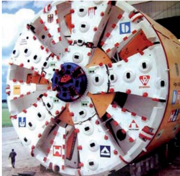
Figure 4.2 The 14.2 m-diameter Herrenknecht Slurry Shield model S-108, used for excavating the Elbe tunnel in Hamburg.
