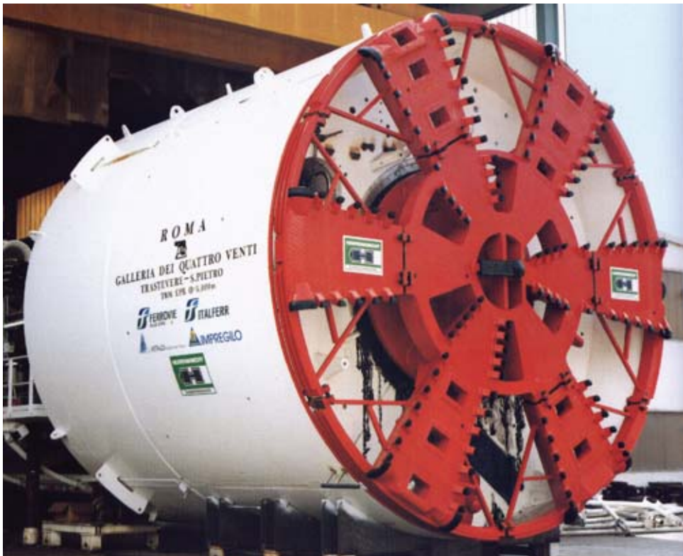
Figure ap.2.2 The 7,97-m diameter Herrenknecht Earth Pressure Balance Shield which operated in Galleria Quattro Venti project.
