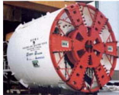
Figure ap.7.10.1 The TBM for excavating the “Quattro Venti” tunnel.
