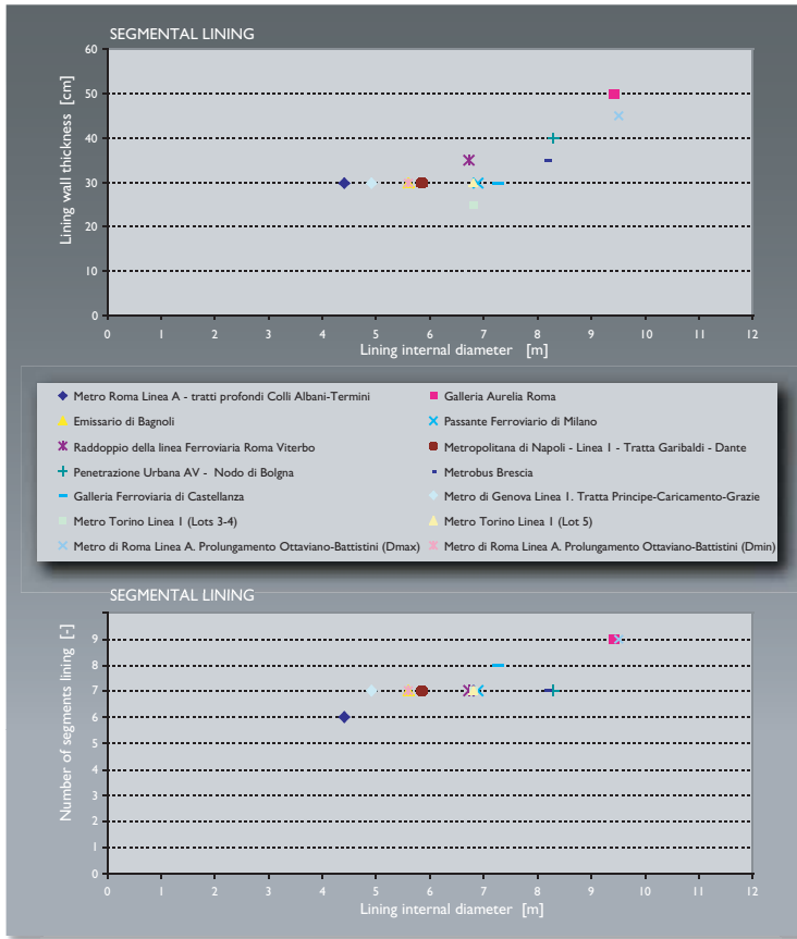
Figure 5.58 Relation between internal diameter and (a) lining thickness, (b) number of segments.
