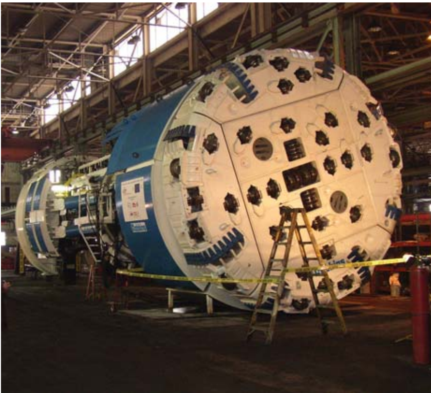
Figure ap.2.5 The Robbins Hard Rock TBM supplied for the excavation of Venaus explorative tunnel.
