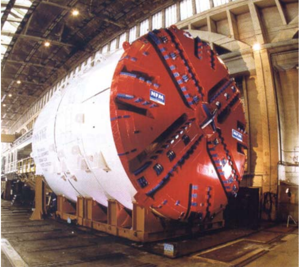
Figure ap.2.3 The 8.03-m diameter NFM Earth Pressure Balance Shield which operated in Milan railway system.
