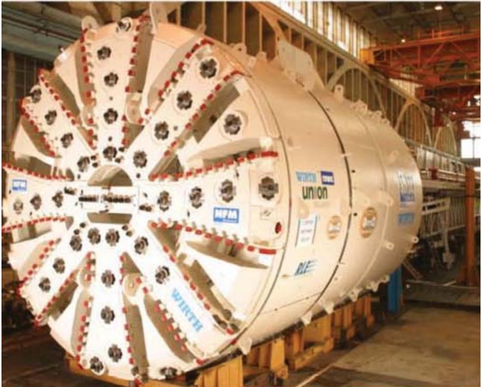
Figure ap.2.4 The 8.17-m diameter WIRTH Earth Pressure Balance Shield which operated in Channel Tunnel Rail Link.
