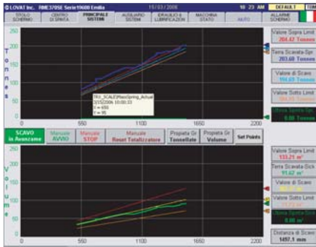
Figure 6.23c Example of the use of screw conveyor for controlling the material extraction.
