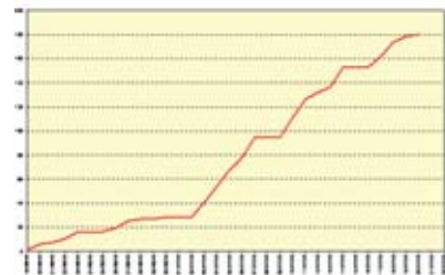
Figure ap.7.13.7 Advancement of the TBM operating at Brescia metro site.
