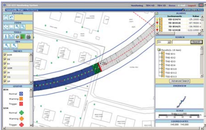
Figure 8.52 Enlargement of Figure 8.50 showing: (1) the position of the face and (2) the installed and the indicated, future rings.
