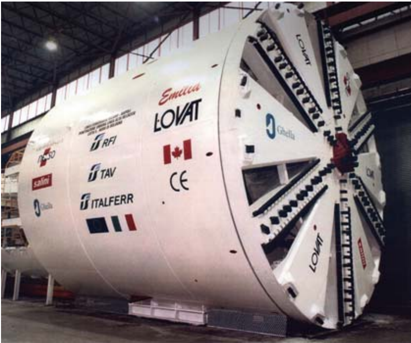
Figure ap.2.1 The LOVAT 9,4 m diameter Earth Pressure Balance Shield machine which operated in Bologna Railway system.
