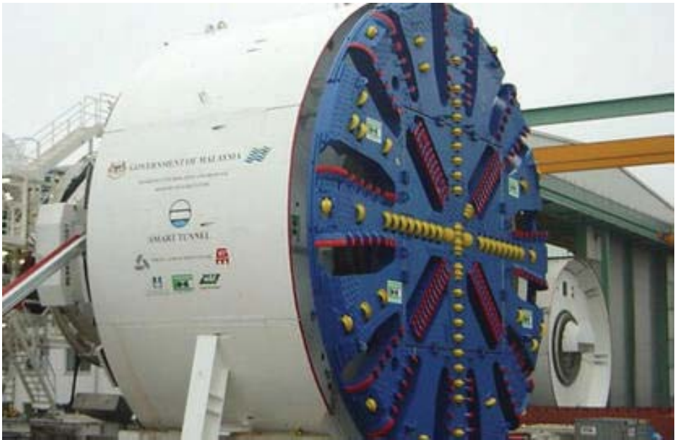
Figure 8.49 One of the two Herrenknecht (13.26-m diameter) Mixshields.
