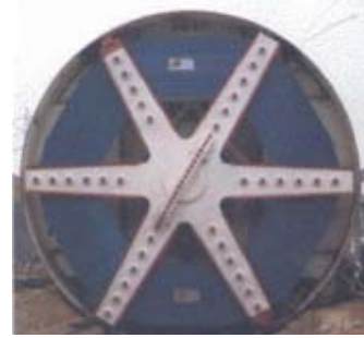
Figure ap.7.5.1 The TBM for excavating the LTR tunnel.
