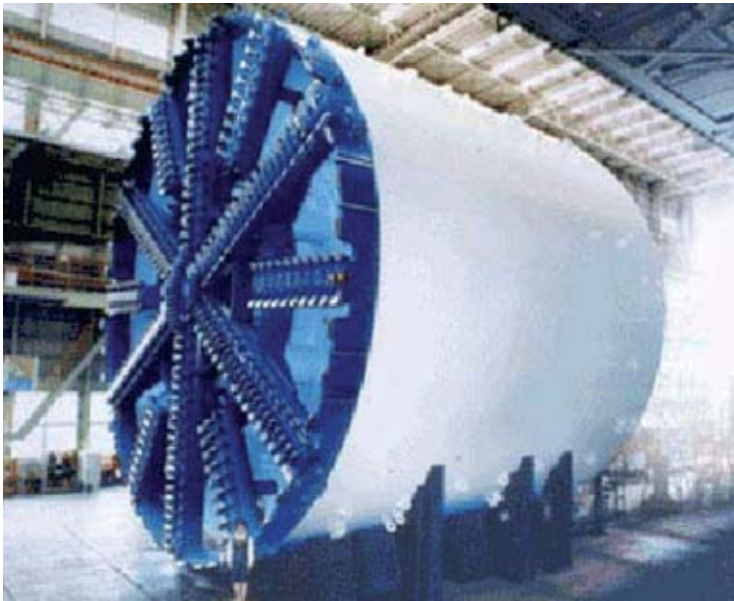
Figure 4.15 The Mitsubishi 15.1 m diameter EPB machine used in Calle 30 Project in Madrid.
