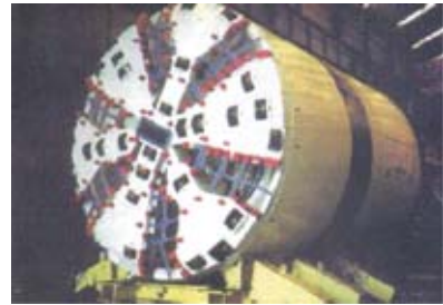
Figure ap.7.8.1 The TBM for excavating the tunnel.
