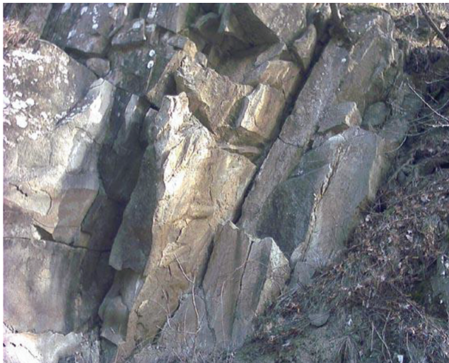
Figure 3.9 Example of geostructural survey. Lithology: 'Arenarie di San Salvatore' (sandstones) URV (unitary rock volume) ( \text{m}^3 ): 0.22.
