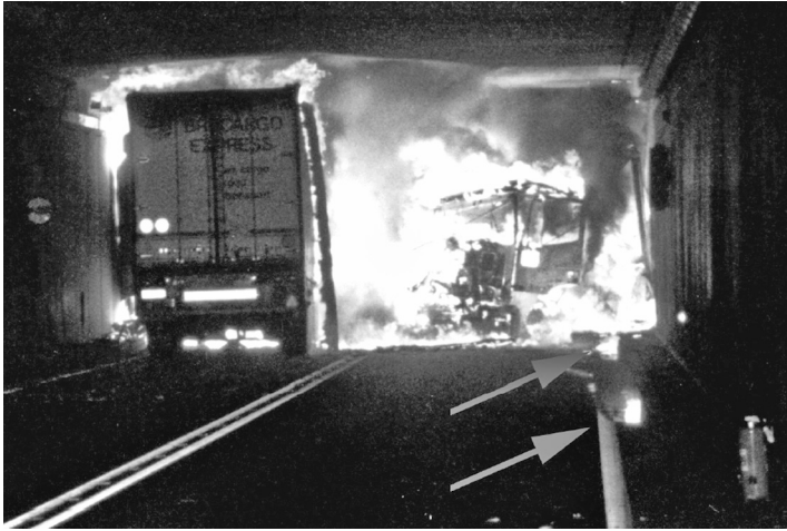
Figure 3.9 Photograph showing HGVs 1 and 2 during the fire. The burning liquid in the gutter is indicated. (Photograph courtesy of Mr C. Grassi.)
