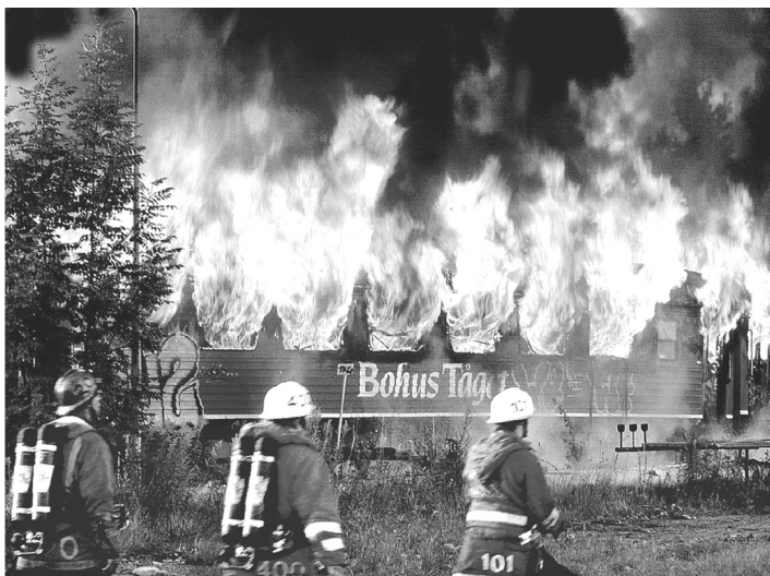
Figure 13.3 A fully developed fire in a train coach (Photograph courtesy of Tomas Karlsson)
