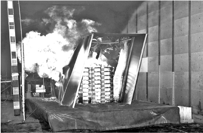
Figure 12.2 Fire experiment with wooden pallets and an aluminium covering carried out in the second Benelux Tunnel, The Netherlands (Photograph courtesy of Steunpunt Tunnelveiligheid, Rijkswaterstaat, The Netherlands)
