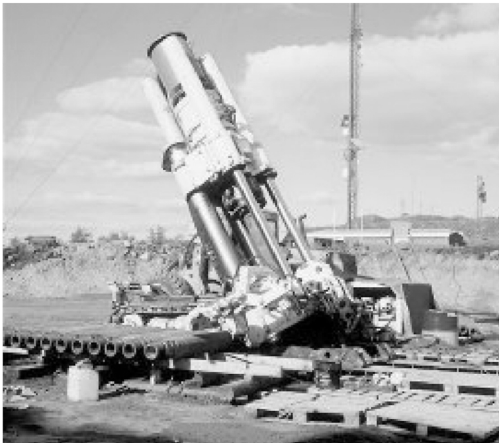
Figure 9.6 The most popular and widely-used model, the Robbins 73RM is considered a reliable workhorse for virtually any raise-boring application. It is a medium-sized raise drill, 1.8–3.1 m in diameter (courtesy of Atlas Copco AB)
