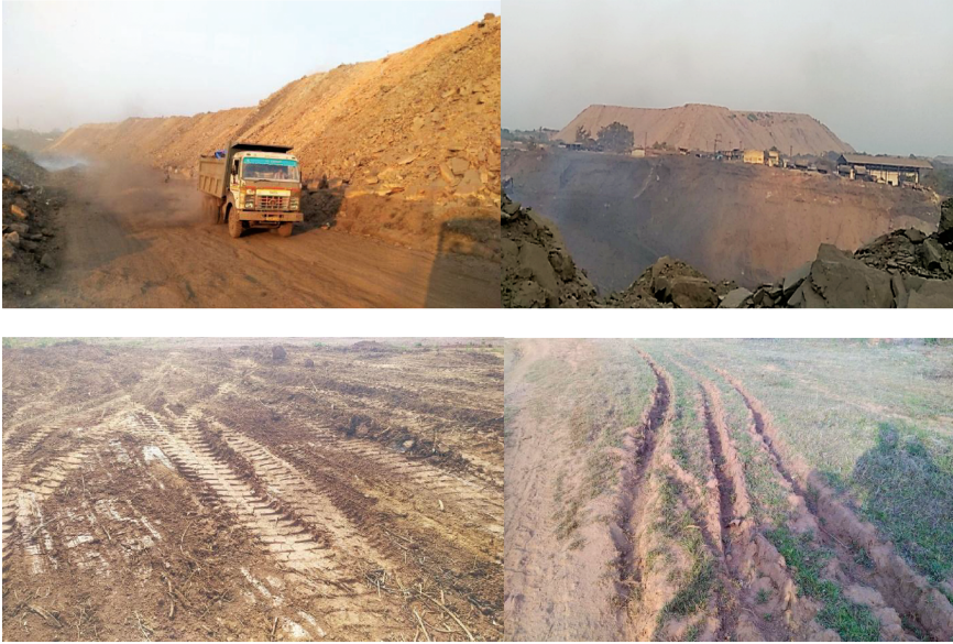
Figure 4.3 Land degradation by mining activities, overburden, and soil compaction due to the movement of heavy traffic in different mining sites of Jharkhand, India
