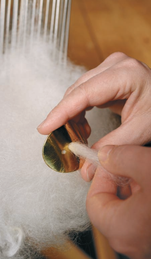
Using the diz to create roving from the combed fiber
