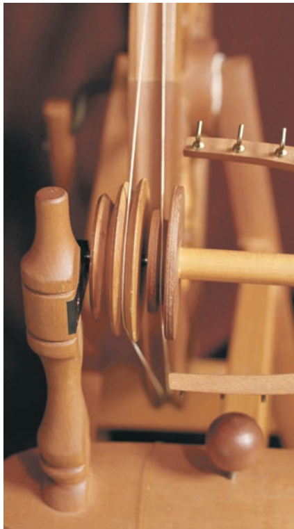
Double drive placement on Ashford wheel
