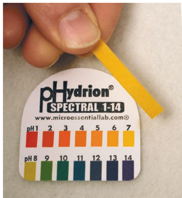
Using a pH tester in dye bath—7 is neutral pH.
