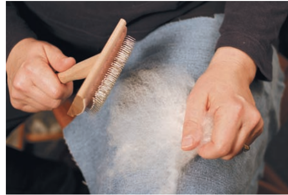
The flick carder process involves hitting the fiber tips with the carder using a snapping motion.
