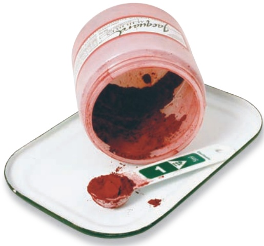
Powdered dyes are easy to measure and dissolve quickly in hot water.
