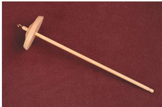
This top whorl spindle is convertible and may also be used as a bottom whorl spindle (as shown in the photo at the upper left).
