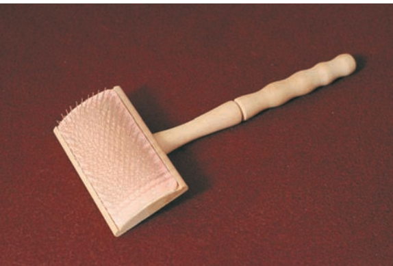
Flick carders help to align fibers for worsted spinning.
