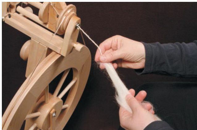
Repairing a singles break
