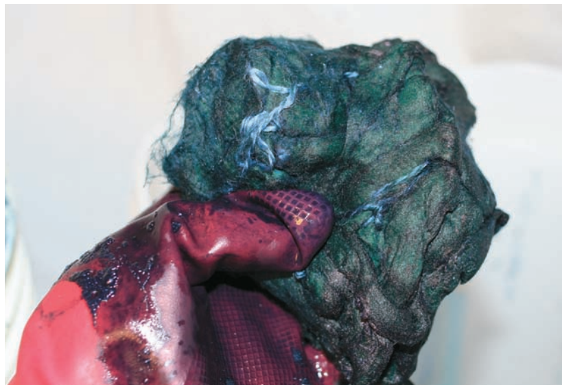
The dipped cotton roving immediately turns blue when pulled out of the vat.
