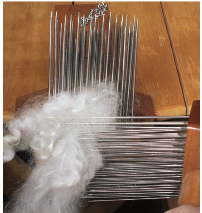
(2) First half pass combing direction is sideways (right to left or left to right)
