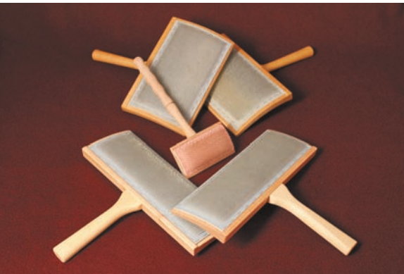
Hand carders—Top: standard wool carders; middle: flick carder; bottom: cotton carders.
