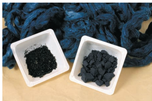
Pre-reduced indigo powder on left and pure indigo crystals on right
