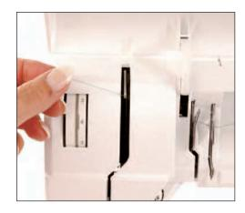
Once you have the thread through the take-up lever, guide it downward toward the needle. There are usually two thread guides before the thread goes to the needle. One may be on the front of the machine, and one is just under the machine body, almost hidden if you aren't looking for it.
