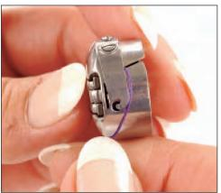
Hold the bobbin case by the latch to insert it back into the machine.
