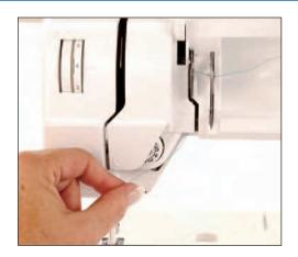
**5** Guide the thread upward to the take-up lever. The take-up lever may have a slot in it to slide the thread in, or you may have to thread it like a needle eye.
