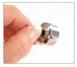
The bobbin tail thread is then threaded though the case slot and tension spring.
