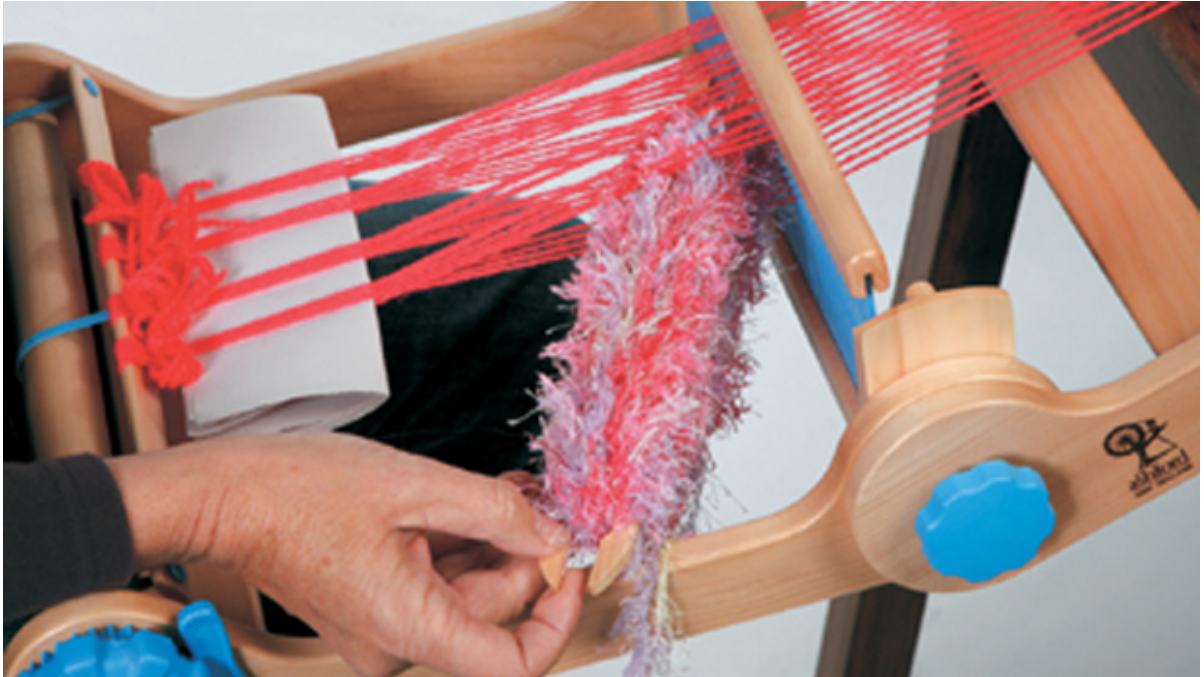
The shuttle is passed through the open space between warp yarns to create fabric.
