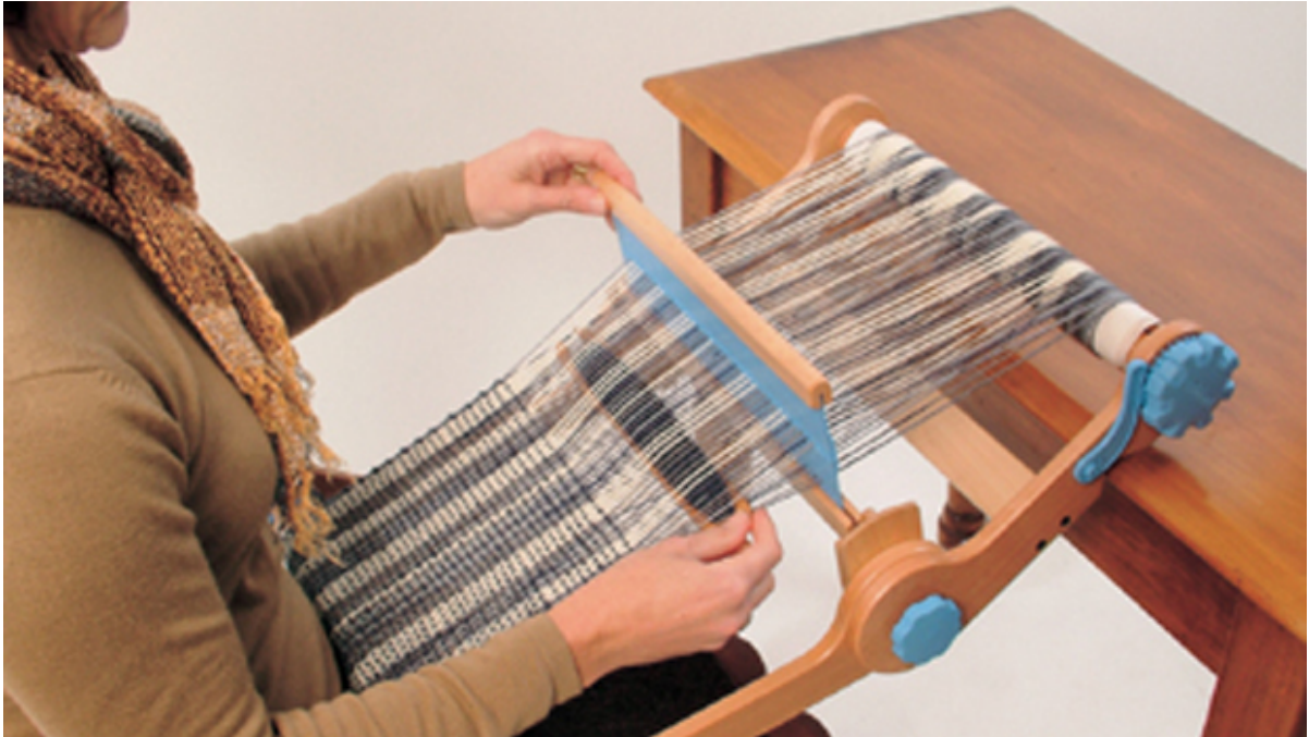
The back of the loom rests on a table while the front rests in your lap. This small loom is very versatile and can handle various weights of warp and weft materials.
