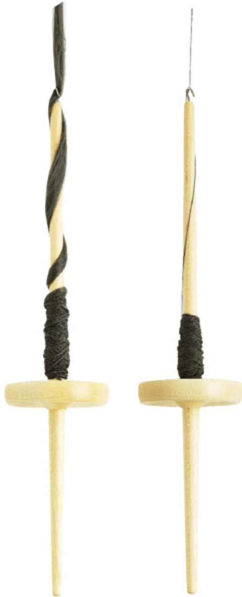
Thick yarn reaches its capacity for holding twist sooner and pushes back against the spindle's rotation harder than thin yarn.
