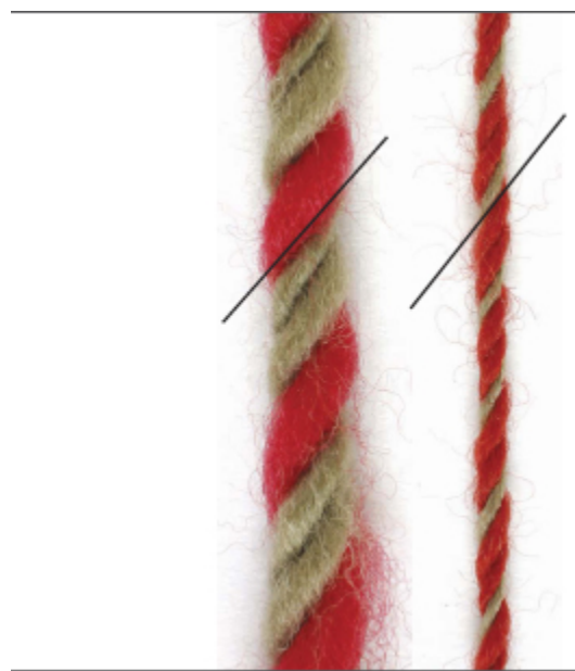
Right: Very bulky 3-ply, 1.6 tpi. Far Right: Sportweight 3-ply, 4 tpi. Both have about a 40° angle of twist.
