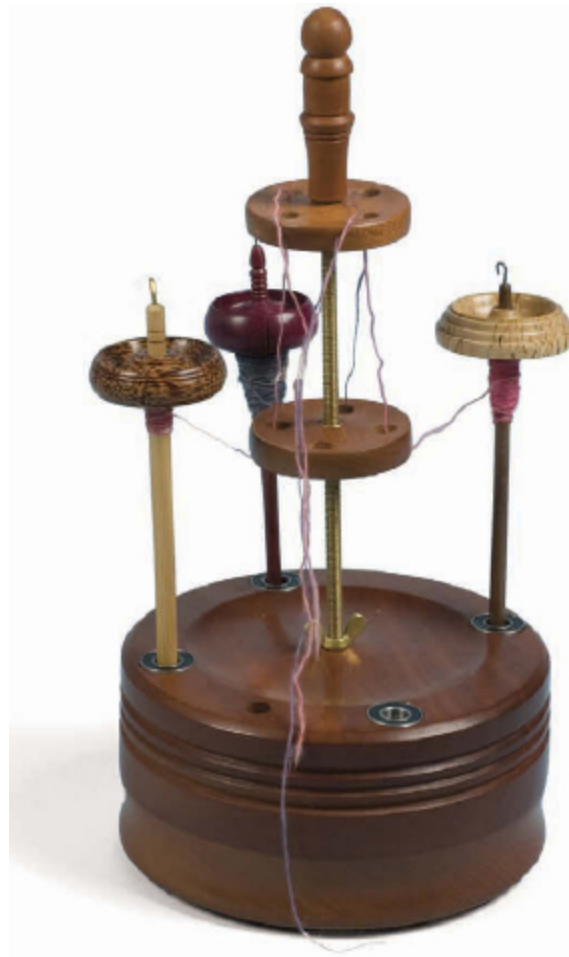
A specially designed spindle kate holds spindles in place and helps keep yarn under tension for plying.
