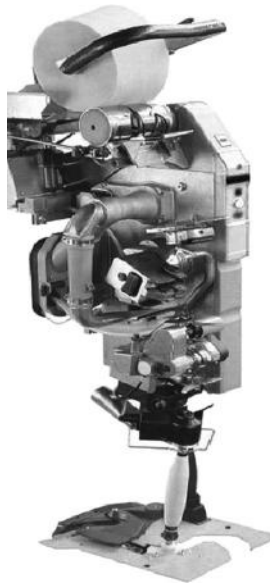
FIGURE 3.19 Cone winder with bobbin supplied by conveyor belt, Savio machine manual.
