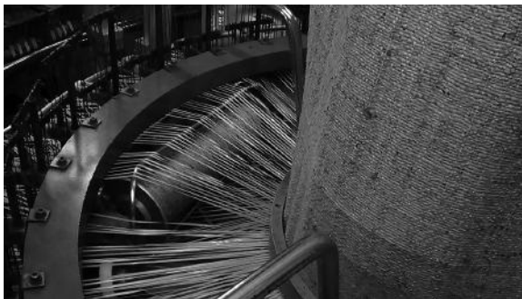
FIGURE 11.3 Tubular package within warp shed on a circular loom.
