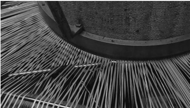
FIGURE 11.7 Beating up by a spur on a circular loom.
