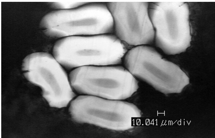
10.11 Dumbbell shape skin/core structure of PVA fiber.
