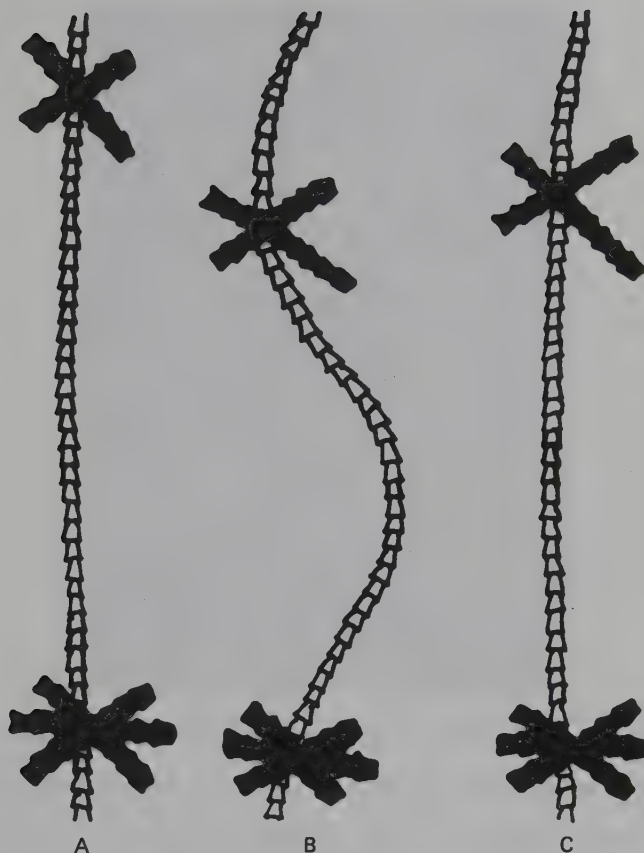
Figure 11. Schematic representation of fiber migration in a wool fabric which leads to felting shrinkage. A fiber is firmly entangled (A) with other fibers at its lower end but only partly entangled at its upper end. When the fabric is compressed during washing (B), the two ends of the fiber are brought together and it is temporarily bent. The scales are oriented so that the fiber can straighten elastically by sliding through the upper entanglement (C). The fibers in the two entanglements are now drawn closer together permanently because the scales permit fiber movement in one direction only. The fabric has shrunk.
