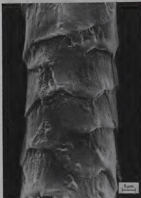
Figure 14. Electron micrograph of a merino wool fiber after treatment by the chlorine-Hercosett process, showing the polymer layer spread over the surface of the fiber.
