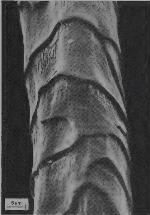
Figure 13. Electron micrograph of a merino wool fiber after treatment with chlorine, showing slight degradation of the scales.
