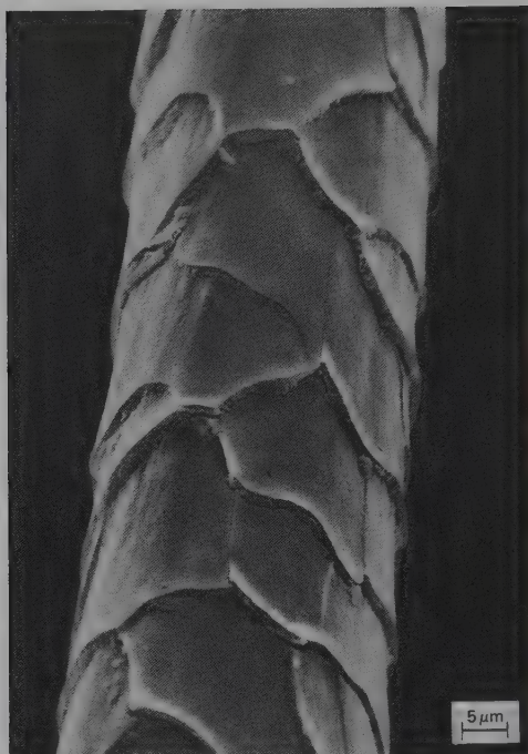
Figure 12. Electron micrograph of a merino wool fiber showing the scales on the surface.
