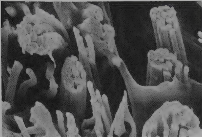
Figure 10. Impregnated suede (magnification 1000 \times ).
