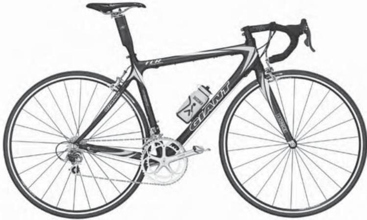
14.1 Lightweight race bicycle made of composite parts (courtesy: Giant, <http://www.giant-bicycles.com>)
