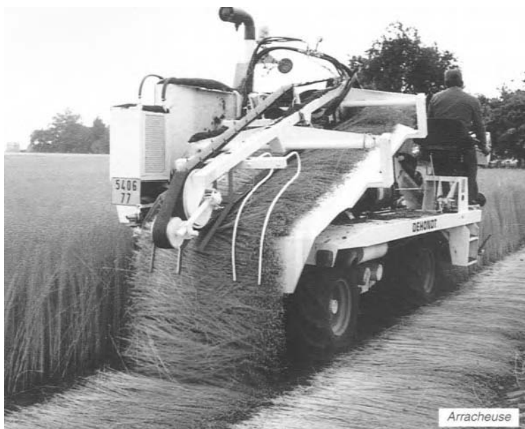
Figure 3.13 Flax puller in action. Source: Dehondt Technologies promotional literature. Courtesy: Guy Dehondt.
