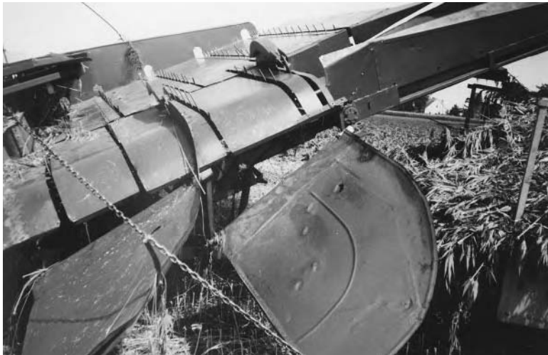
Figure 5.2 Mechanical harvester for bast fibres developed by the Institute of Natural Fibres, Poznan, Poland.
