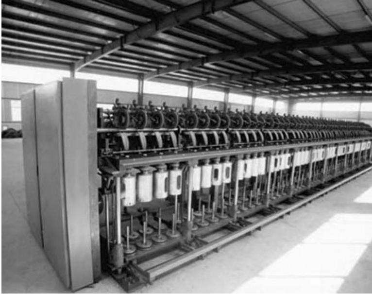
Figure 6.23 Vertical ring frame for sisal spinning.
