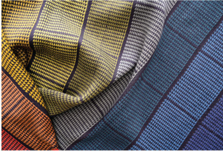
Figure 95 Weft-faced rep in rotation, 2/2 twill, 4 shafts. Fonty BB Merinos, 1,985 yd/lb (4,000 m/kg)
