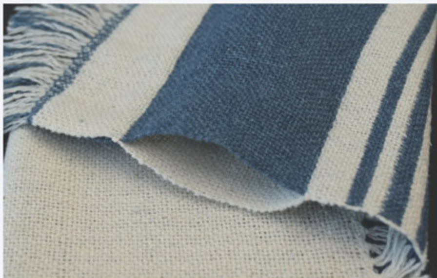
Figure 79 Sample of doubleweave, 4 shafts. Holstgarn Tides wool and silk, 2,828 yd/lb (5,700 m/kg)
