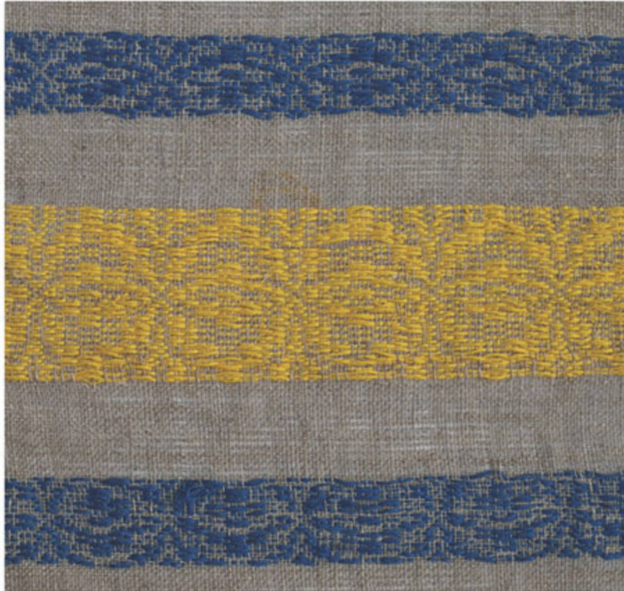
Figure 10 Overshot floats in 266 Royal Linen 24/6 100% MERO pure fine linen placed on a linen plain weave
