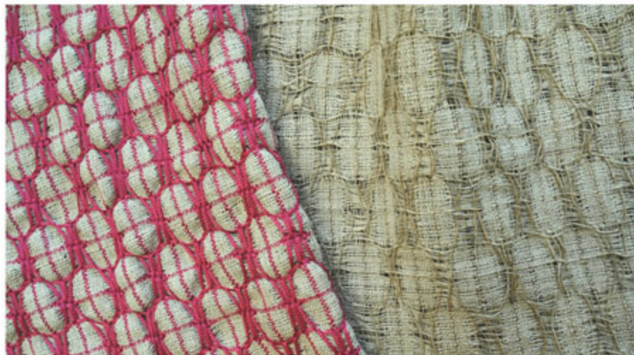
Figure 59 Honeycomb, 8 shafts. FIR Group Linen and Nepal nettle yarn or lacing.
