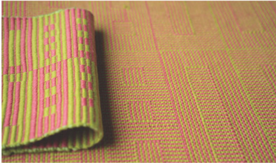
Figure 48 Plain weave and reps on 6 shafts—only the density changes
