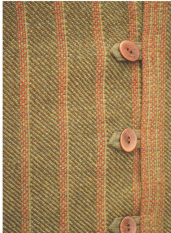
Figure 61 Vest made in 2/2 twill, straight twill threading, 4 shafts, Holstgarn Tides, 2,852 yd/lb (5,750 m/kg)
