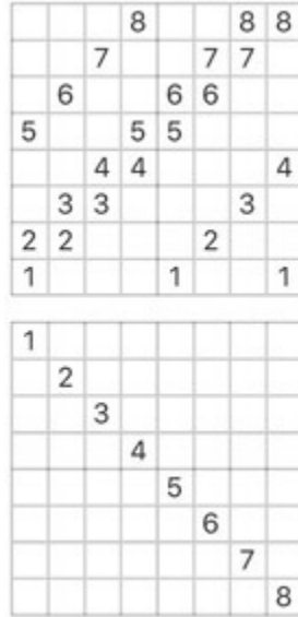
Figure 4 Simplification for reading the tie-up of a 2/2/1/3 twill
