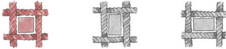
Figure 9 Square thread count in plain weave vs. rectangular distortion
