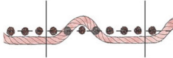
Figure 127 Number of interlacings in a 5-shaft satin
