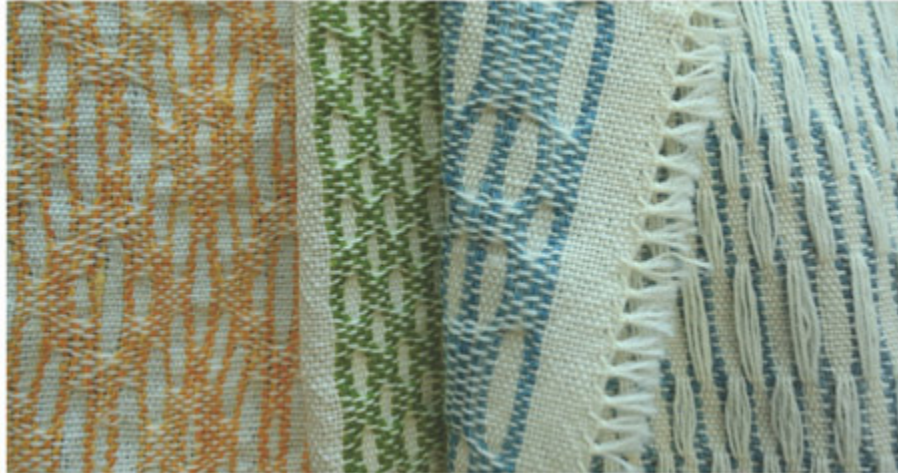
Figure 61 Honeycomb, 8 shafts. Fonty Zephir 17/2 wool
