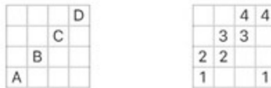
Figure 23 Tie-up for an overshot in profile draft and its expanded draft
