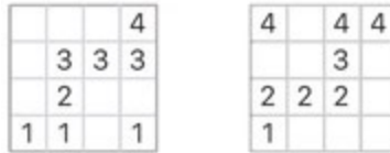
Figure 83 Tie-up on 4 shafts: light plain weave or dark plain weave visible on top
