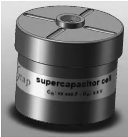
Figure 10.31 Batscap cell design with direct laser welding between cover and can.
