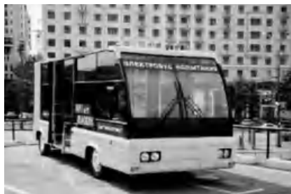
Figure 14.6 All-electric bus powered by ESMA asymmetric electrochemical capacitors.
