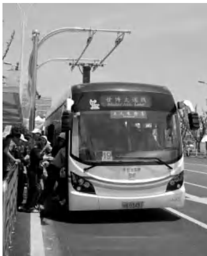
Figure 14.7 Capacitor-powered bus in Shanghai.
