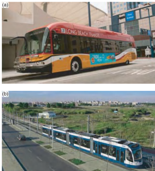
Figure 5.21 (a) A rideHybride gasoline/electric bus in Long Beach, California. The use of capacitors, located on the roof, improves the emissions and offers almost the same fuel efficiency as diesel fuel even for the less fuel efficient gasoline engine. Courtesy of Brynn Kernaghan and Juan Vigil of Long Beach Transit. (b) A tram without
