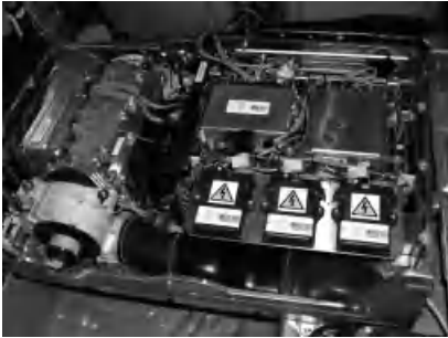
Figure 8.6 Schematic view of the UltraBattery and UltraBattery cycling versus NiMH under the EUCAR power-assist profile, the UltraBattery in place and changes in the discharge voltages
