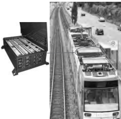
Figure 14.14 Onboard electrochemical capacitor storage system for a light-rail system.
