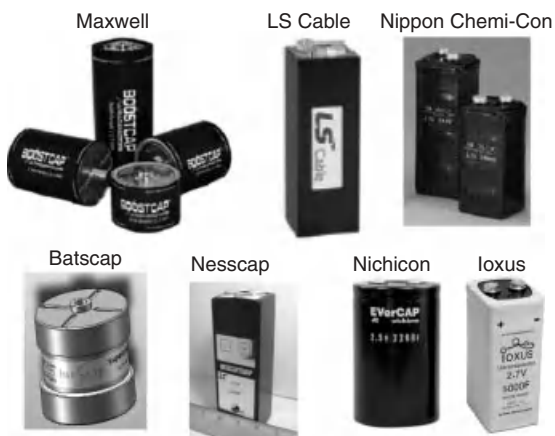
Figure 14.4 Electrochemical capacitor cells, each using an organic electrolyte. Voltage ratings are 2.5 or 2.7 V, depending on the manufacturer. Cells are connected in series to provide higher working voltage.
