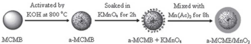
Fig. 3.63. Schematic diagram demonstrating the growth process of the nano-MnO 2 onto the a-MCMB particles. Reproduced with permission from [193], Copyright © 2010, Elsevier.
