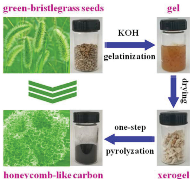
FIGURE 7.7 Flow diagram of the synthesis of 3D interconnected honeycomb-like porous carbon materials derived from green bristlegrass seeds. (Reprinted with permission from Zhou, W. et al., J. Power Sources , 402, 203–212, 2018.)
