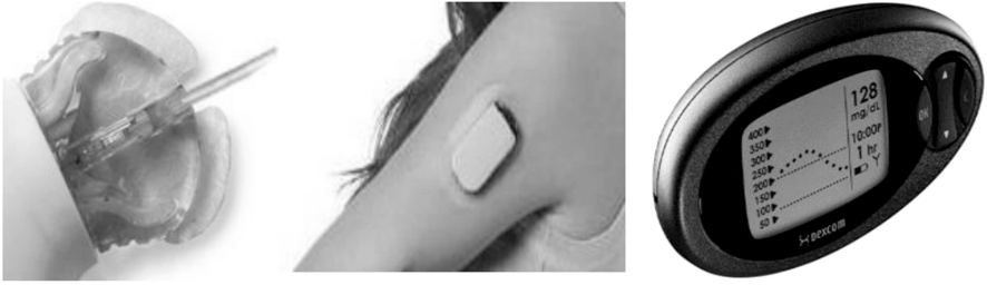
FIGURE 7.3 Continuous glucose monitoring (CGM) sensor, receiver and transmitter.
