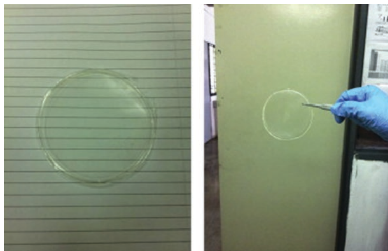
Figure 22.4 Transparent and free-standing starch-chitosan-based film. Reproduced with permission [49]. Copyright 2015, Elsevier.
