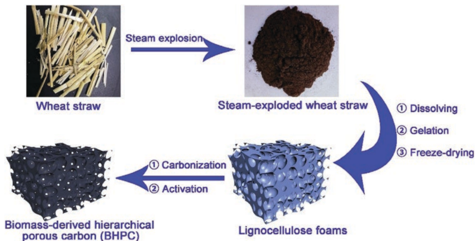
Figure 11.3 Synthesis of biomass-derived hierarchically porous carbon materials. Reproduced with permission [93]. Copyright 2020, Elsevier.
