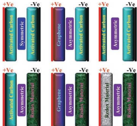
Figure 6.4 Schematic representation for the symmetric and asymmetric configuration of supercapacitors.
