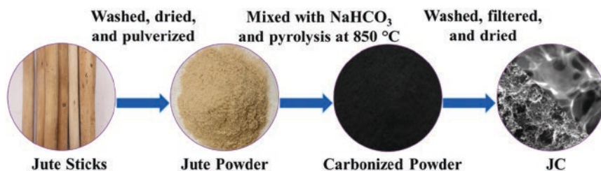
Figure 9.4 Schematic representation for synthesizing AC from jute sticks using \text{NaHCO}_3 as an activation agent. Reproduced with permission [5]. Copyright 2021, Elsevier.
