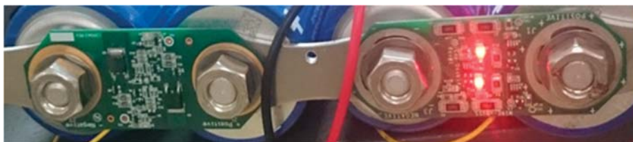
Figure 10. Four SCs connected in series with the active balance board in “standby mode” (left one) and in “on mode” (right one).
