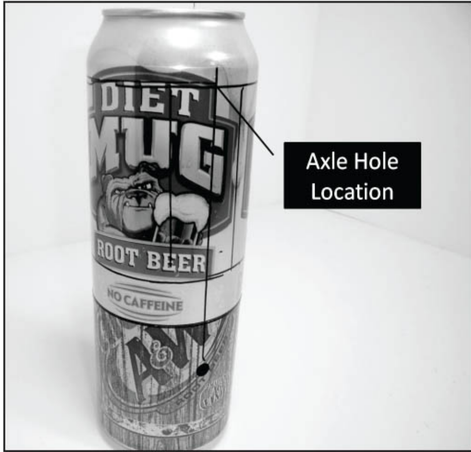
Figure 24 - Punch a hole for the axle (crankshaft) on both sides of the engine at the point where the centerline crosses the top line. The hole should be the same size as the crankshaft material.
