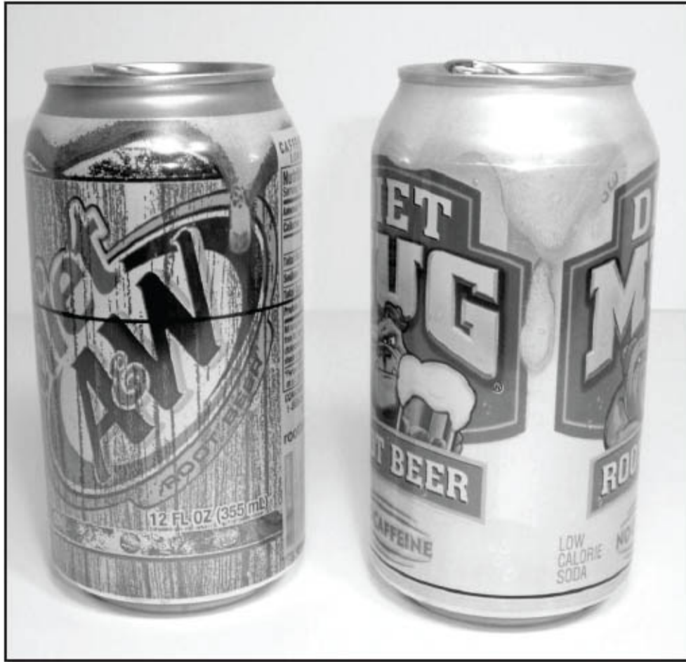
Figure 11 - The bottom can (left) is marked at 2 1/2" (64 mm) from the bottom. The top can (right) is marked 1/8" (3 mm) from the bottom edge. The brand of beverage is not important, but both cans must be the same size.
