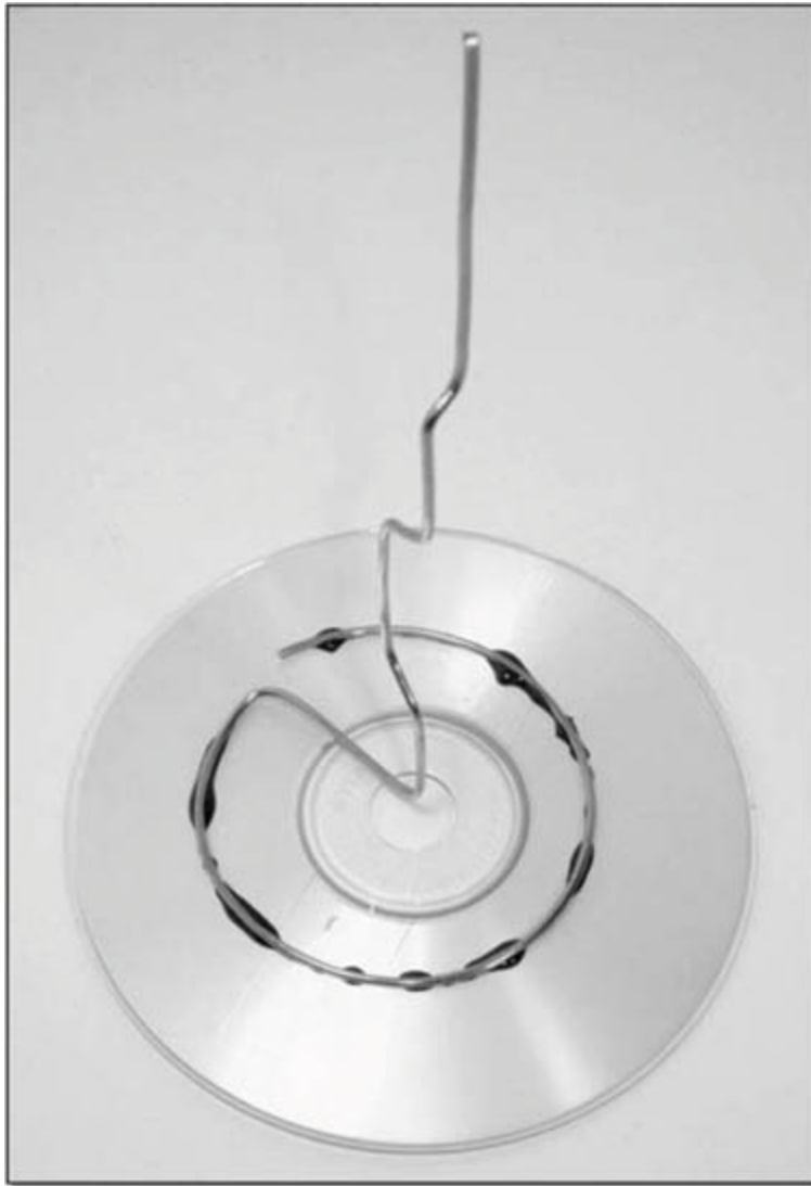
Figure 33 - This is the crankshaft with the flywheel attached. Note how the loop is formed in the end of the wire to attach the flywheel.
