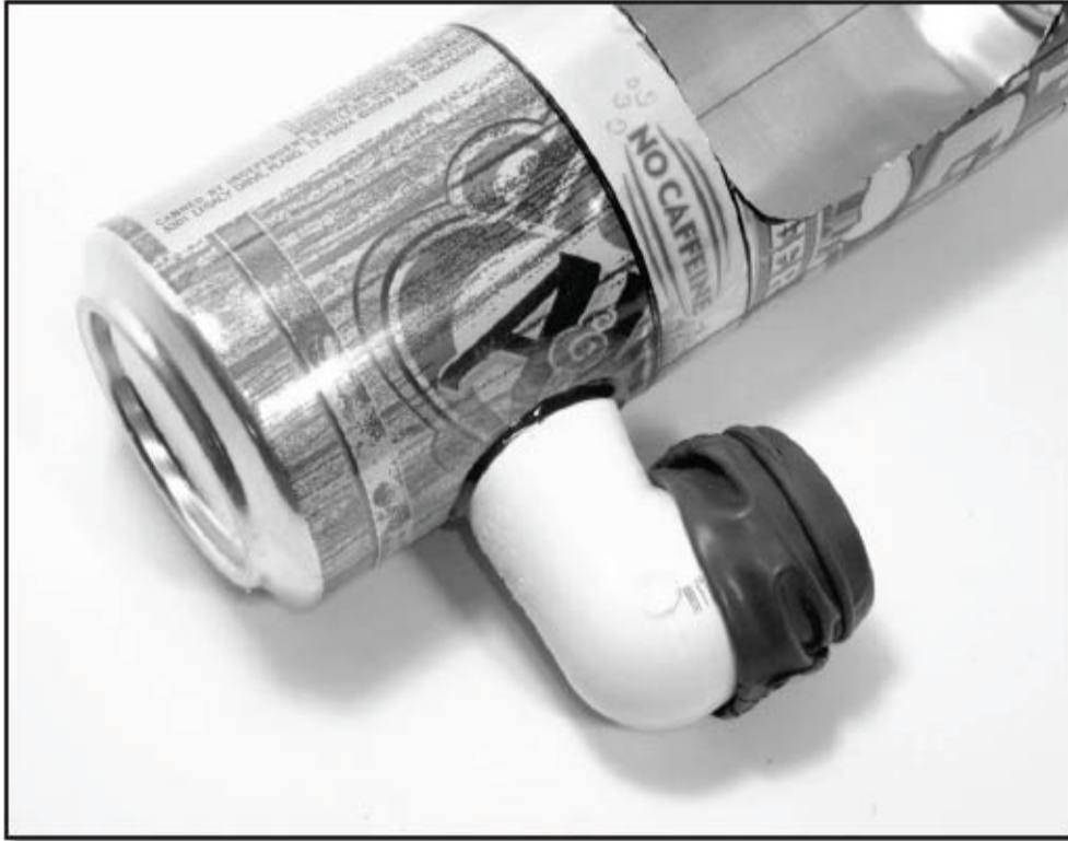
Figure 28 - The pipe elbow has been glued in place over the hole in the pressure chamber. Use sandpaper to roughen the side of the can prior to gluing.
