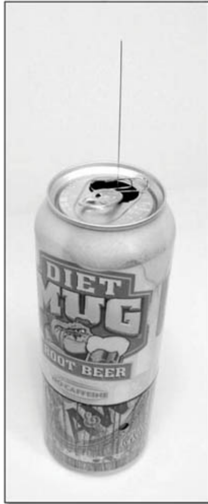
Figure 20 - The top can is pressed down into the pressure chamber bottom until the line on the top can is lined up with the seam.
