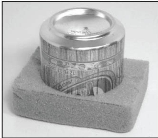
Figure 15 - Use the pressure chamber bottom like a cookie cutter to create the displacer disk.
