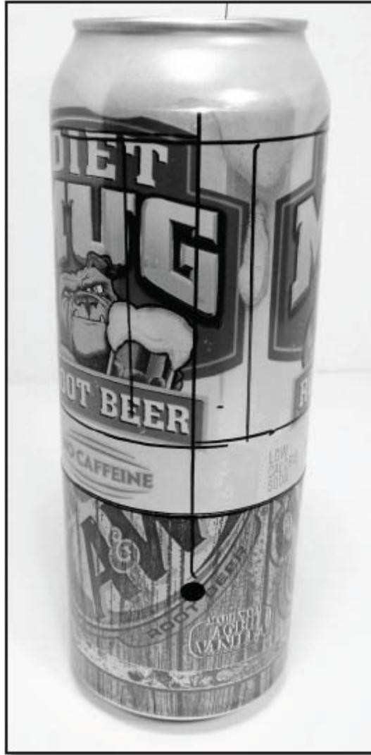
Figure 22 - Draw a centerline up from the hole. Draw parallel lines 1/2" (13 mm) from the center line. Draw a line 3/4" (19 mm) above the seam and 1/8" (3 mm) below the top edge. Repeat the pattern on the opposite side of the can.
