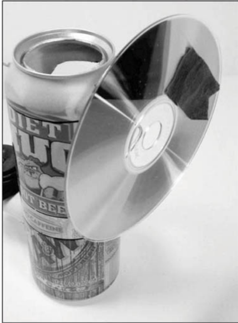
Figure 35 - A small coin is taped to the flywheel to provide balance.
