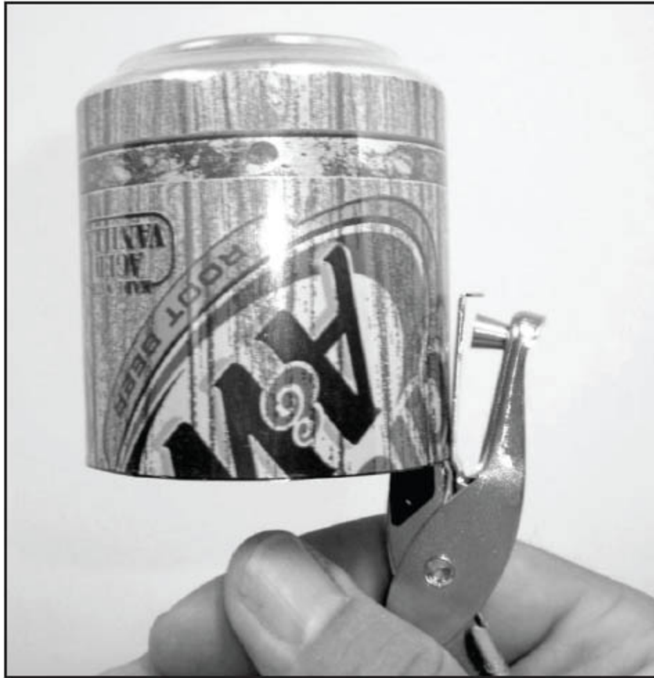
Figure 18 - Use a paper punch or a sharp cutting tool to make a hole in the side of the pressure chamber. The drive cylinder will attach here.
