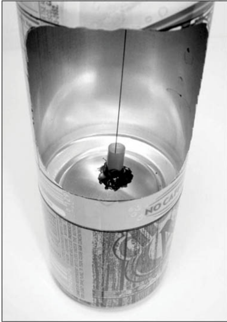
Figure 26 - Glue the drinking straw in place around the pinhole and music wire. Be very careful that you do not get any glue on the music wire or the pinhole.
