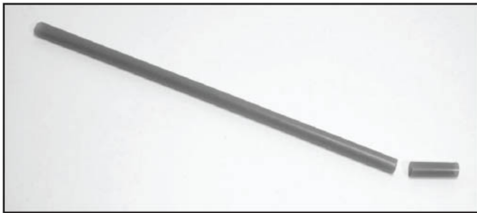
Figure 25 - Cut a 3/4" piece from the end of a large diameter drinking straw.
