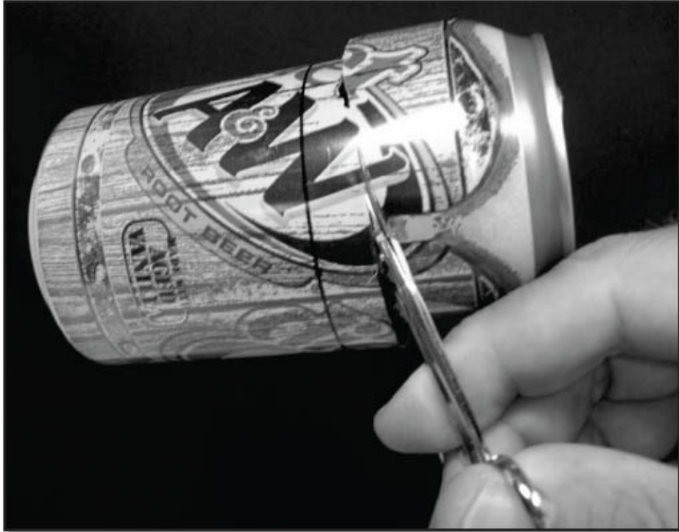
Figure 12 - Make the initial rough cut about 1/4" (6 mm) above the line.
