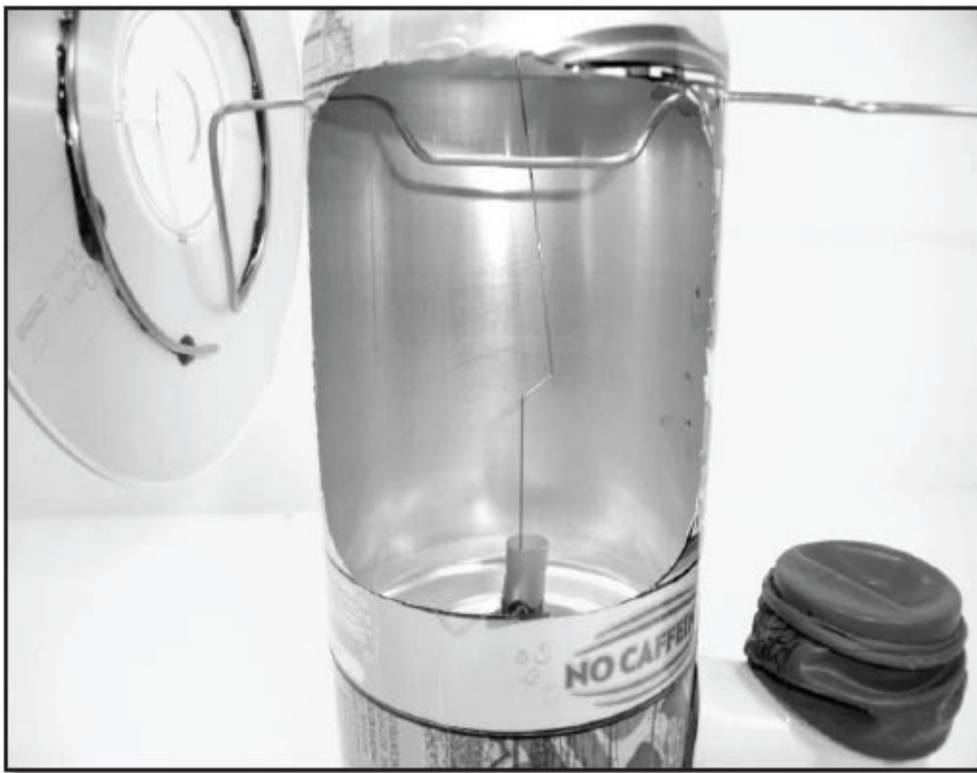
Figure 34 - There is a Z-shaped bend in the displacer pushrod. This makes it possible to adjust the length of the pushrod after it is attached to the crankshaft. Attach it to the crankshaft with at least one half turn around the shaft.
