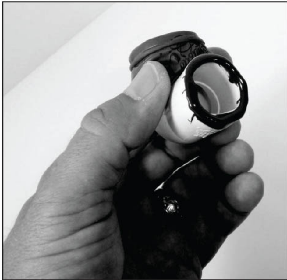
Figure 27 - Apply J-B Kwik ® epoxy to the small shaped end of the PVC pipe elbow and glue it over the hole in the side of the pressure chamber.
