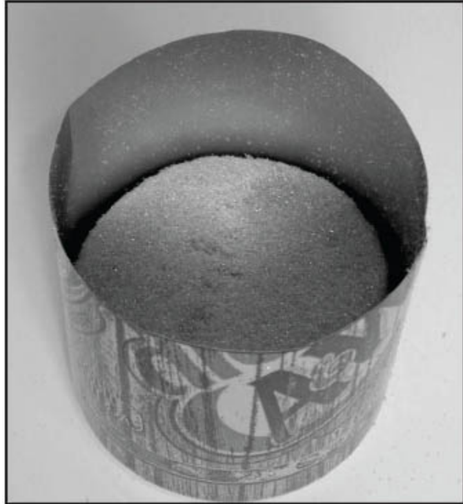
Figure 16 - The displacer disk is reduced in size until it will fall into the soda can under its own weight.
