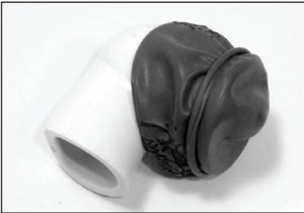
Figure 10 - Use the rubber band made from the balloon neck to hold the diaphragm in place.
