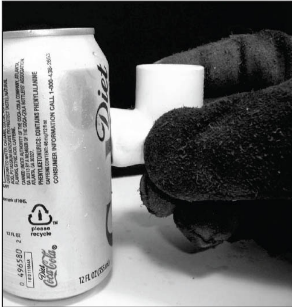
Figure 7 - Press the heated end against an unopened soda can and hold it until the fitting cools. The PVC fitting will take on the contour of the outside of the can.
