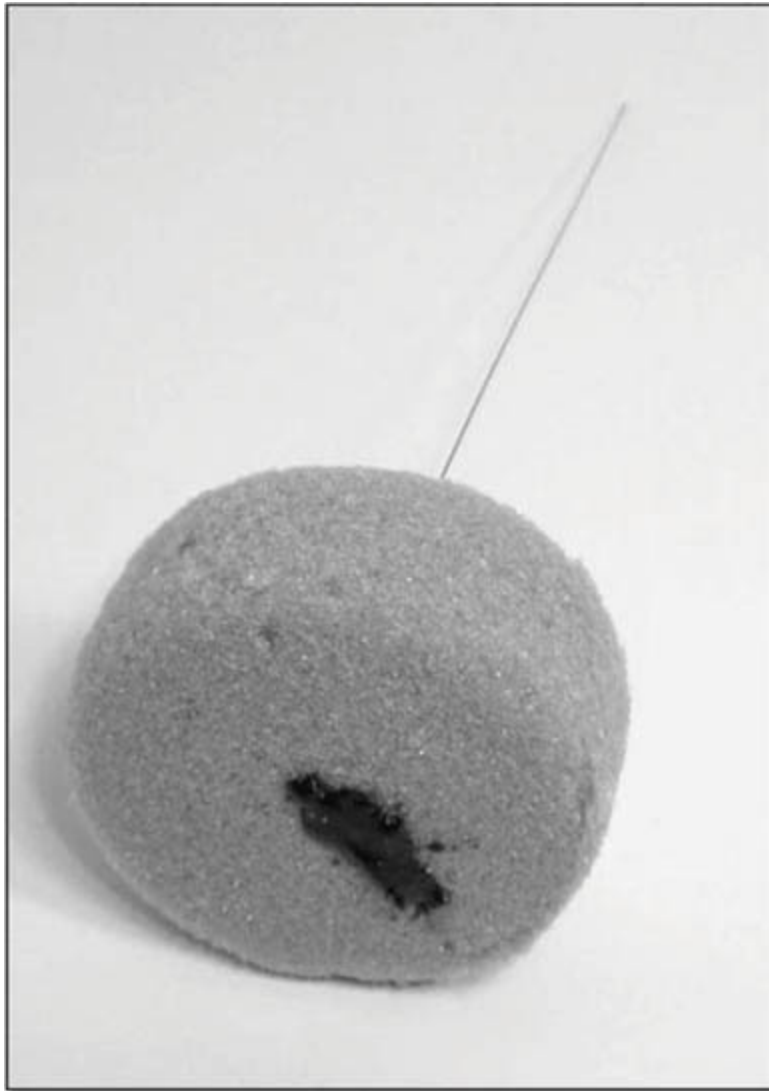
Figure 17 - The music wire is passed through the foam disk and glued with J-B Kwik ® epoxy.
