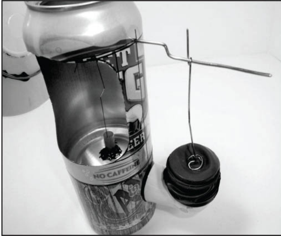
Figure 37 - The pushrod is attached to the balloon with Super Glue. There is a Z-shaped bend in the middle of the rod for adjusting the length (It is difficult to see at this angle). It is attached to the crankshaft with a single wrap around the shaft.
