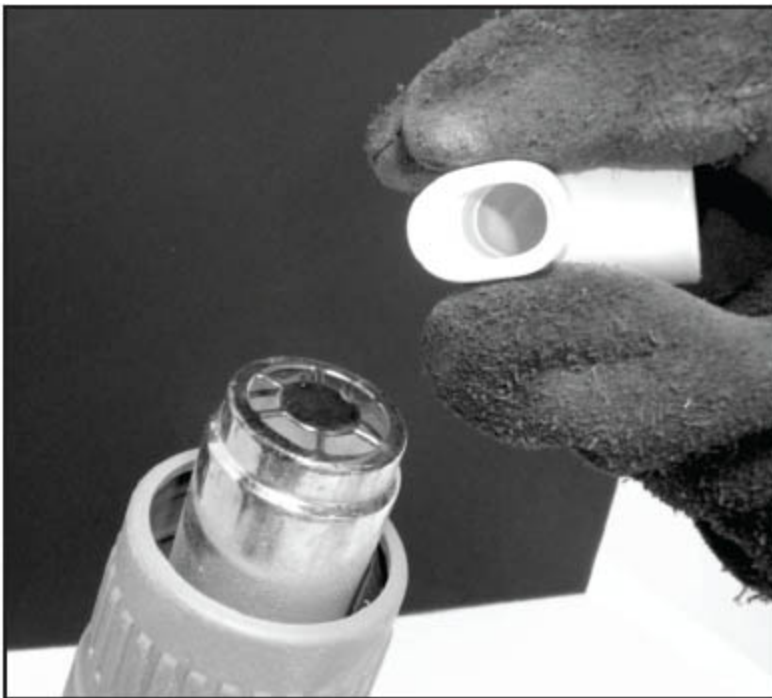
Figure 6 - Heat the small end until it becomes soft. You can tell when it is getting soft as it will deform easily when pressure is applied, as you can see here.
