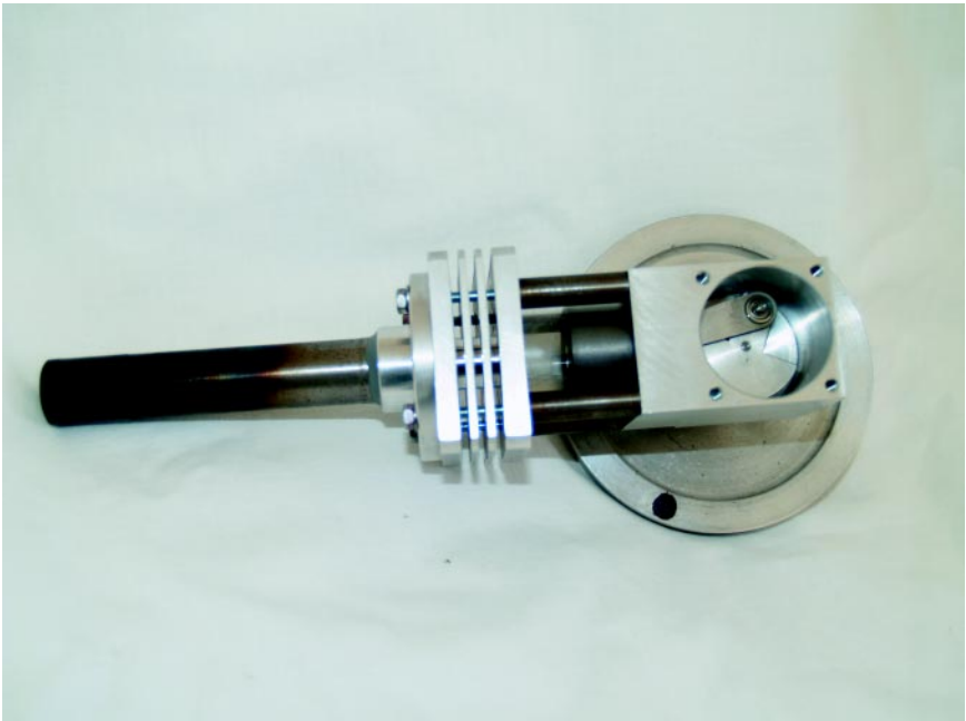
Plate 3 'Thermal lag' engine of 20cc displacement. Machining work by Ian Larque.
