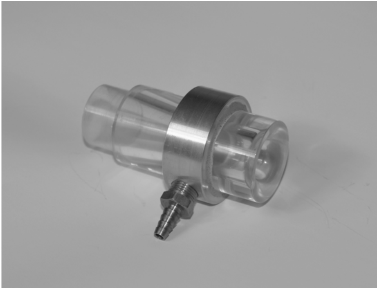
4.5 Siting the venturi-meter at the pre-heater inlet means it operates at ambient temperature, and can be made from a readily-machined material such as acrylic.
