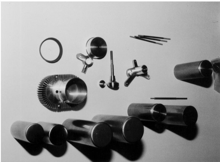
7.12 Selected components of small rotating-displacer engine. The concept was under exploration for possible addition to a portfolio of teaching projects under the 'guided mechanical design' heading. It was eventually judged too demanding for the timetable hours allocated.
