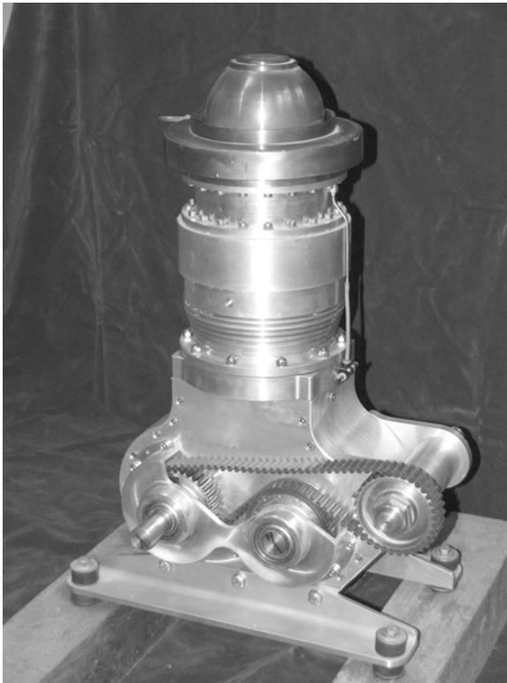
16.1 Rhombic drive engine, synchronized by external double-sided timing belt. With permission of G. Vaisey.
