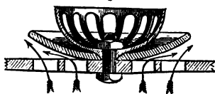
MAUDSLAY'S DISC VALVE FOR AIR PUMP. Section.
