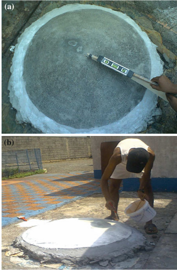
Fig. 4.9 Fibreglass layout. a Paraboloid after application of silicone paste. b Fibreglass being laid
