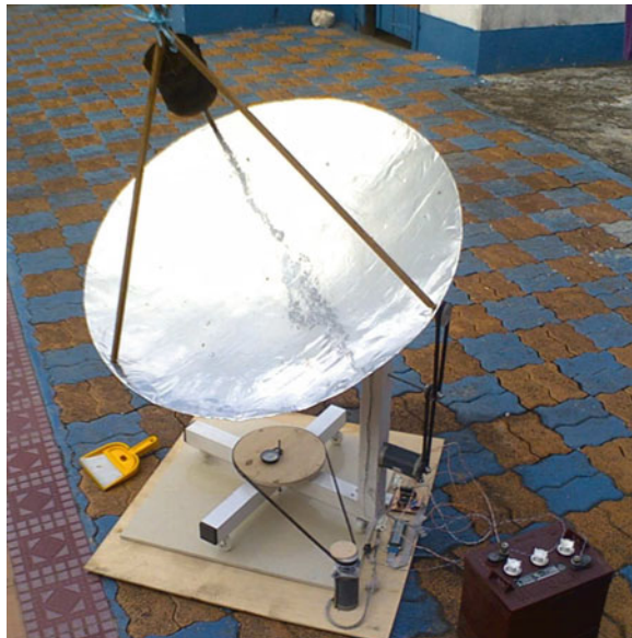
Fig. 5.3 Diagram showing a blackened can affixed to the concentrating dish using a tripod
