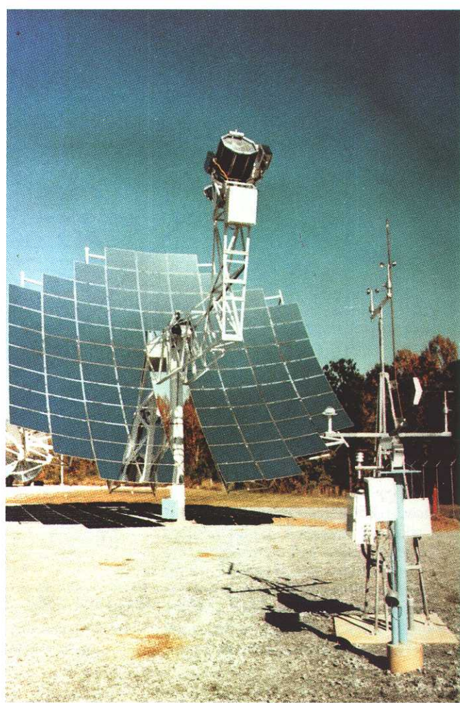
Figure 3-30. Faceted dish collector design by MDAC (Source: MDAC)
