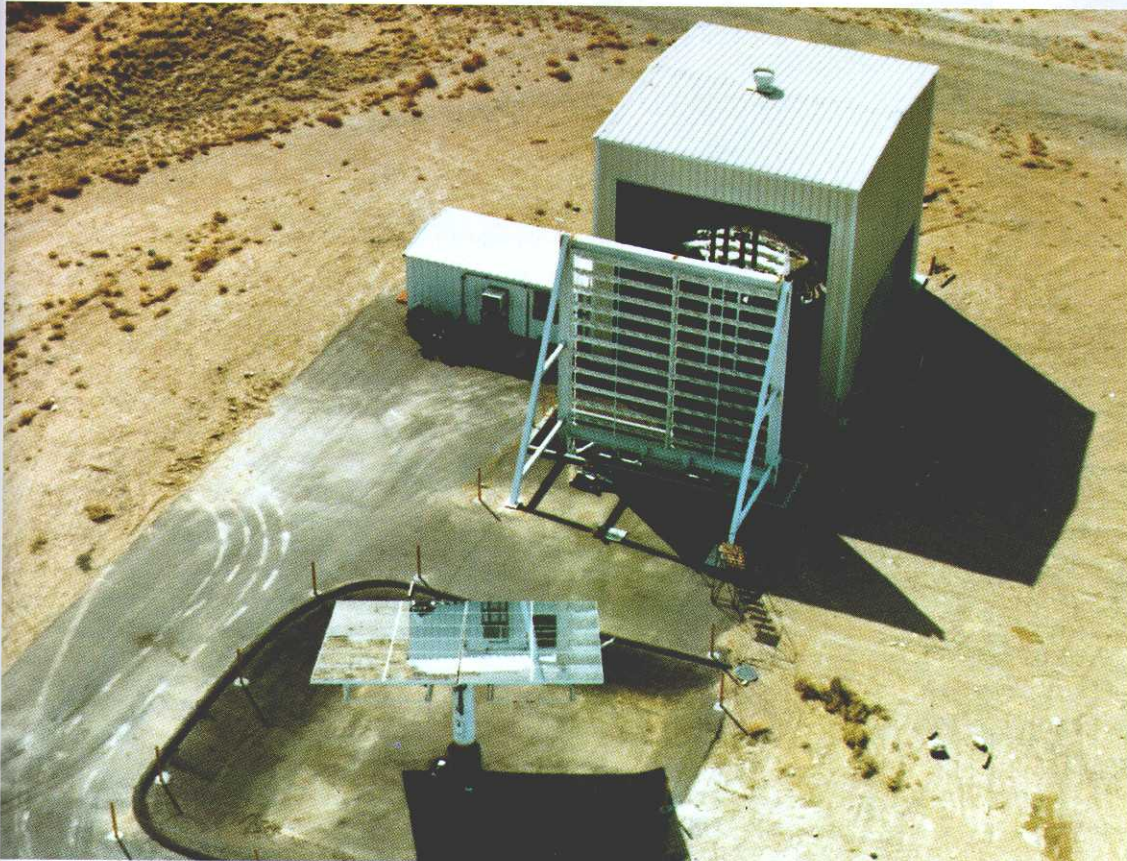
Figure 5-3. The 16-kW solar furnace at SNL in Albuquerque, New Mexico, USA (Source: SNL)
