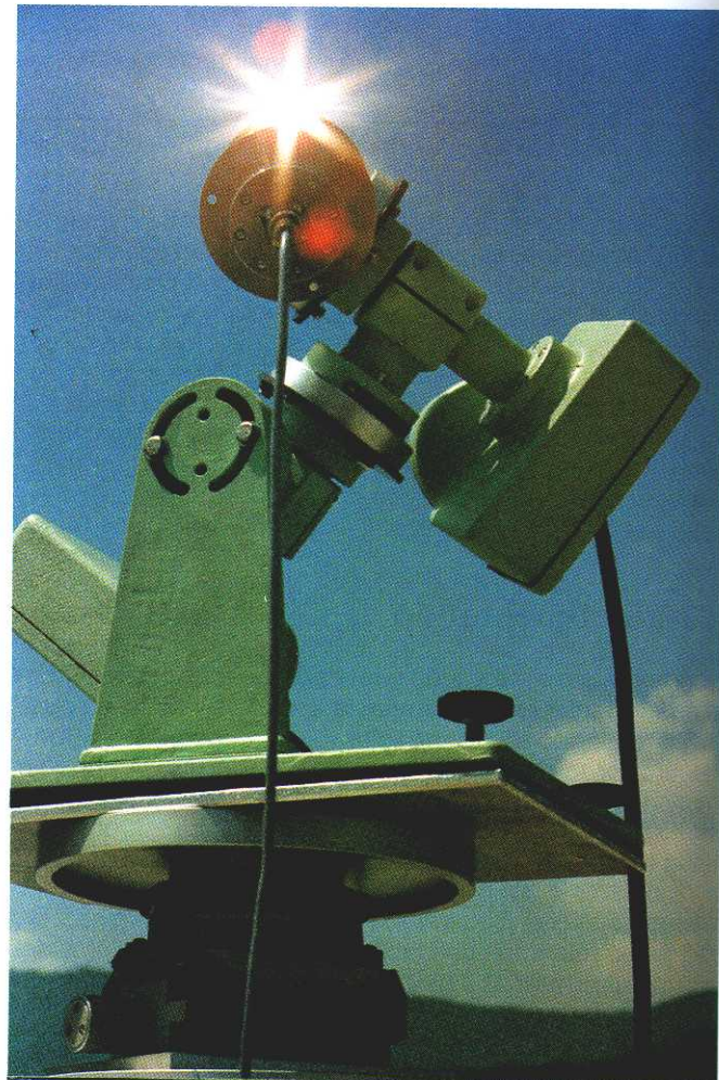
Figure 4-6 Pyrheliometer mounted on solar trackers (Source: PSI)
