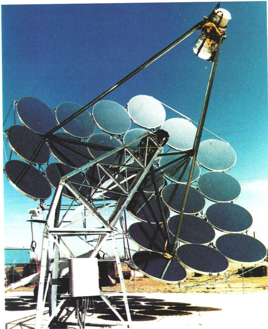
Figure 3-29. Concentrator structure of the 5-kW e Cummins dish/Stirling prototype system 460B (Source: CPG and SNL)
