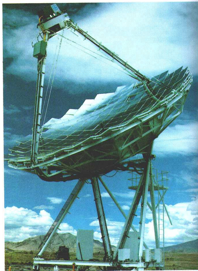
Figure 5-2. The 75-kW test bed concentrator (TBC) with sodium pool boiler refluxing receiver at SNL in Albuquerque, New Mexico, USA (Source: SNL)
