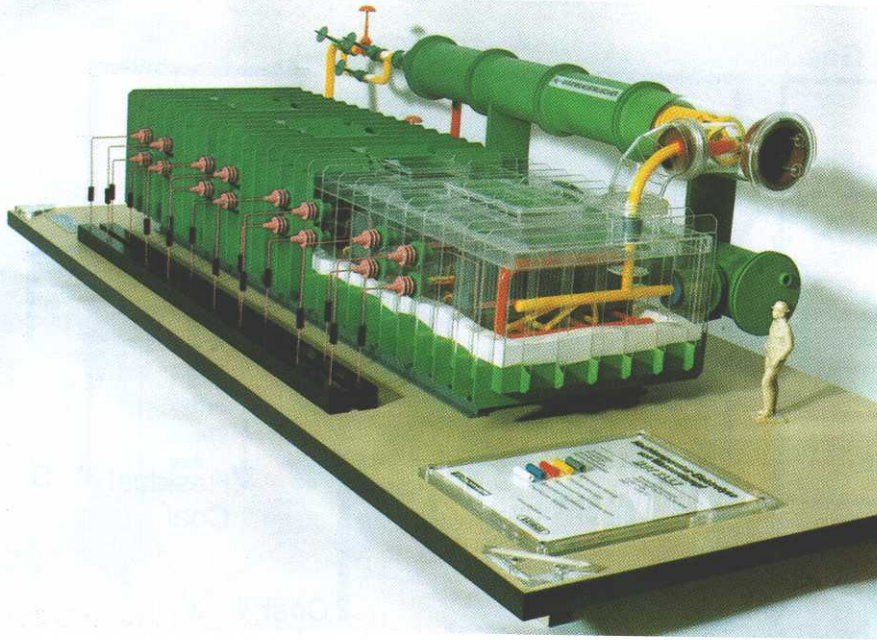
Figure 2-53. Model of the high-temperature steam electrolyzer for hydrogen production, HOT ELLY (Source: Lurgi/Dornier)
