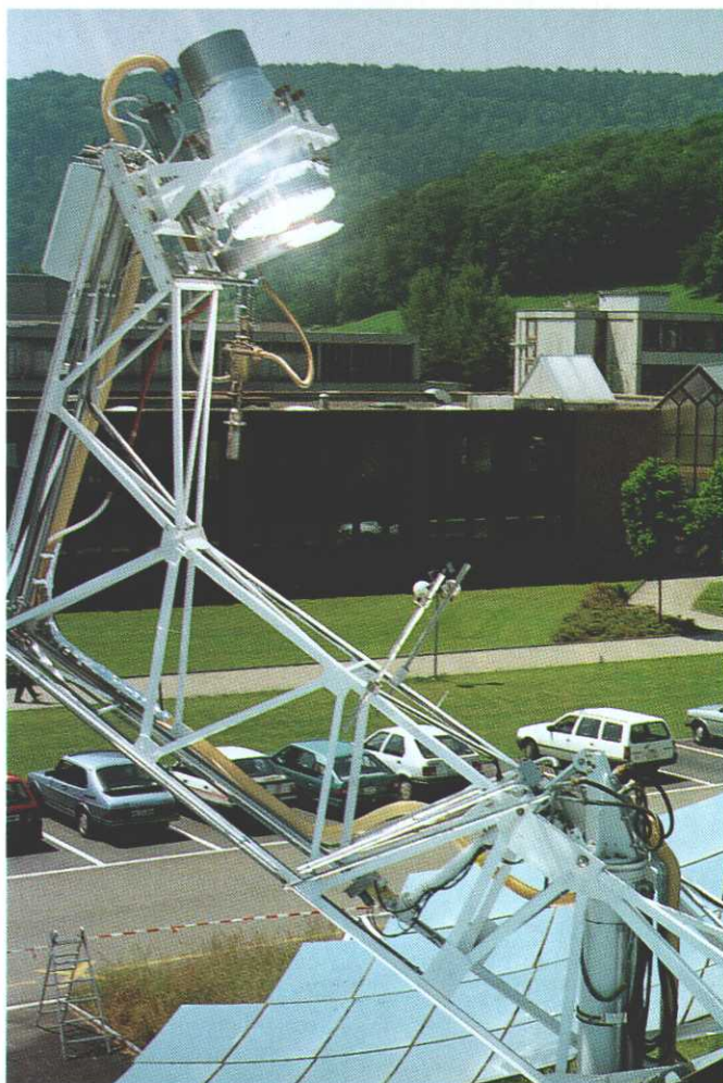
Figure 2-57. Testing the atmospheric open solar cyclone reactor on the 60-kW parabolic test bed concentrator of PSI for decarbonation of limestone (Source: PSI)
