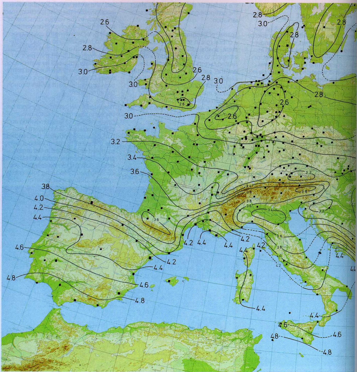
Figure 4-2. The distribution of annual averages of daily global solar ra- diation data across Europe during 1966-1975; contours are labelled in units of kWh/m 2 per day (Source: EU, Brussels)
