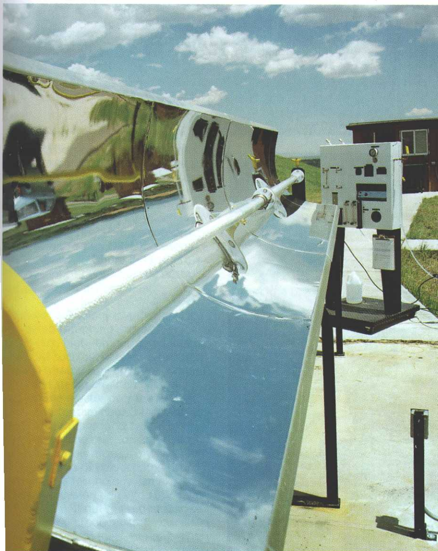
Figure 2-34. Parabolic trough used for detoxifica- tion of water conta- minated with trichlorethylene (Source: NREL)
