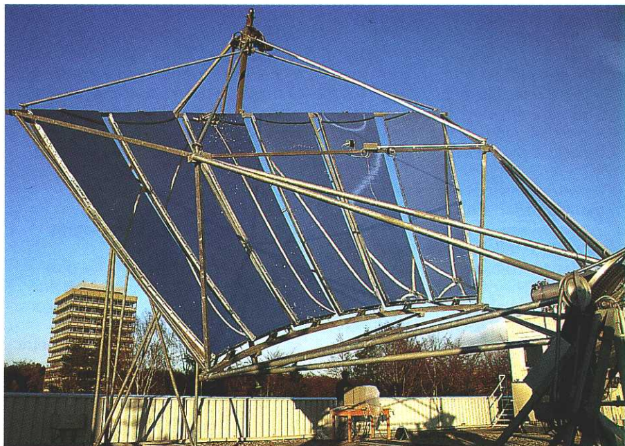
Figure 3-31. Fix-focus dish concentrator/structure (Source: HTC-Solar)
