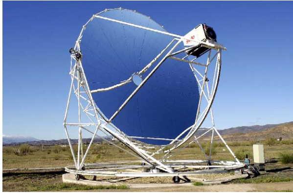
FIGURE 11 Paraboloidal dish solar concentrator with a receiver-mounted Stirling engine operating in southern Spain. Source: Schlaich, Bergermann, and Partner.
