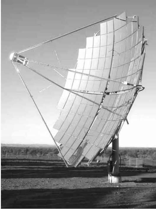
10.8 Example of a point focus imaging paraboloidal concentrator from Solar Systems, Australia.
