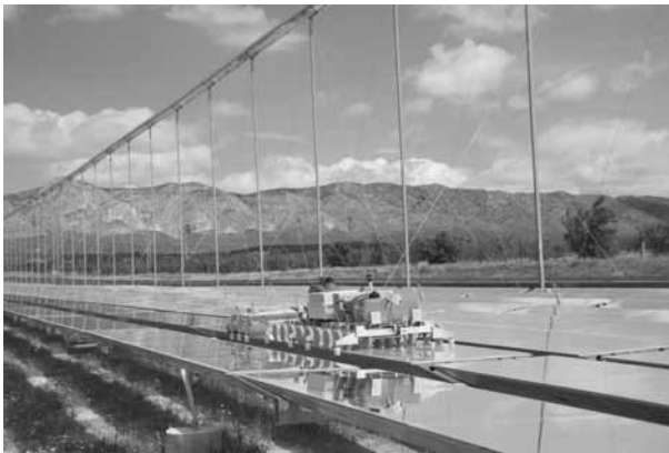
6.25 Illustration of Novatec dry cleaning robots moving down a reflector line (courtesy Novatec Solar GmbH).
