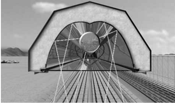
6.28 Cross-sectional sketch of the Novatec receiver and secondary reflector (courtesy Novatec Solar GmbH).
