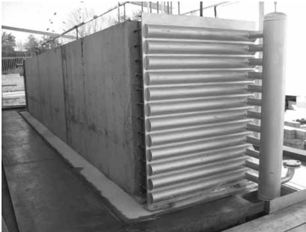
11.10 Concrete storage module (400 kWh th ) connected to test rig, before installation of insulation.
