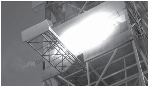
20.16 (a) Partitioning of the SSPS-CRS heliostat field at the PSA (Roeb et al. , 2011); (b) focus of solar radiation on the dual HYDROSOL-II reactor (Konstandopoulos and Lorentzou, 2010).
