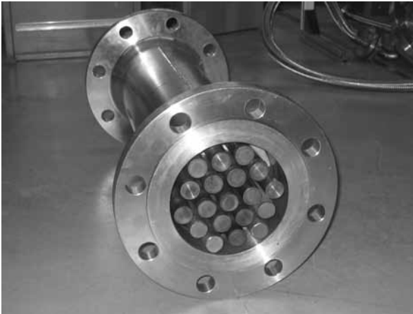
11.15 Pipe segment with containers filled with PCM (macro-encapsulation).
