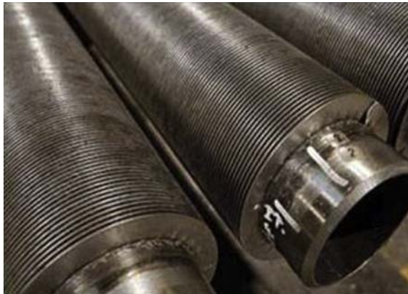
Figure 9.6 Finned tube heat exchanger. Gatton Tower, Gatton campus of the University of Queensland.
