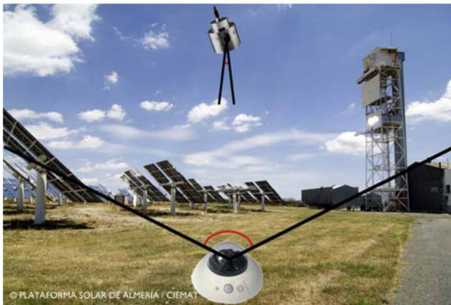
Figure 13.3 Comparison of satellite view (facing the earth surface) and sky camera (facing the sky). Supported angles at a given location are also different. Satellite pixel is typically contained in 2 degrees from satellite position; sky camera has about 2\pi stereo-radians view.
