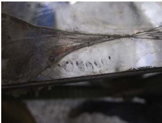
Figure 2.6 Mirror cracks appeared during the testing of the REFOS secondary concentrator, close to the edges.
