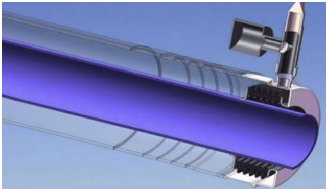
Figure 4.3 Re-evacuation system in Huiyin's receiver tube.
