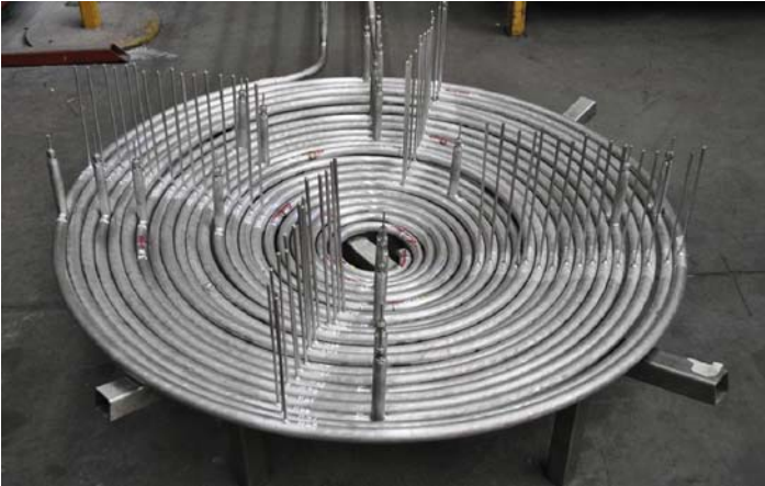
Figure 17.1 A picture of the CSIRO supercritical steam receiver [15].
