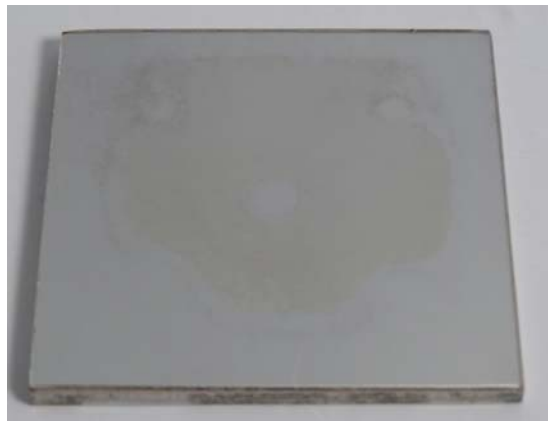
Figure 2.7 Picture of a silvered thin-glass reflector glued to an aluminum back sheet, after the damp heat test, where corrosion appeared due to a chemical reaction provoked by the glue under the test conditions. PSA.
