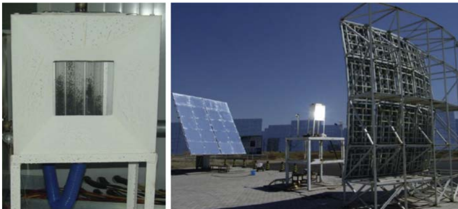
Figure 6.8 Images of testing of a quartz-tube particle air receiver [60].
