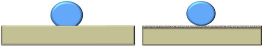
Figure 2.2 Schematic of a hydrophobic surface (left) and a super-hydrophobic surface (right).
