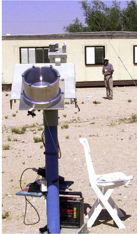
Figure 18.21 Optical system for the transmission of high-flux concentrated solar radiation. Reprinted from [200], Copyright with permission from Elsevier.
