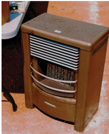
Fig. 5.5i. Gas flame heater used to heat older buildings.
