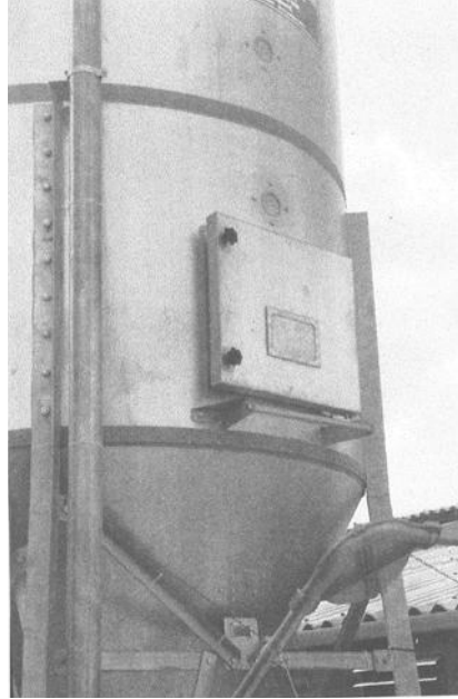
Praise be - a bin manufacturer who has seen the light. Side access door, simple swingaway exit boot and a succession of inspection windows. (Uttley Ingham Ltd photo)
