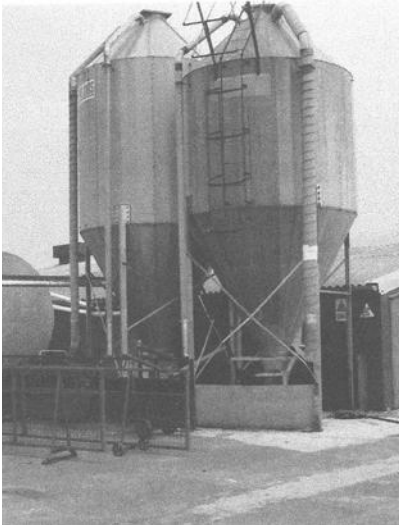
Typical bulk bins today with a tiny upper hatch and firmly bolted-on-draw-off boot. These are extremely difficult to clean properly (Author's photo)
