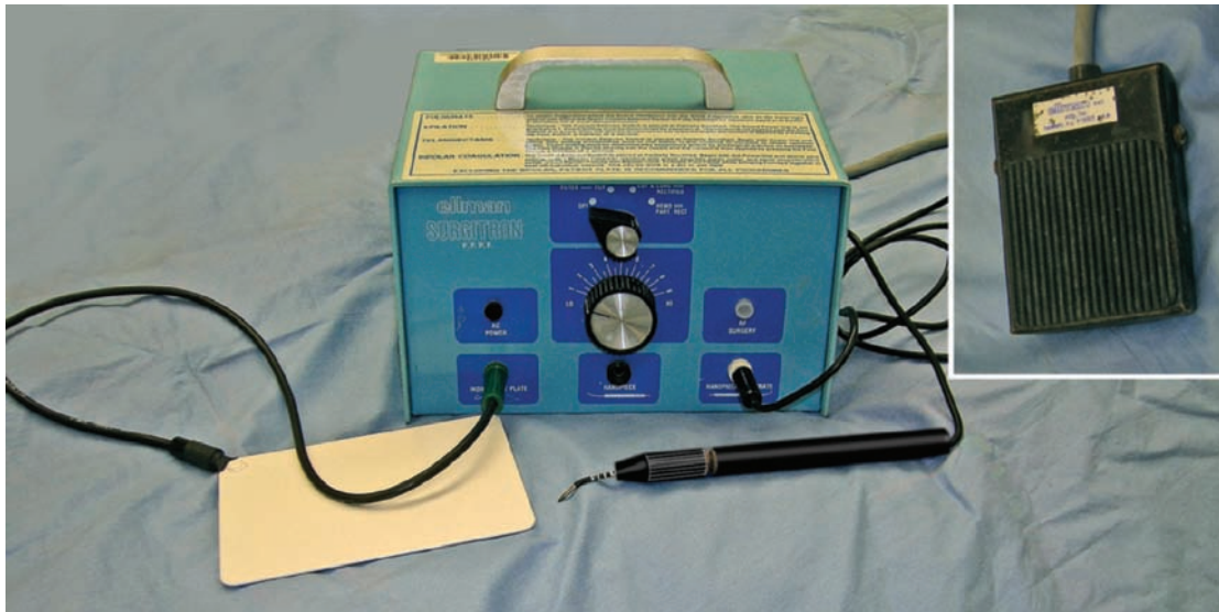
Figure 16.11 Radiosurgery unit. Multiple tip styles are available for the handle. A curved tip is demonstrated here. The handle is plugged into the white fulguration port in this photo, but would be plugged into the black center hand piece port for the more commonly used modes of cutting and coagulation. The white passive electrode is an antenna that receives the radio waves to complete the circuit running through the patient. The white plate is not a grounding terminal and does not need to be in direct contact with the skin. As such, there is no need for conductive gel. The white plate is not necessary for fulguration, but is necessary for cutting and coagulation. The current is activated by stepping on the foot switch (inset).
