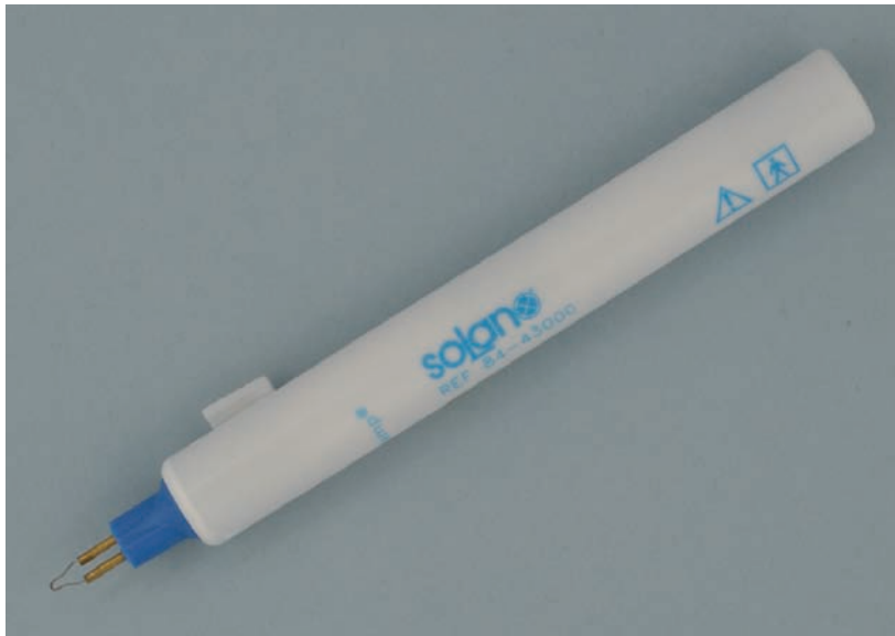
Figure 16.7 Electrocautery unit. An electrical current generated from a battery in the handle heats the metal filament. The heated metal is then applied directly to the bleeding source to burn (i.e., cauterize) the tissue to control bleeding.
