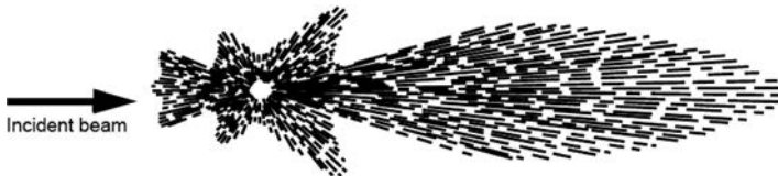
Figure A.7 Scattered light pattern for larger particles (larger than the wavelength of the incident light (Hach, 1985).
