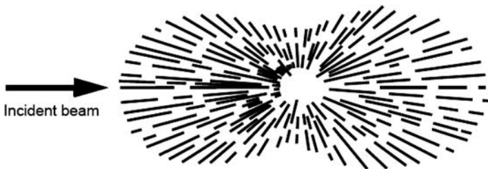
Figure A.5 Scattered light pattern for very small particles (smaller than 10% the wavelength of the incident light (Hach, 1985).
