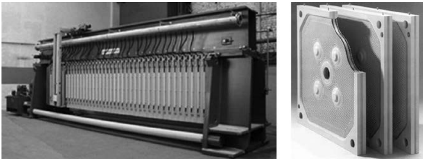
Figure B.25 Filter press (Courtesy Andritz Netzsch) and filter plates (Courtesy Menardi).
