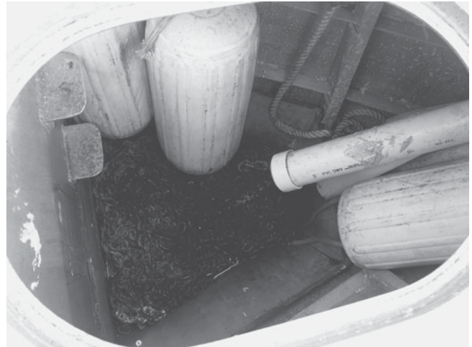
Figure 4-23. The PVC pipe could be led farther aft in Hawk's chain locker for better weight distribution; however, it is high enough that the chain never pyramids and jams under the pipe.
