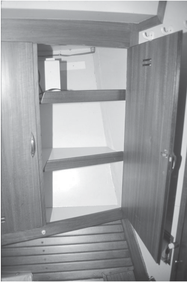
Figure 11-4. The contents will not stay in this locker if it is opened when the boat is heeled over or rolling.
