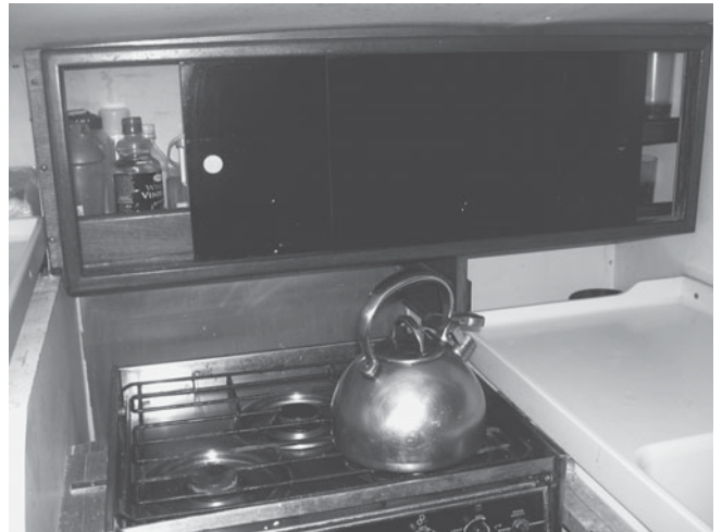
Figure 11-7. Horizontal sliding doors and a large fiddle offer the best solution for accessing galley lockers.
