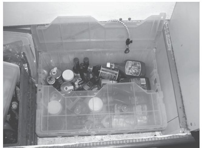
Figure 11-11. We stow glass containers and plastic containers with liquid contents in this heavy-duty plastic crate with a lid to contain the mess in the event of breakage. The crate is bolted to the bottom of the locker and the bungee cord would keep the lid on in a knockdown.
