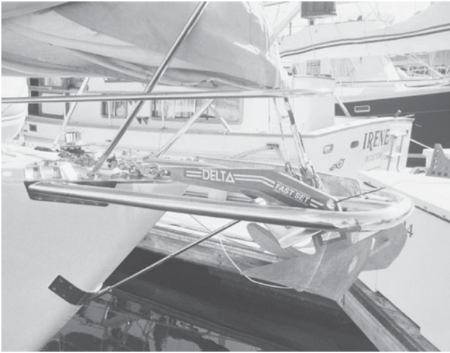
Figure 4-21. A solid stainless steel bow platform that could be fabricated for most offshore boats.
