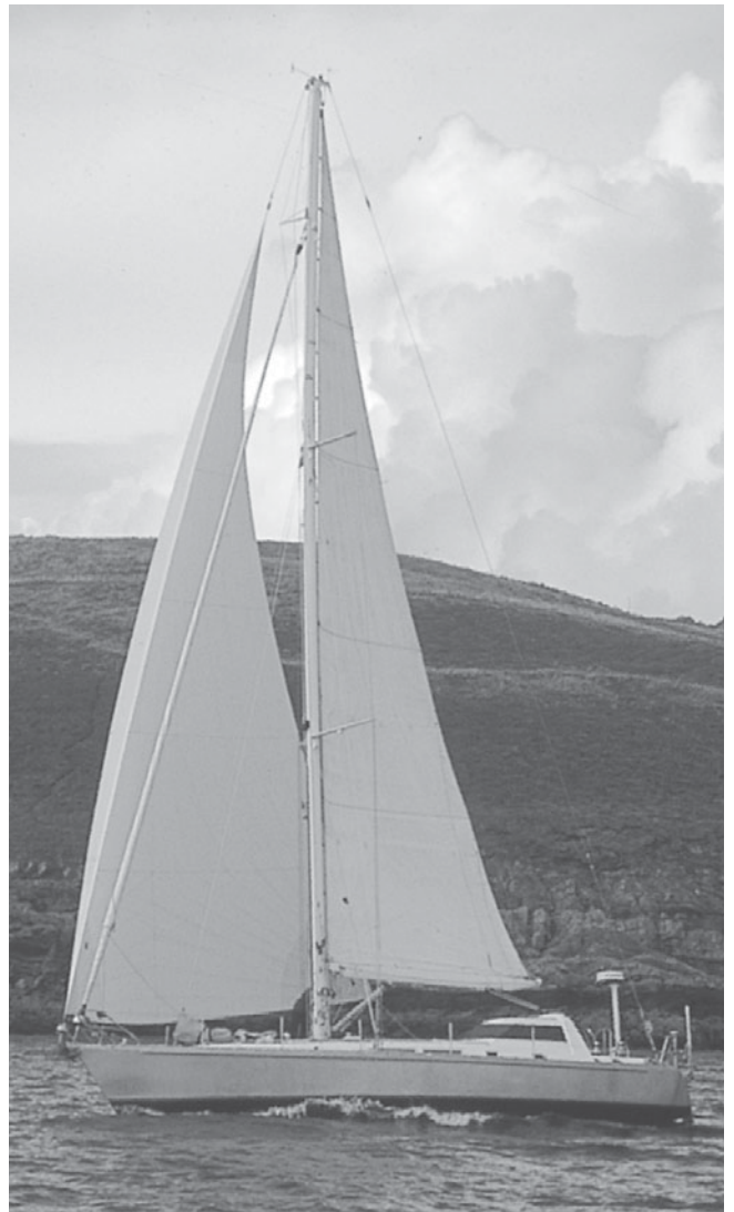
Figure 5-22. Evans is at the mast tensioning the halyard to tighten the luff as I unfurl the sail from the cockpit. (John Neal photo)
