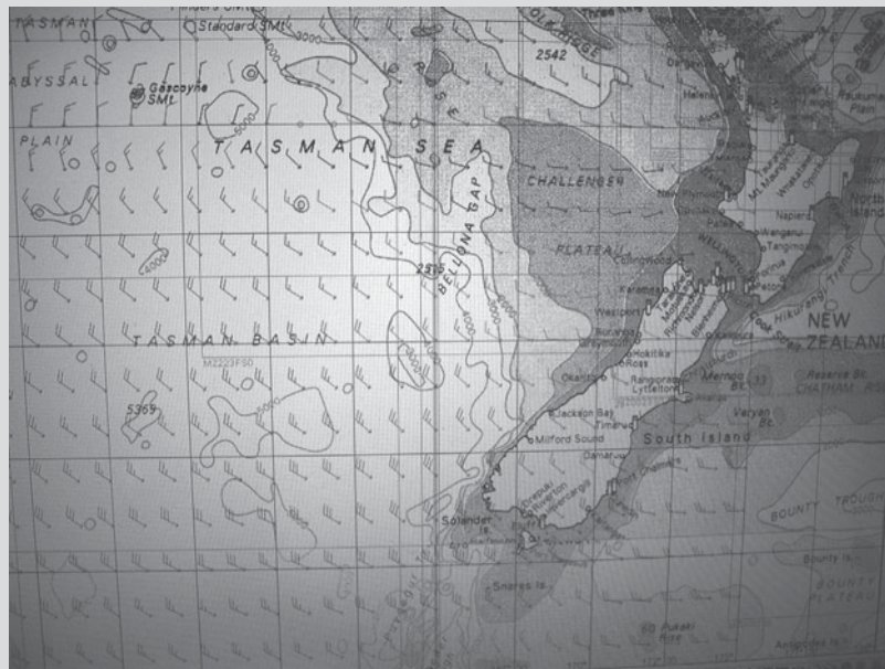
Figure 19-14. A wind speed and direction GRIB.
