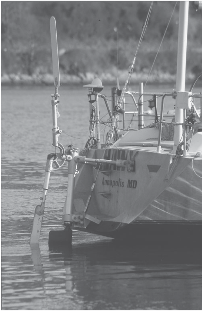
Figure 7-8. Hawk's Windpilot wind vane uses a servo-pendulum gear to drive an auxiliary rudder.
