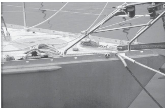
Figure 6-12. All our docklines are fitted with either fire hose or plastic water hose to prevent chafe.
