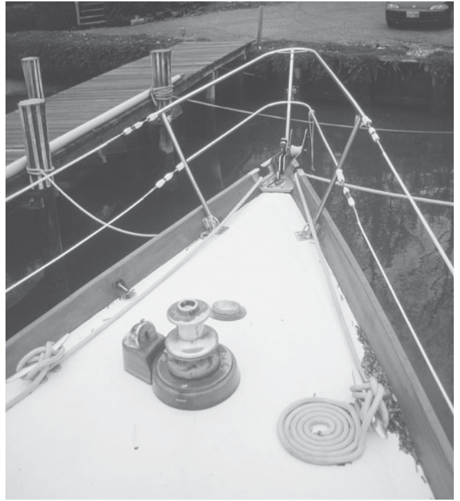
Figure 3-15. Anchoring platform on a Hood 50, a 50-foot fiberglass boat used for coastal sailing and racing.
