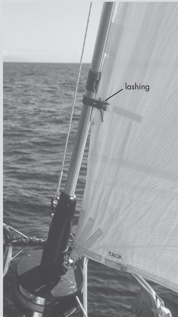
Figure 5-40. The lashing holds the tack of the jib to the roller furling foil and prevents chafe or wear at the tack.
