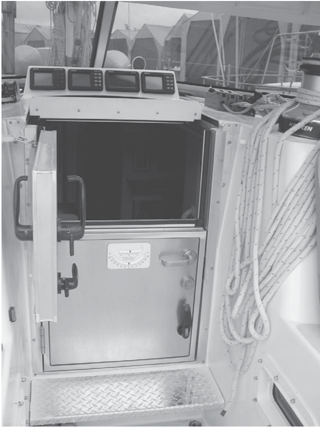
Figure 4-5. This aluminum Dutch door on Hawk bolted into the original frame for the hatchboards but was significantly stronger and more watertight.
