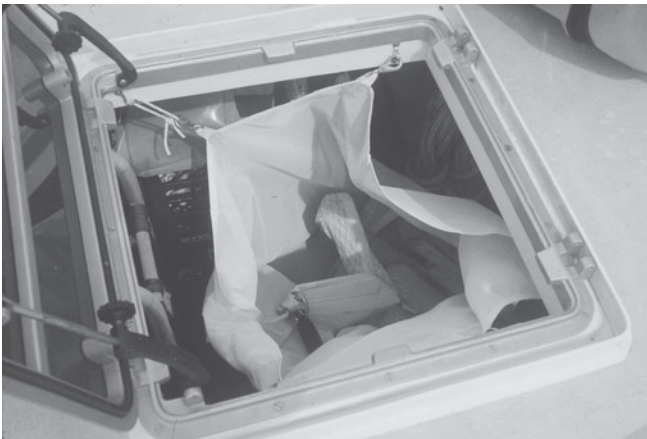
Figure 5-19. We stow the furled Code Zero in a mesh bag that clips to the sail locker hatch.
