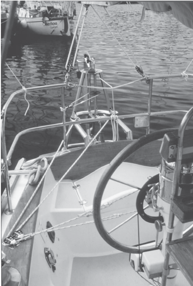
Figure 7-9. Silk's control lines ran through a single turning block between the wind vane and the wheel.
