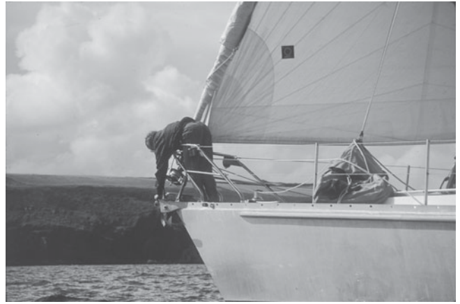
Figure 5-21. Evans attaches the furling unit to the bow roller using a low-stretch, high-strength Spectra pendant. (John Neal photo)
