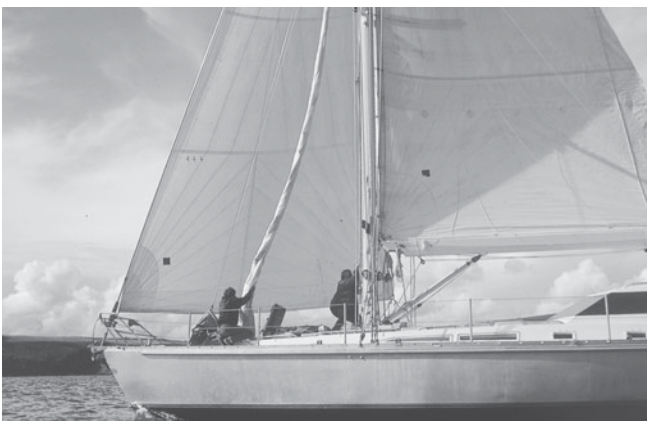
Figure 5-20. After attaching the halyard, I raise the sail out of the bag while Evans keeps it from getting caught on the rig. (John Neal photo)
