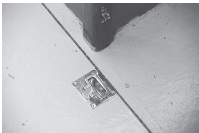
Figure 4-35. These stout ABI latches can be retrofitted to secure the floorboards on almost any boat.
