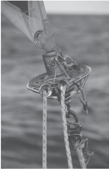
Figure 5-18. Our Facnor continuous-line Code Zero furler—a removable furler for handling large sails.
