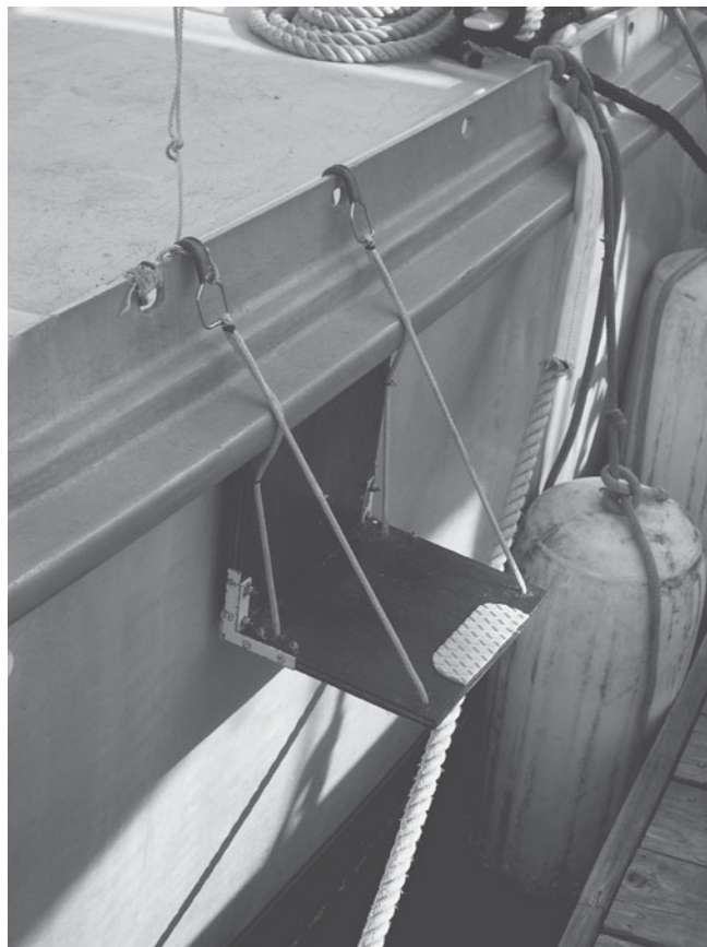
Figure 11-17. Our dinghy step makes it easy to get on and off the boat from a dinghy or floating pier.
