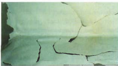
If holes or cracks are not welded properly this may cause problems with cleaning and pre-treatment. This in turn can cause small blisters, that cause de-tacking of the paint-layer.
