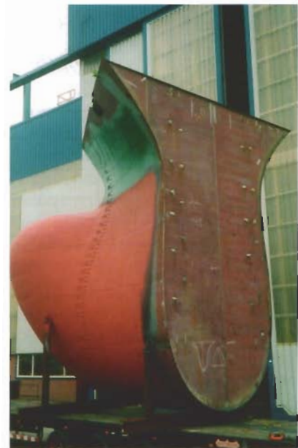
Forepeak, ready to be installed
