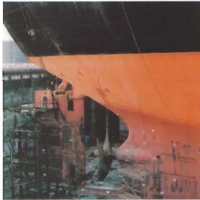
Removal of complete rudder, weight approximately 120 tons
