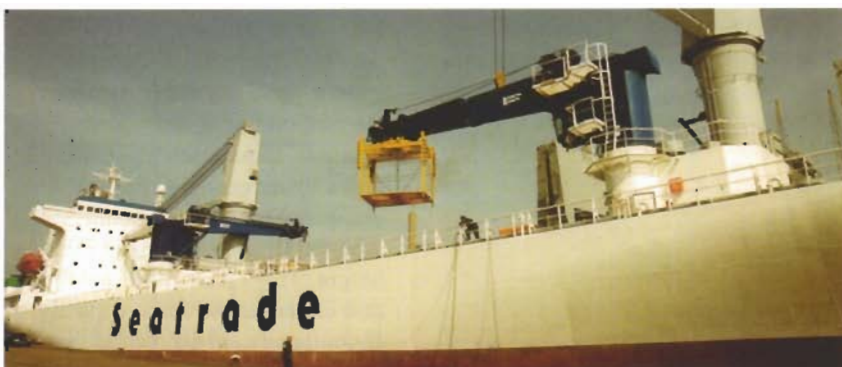
Reefer with pallet-swinger and conventional cranes
