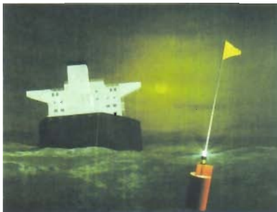
Buoy of an emergency towing system
