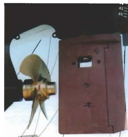
A controllable pitch propeller and a flap rudder of a multi-purpose vessel. The underside of the rudder stock can be seen in the rudder.
