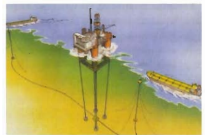
TLP on location connected to the oilwell(s), giving its oil to the temporarily moored shuttle tankers. Water depth 350 metres
