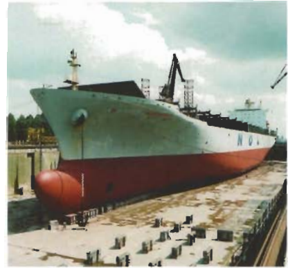
A ship with a small block-coefficient and a large midship section coefficient
