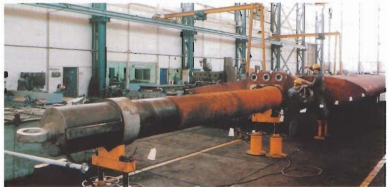
Alignment of rudder and stock in shop
