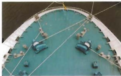
Winches on the forecastle and on the quarter deck of a car ferry
