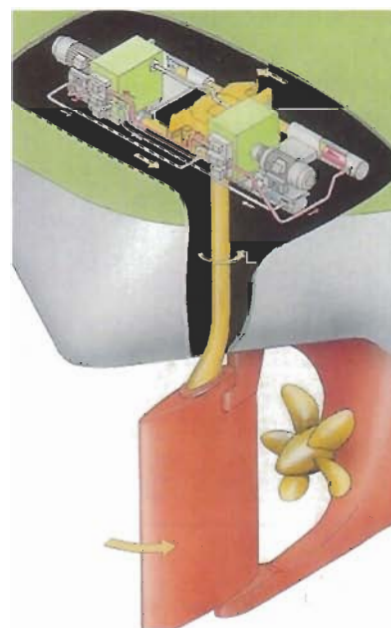
Ram steering engine on a large ship (turning the rudder to starboard)
