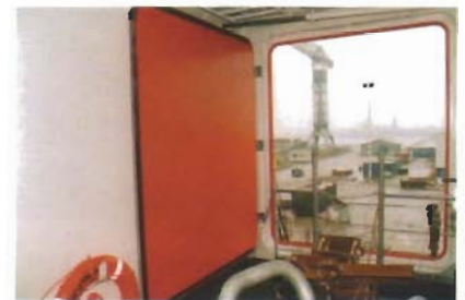
An opened side door, equipped with hydraulic cylinders for opening and closing. Also shown in the photo a lifebuoy and the pilot ladder.
