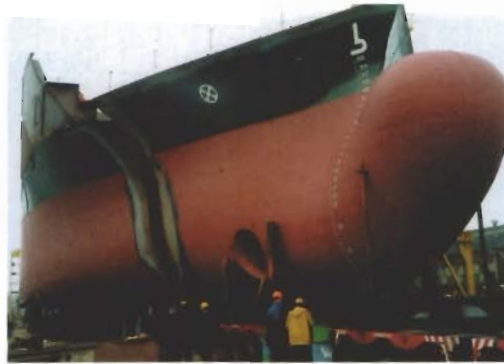
The fore part is being attached to the ship
