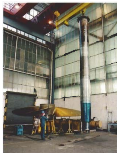
Preparing propeller and tailshaft for proper fit on conical part prior to installation on board
