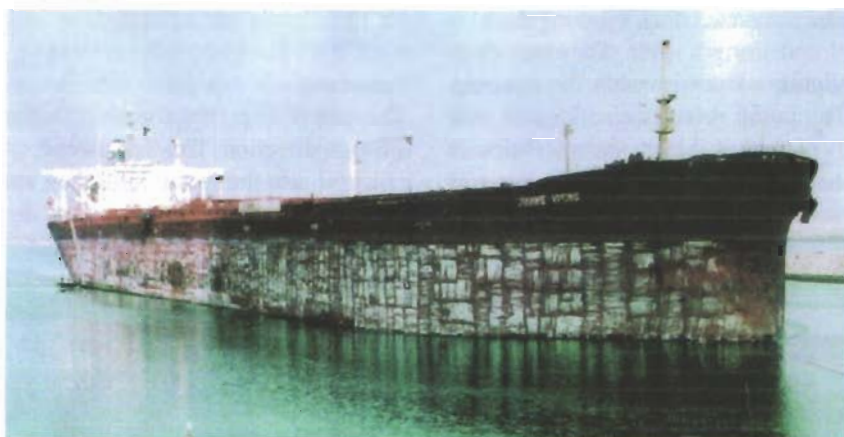
Antifouling at the end of its life and worn out. Time for repainting. The spraying pattern on the skin is still visible. The outermost layer of antifouling is still partly visible on the overlap. In between it has disappeared completely.
