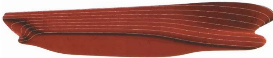
The submerged part of this ship clearly shows the difference in volume between the midships section and the aft ship. This explains the difference in upward pressure.
