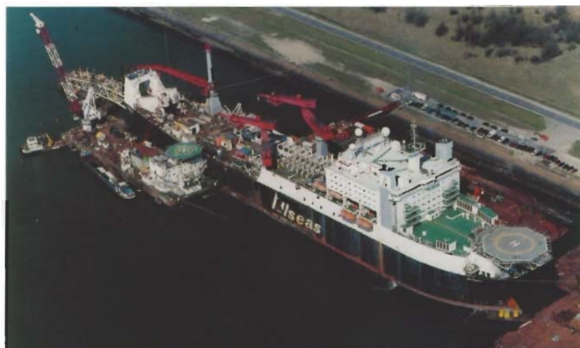
S-lay pipelaying vessel with crane barge alongside
