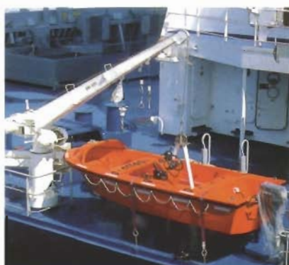
Permanent MOB -boat. If the boat is suspended from the crane, it can be lowered by pulling the triangle.
