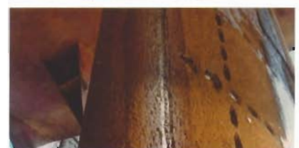
Cavitation damage on a rudder blade
