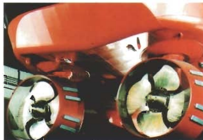
Two rudder propellers in a nozzle, with 360° rotation.
