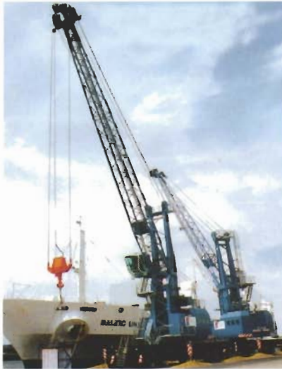
A mobile crane on pneumatic-tyres
