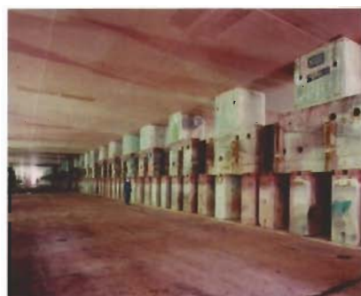
Ship supported by special dock block-arrangement with enlarged height (in a graving dock).
