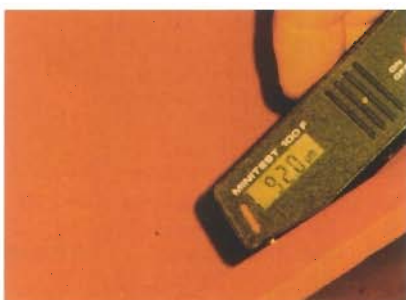
Ultra-sonic device to measure the thickness of the paint-layer
