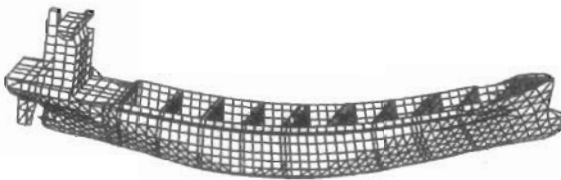
Ship on a wave top, hogging
