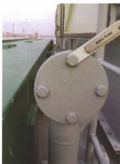
In port, oil and sludge are to be pumped ashore to a reception facility via the standard discharge connection.
