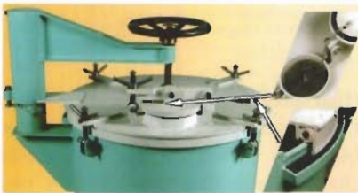
A rotating tank-lid on an expansion trunk
