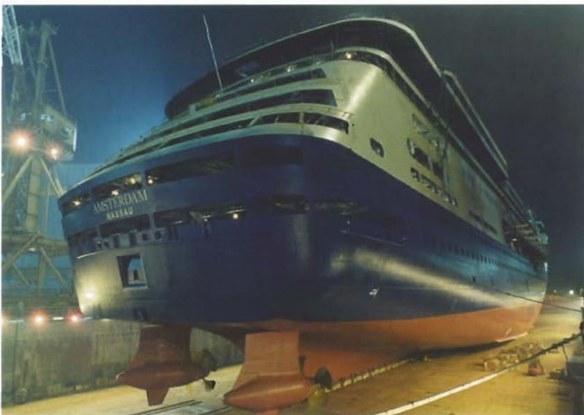
A cruise ship with 2 electrical rudder propellers that can rotate 360°.
