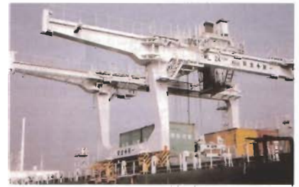
U-gantry with trolley on a container-ship
