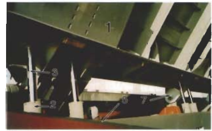
Partially opened hatch
