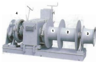
Anchor windlass with mooring gear and warping head
