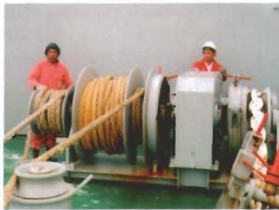
The main shaft is rotating, the warping end is the only part that is also rotating. The gypsy wheel and both drums are disconnected.
