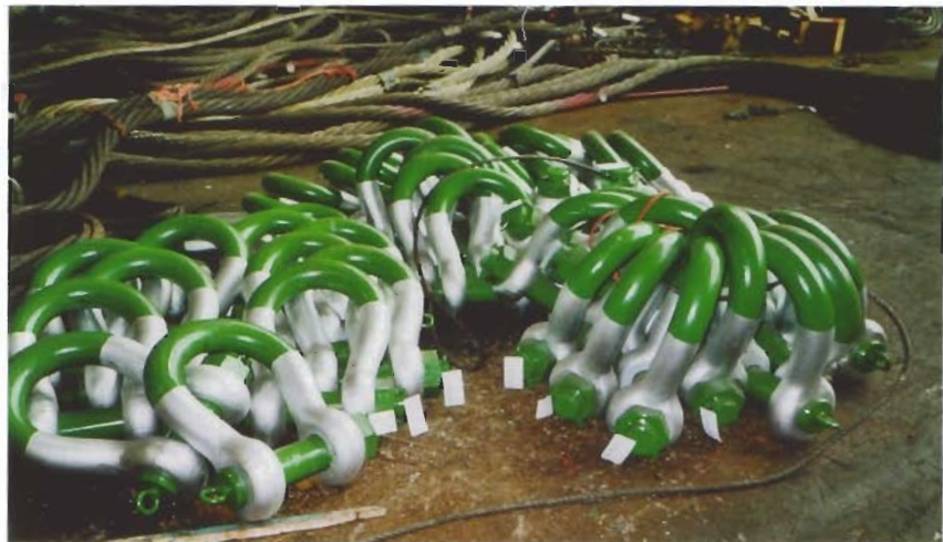
Heavy-duty bow shackles ready for testing
