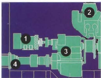
Various methods of driving a shaft generator, the "power take off" or PTO
