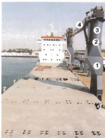
Feeder with deck cranes
