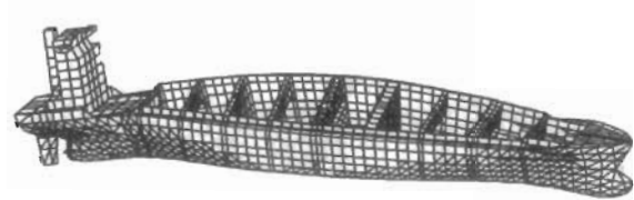
Waves coming in from starboard at an angle, torsion
