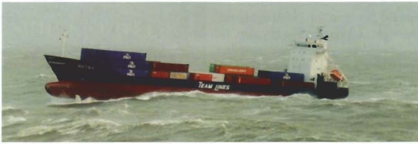
Container feeder in heavy weather. The ship is partially on a wavetop; hogging
