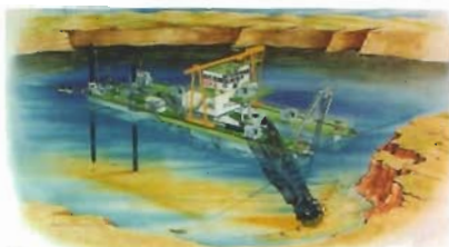
Cutter suction dredger, moving around a spud pole
