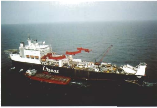
S-lay pipelaying vessel on DP with pipe supplier alongside
