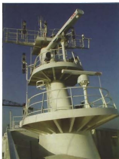
Top deck of a modern ship showing the compromise in installation of a transmitting disturbing radar aerial and the VHF receiver aerials.
