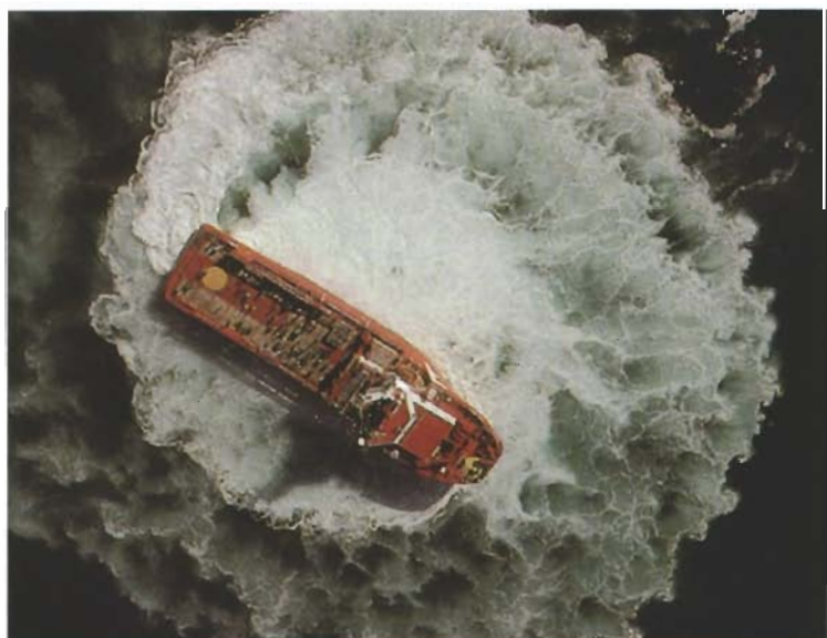
Aerial photograph of a supplier shows the optimal manoeuvring capabilities of a rudder propeller in combination with a bow thruster
