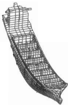
Ship in a trough, sagging
