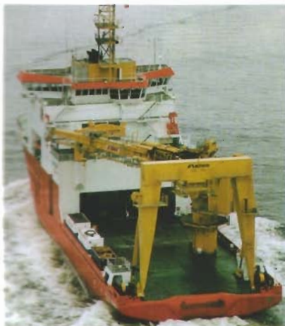
A multipurpose support vessel (with heavy crane and A-frame) for the offshore industry.
