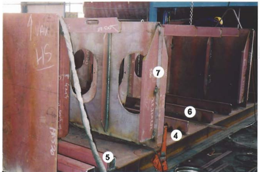
Double bottom of a container feeder
