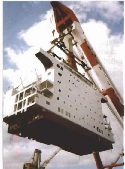
Installation of a complete deckhouse, while the ship is at the fitting out dock.
