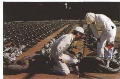
Surveyors check links and shackles of an anchor chain.
