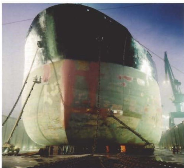
Anchors and chaincables are lowered. Blasting and painting is in progress..
