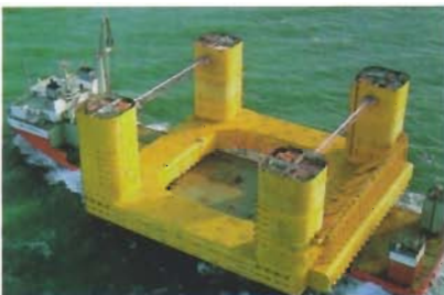
Semi-submersible ship with the lower hull of a floating production unit (semi-sub).
