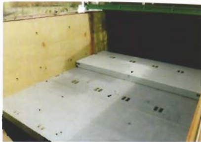
Horizontally placed pontoons as tween deck
