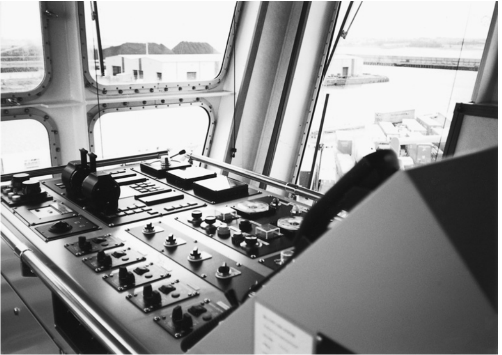
Remote controlling station. An enclosed bridge wing control station having dual controls for CPPs, bow thrust and numerous indicators for displaying operational data.
