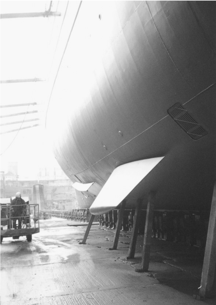
Fixed stabilizer fins. Non-retractable trapezoidal stabilizer fin seen exposed from the hull of a vessel in dry dock. The angle of the fin can be changed by use of hydraulic cylinder action or by a rotary vane motor.
