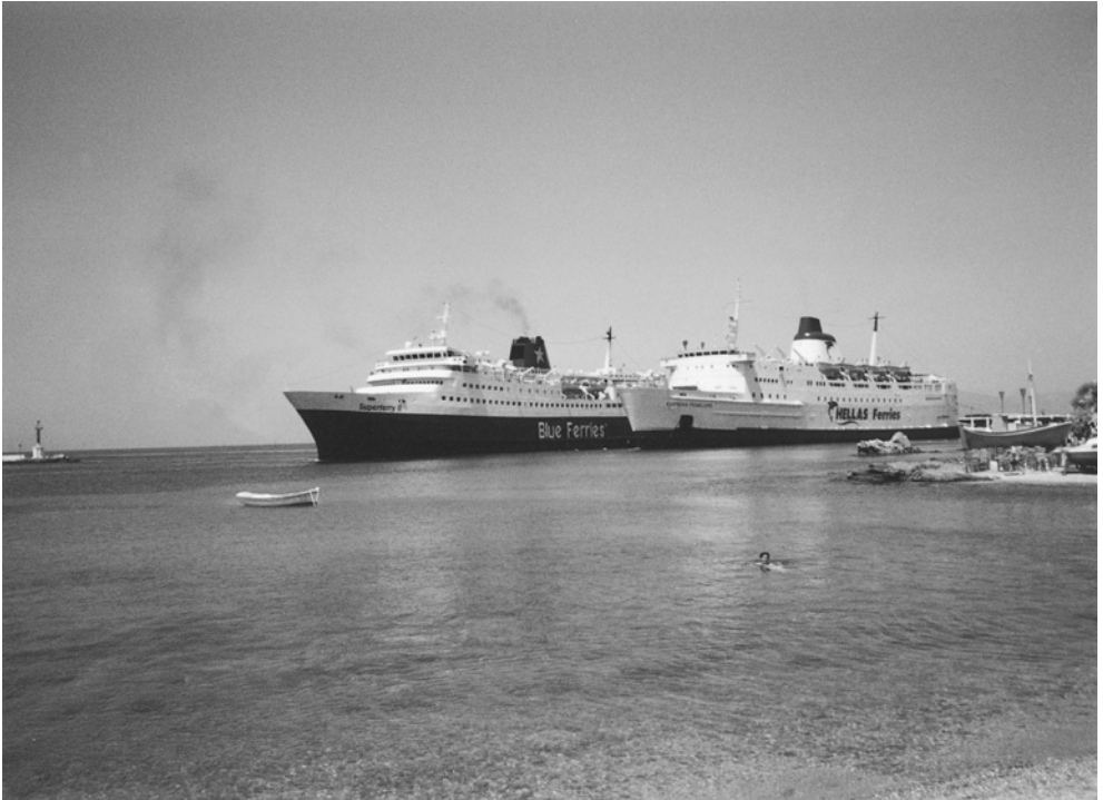
The 'Superfast II', passenger/vehicle ferry manoeuvres to establish into a Mediterranean Moor alongside the passenger/vehicle ferry 'Express Penelope'. Both vessels will be secured by stern moorings with both anchors released at short stay.
