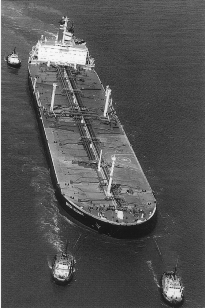
The BP Tanker British Reliance assisted by four tugs. Two bow tugs are engaged in pulling, while two other stern tugs are just visible operating off the port and starboard quarters.
