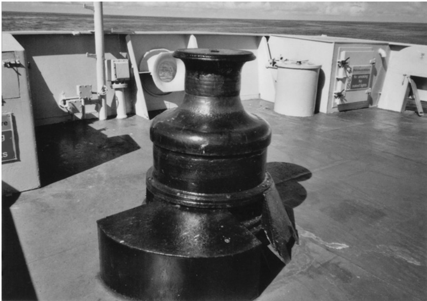
Mooring equipment: Types of roller leads. Pedestal roller fairlead welded to aft mooring deck. Colloquially referred to as an 'old man'.
