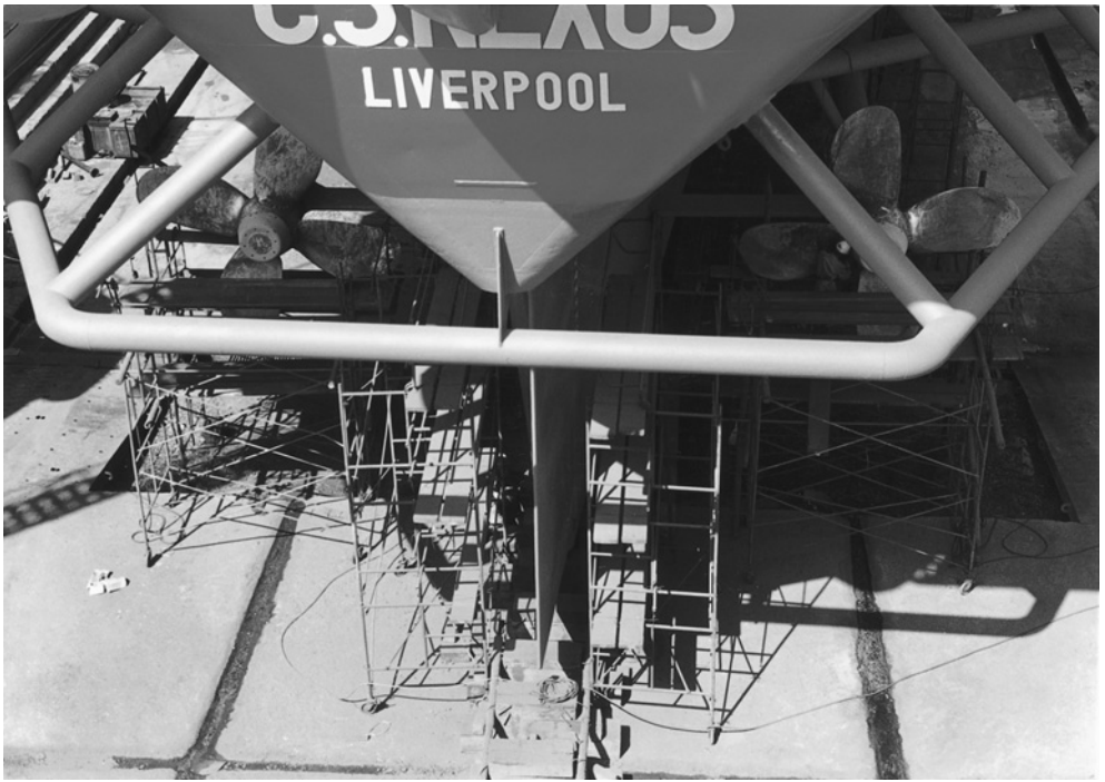
Twin, four-bladed, fixed pitch propellers, positioned either side of a single balanced rudder. The arrangement seen fitted to the cable ship 'Nexus' exposed in dry dock.
