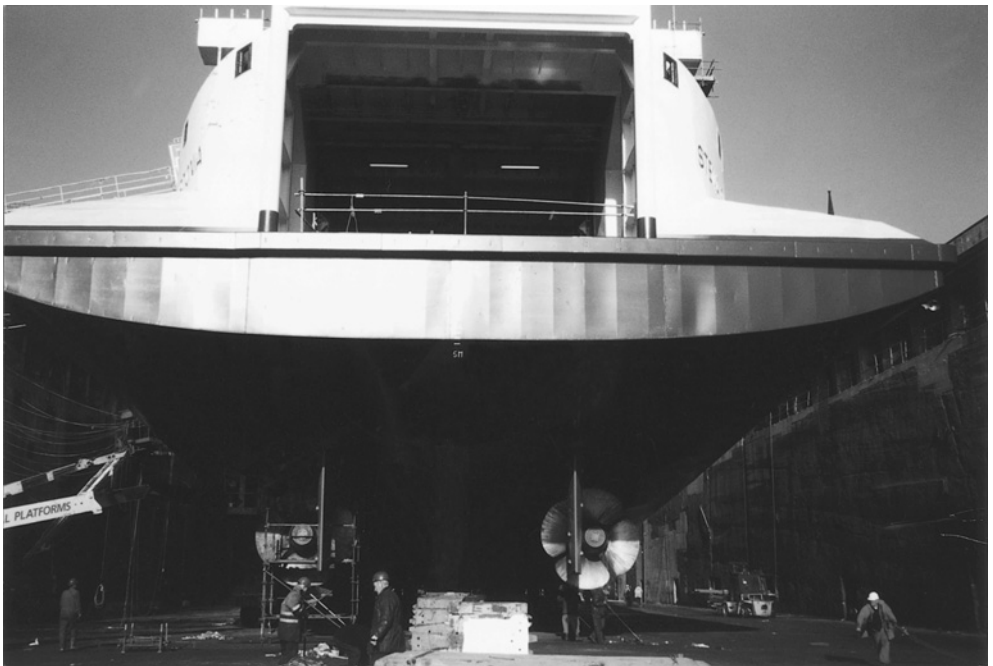
Twin multi-blade propellers fitted in association with twin rudders aboard a vehicle ferry, seen exposed in dry dock.
