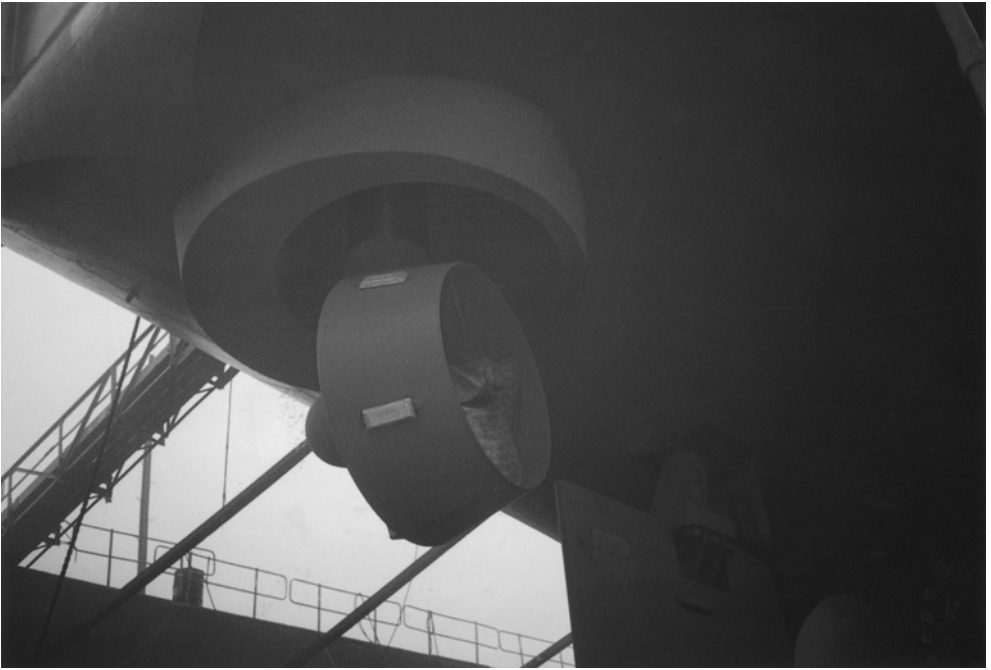
A ducted azipod, featured on the outer hull port side, of a twin rudder/twin propeller vessel.
