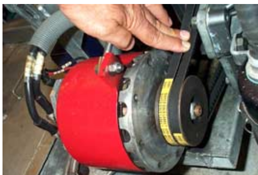
A common area for problems is the shaft coupling or flexible joint (above) between transmission and prop shaft. We check the bolts before every long passage and at least once every 100 engine hours. If a flex coupling is used watch for signs of fatigue (cracking is common). Alternator belt tension and brackets are checked every 100 hours, too.
