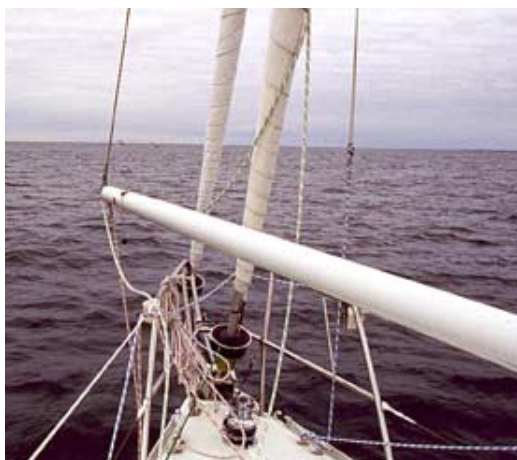
Fernando Goes sets the carbon fiber spinnaker pole on a Sundeer 60 during sea trials. If conditions were rougher there would be someone guiding the outboard end.
