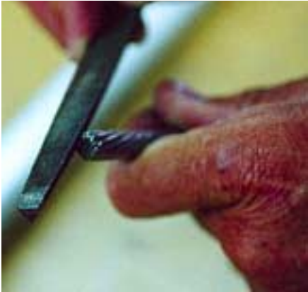
Step one is to file the edges of the wire so there are no sharp burrs. This allows them to slide into position more easily inside the body of the terminal.
