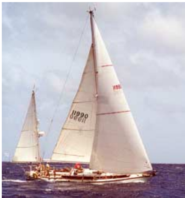
Reaching along in fresh tradewinds this yawl has taken a quick tuck in the mainsail. While changing headsails is always a pain, she would be more efficient if she were flying a smaller, higher clewed jib and full main on this range of sail.
