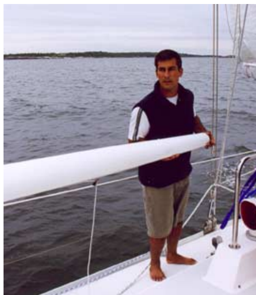
Fernando Goes sets the carbon fiber spinnaker pole on a Sundeer 60 during sea trials. If conditions were rougher there would be someone guiding the outboard end.
