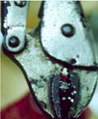
After sliding the female portion of the terminal down the wire the next step is to unlay the wire so that the outer strands are splayed out from the core. A vise grip works well for this process.
