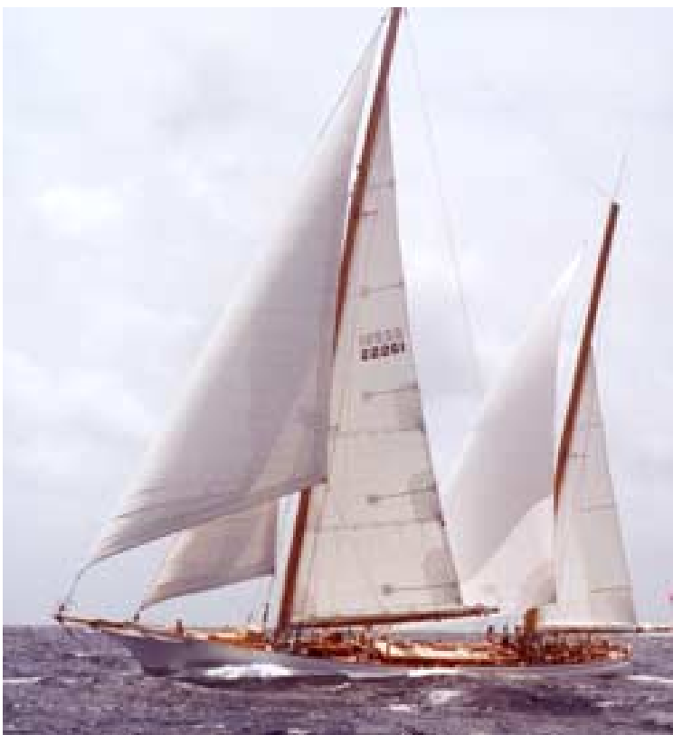
White Hawk set up for power reaching in just a hair too much wind. She's got reefs in the main and mizzen, but is carrying her mizzen jib. The very high clew on the yankee jib makes the slot between it and the staysail more efficient. But that staysail would work even better if its clew were lower.
