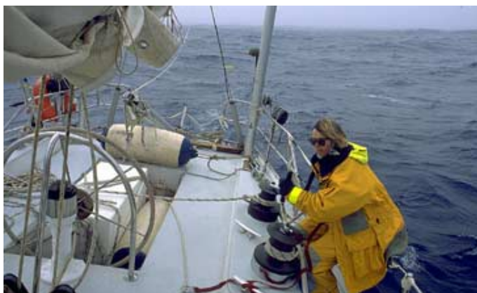
Sweep control lines were lead to a pair of cockpit winches (below). With a somewhat smaller sweep one could accomplish a similar amount of control using five- or six-to-one-tackles.
