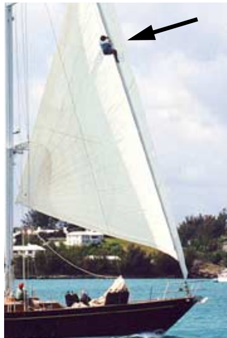
If working on the headstay is required, typically on the furler joints, the same lazy halyard approach can be used to provide some security. In this case the halyard is secured just forward of the headstay, and then winched very tight. A short strap from the top of the chair is attached to hold the person aloft from swinging back to the mast.
