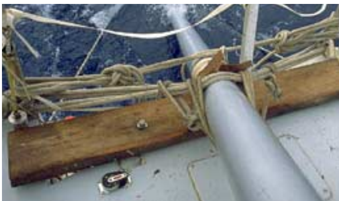
A detail shot (above) of the lashings used to hold the sweep in place. Note lashings over the athwartships lines and then under the pole, and then back again. The fender (below) is used to keep the sweep from dropping too low.
