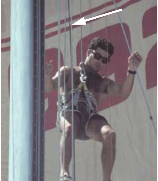
A climbing harness (above) is more secure than a chair. Note the tensioned halyard (white arrow) which makes a great handhold. At sea, we typically clip onto the tensioned halyard, using it like a jackstay, to prevent swinging away from the boat as we roll in the seas.
