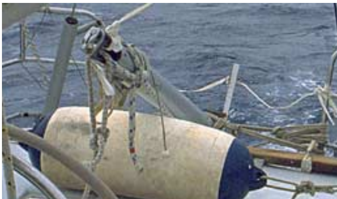
Sweep control lines were lead to a pair of cockpit winches (below). With a somewhat smaller sweep one could accomplish a similar amount of control using five- or six-to-one-tackles.
