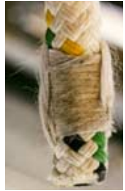
Having a deck knife ready to use in the cockpit and at the mast is handy, and in an emergency can be a tremendous asset (upper left). A sewn whipping is neater and lasts longer than tape or burning the ends of running rigging (upper right).
