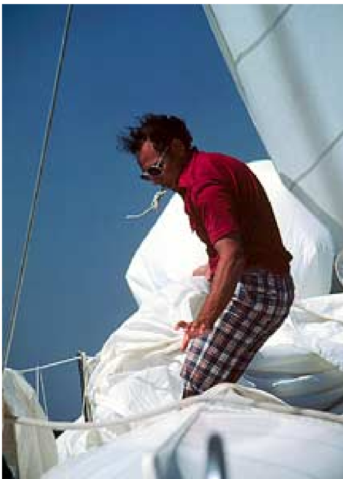
When you are working with sails, always position yourself inboard of the sail (as shown below). This way if a puff or wave catches the sail it doesn't take you over the side with it. (And unlike what is shown always wear a harness.)
