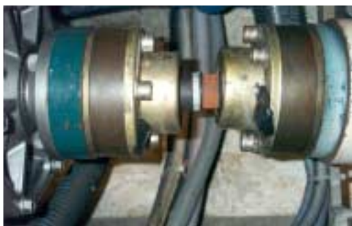
A common area for problems is the shaft coupling or flexible joint (above) between transmission and prop shaft. We check the bolts before every long passage and at least once every 100 engine hours. If a flex coupling is used watch for signs of fatigue (cracking is common). Alternator belt tension and brackets are checked every 100 hours, too.
