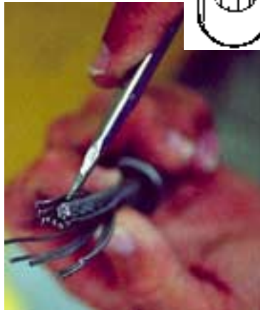
A screwdriver is used to open and direct the wires into an even pattern. This will take awhile, and with some wire is difficult due to construction. Take your time and get it right.
