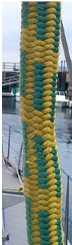
This series of four photos will give you an idea of a way to clean up chafe problems and prolong the life of sheets and halyards. In the left photo we see a heavily chafed halyard. We've stripped the cover off a piece of 1/2-inch (12.6 millimeter) polyester line and slipped it over the end of damaged halyard. The next image shows the cover worked over the chafed area. The narrow spot indicates the chafed section. The third photo (above) shows the end of the cover which has been seized (we taper the ends of the cover to make this neater). We usually make the cover a couple of feet (0.6 meters) long and then do a bit of hand sewing through it to help it carry the load.
